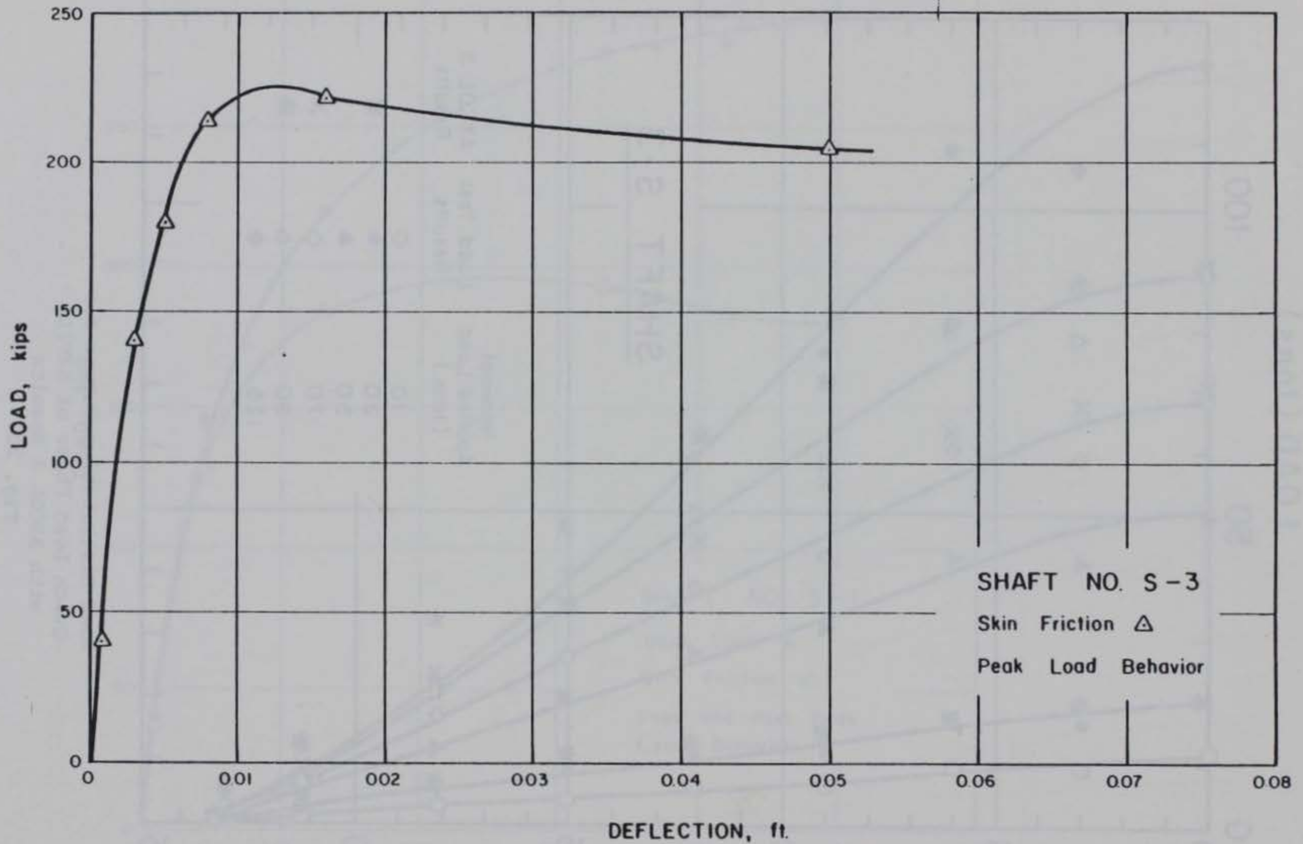
AXCOL Analyses for S-3 (Peak Load Behavior) FIG. 21(a)
