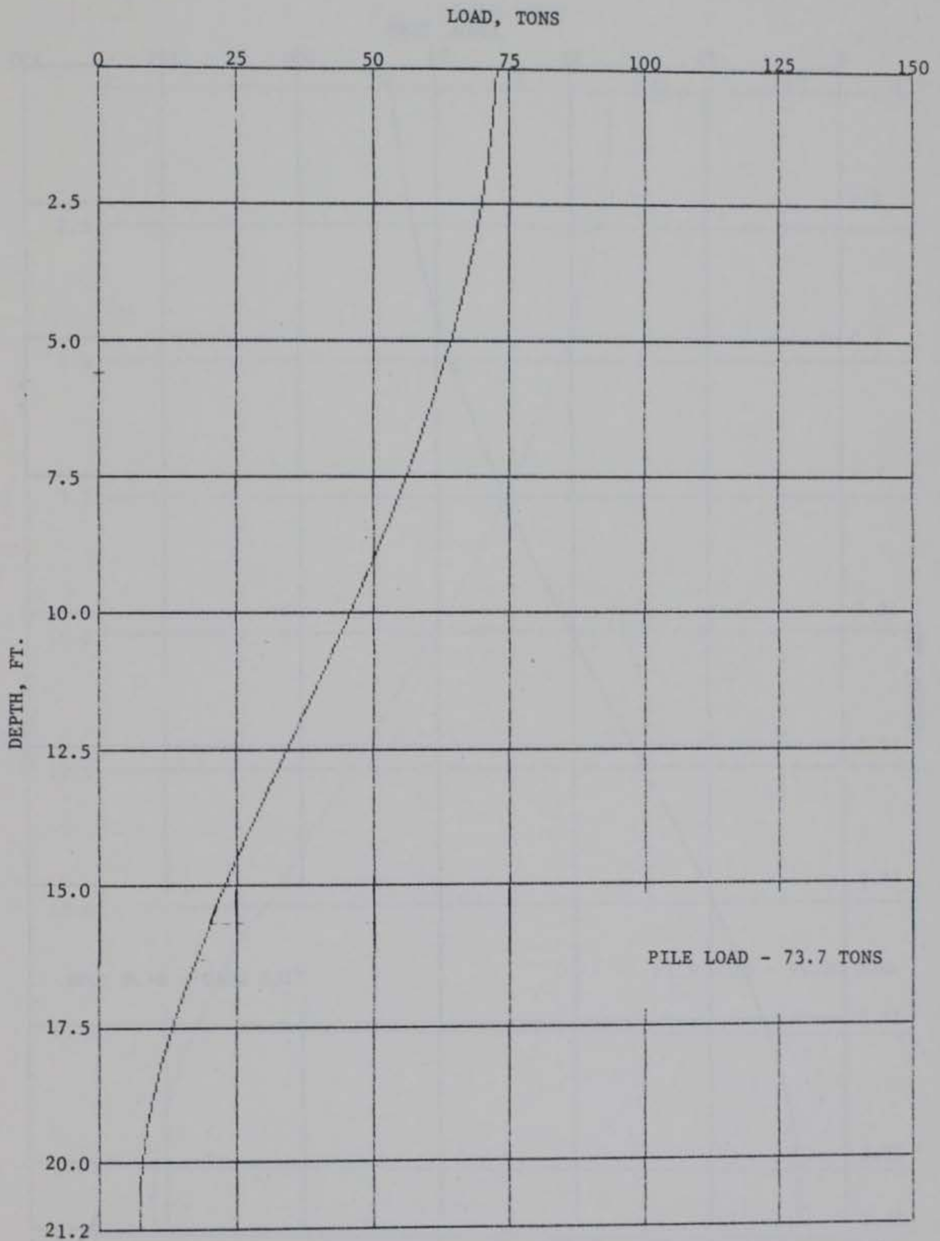
Fig. B-11 LOAD DISTRIBUTION CURVE SHAFT TEST - S1T1
