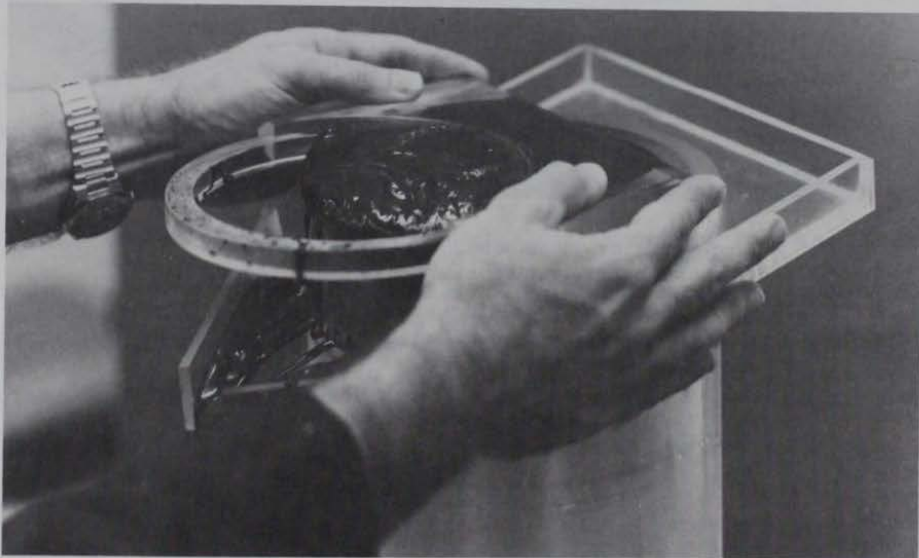
b. Inner ring is removed allowing the removed material to spill into a collection container
