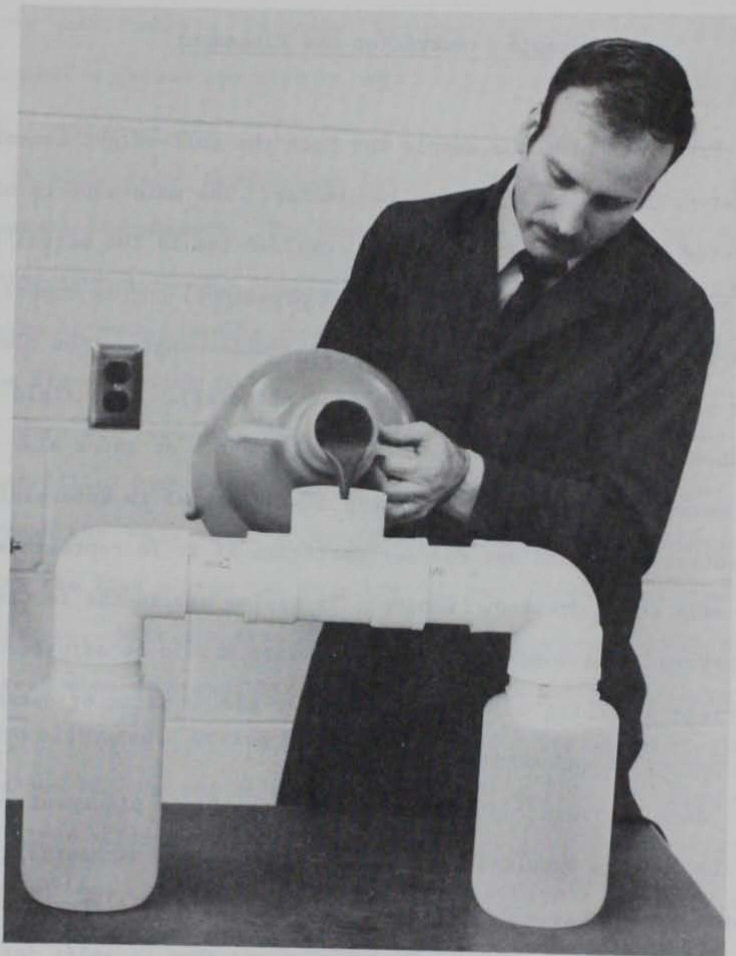
Figure 25. Method for splitting a slurry sample
