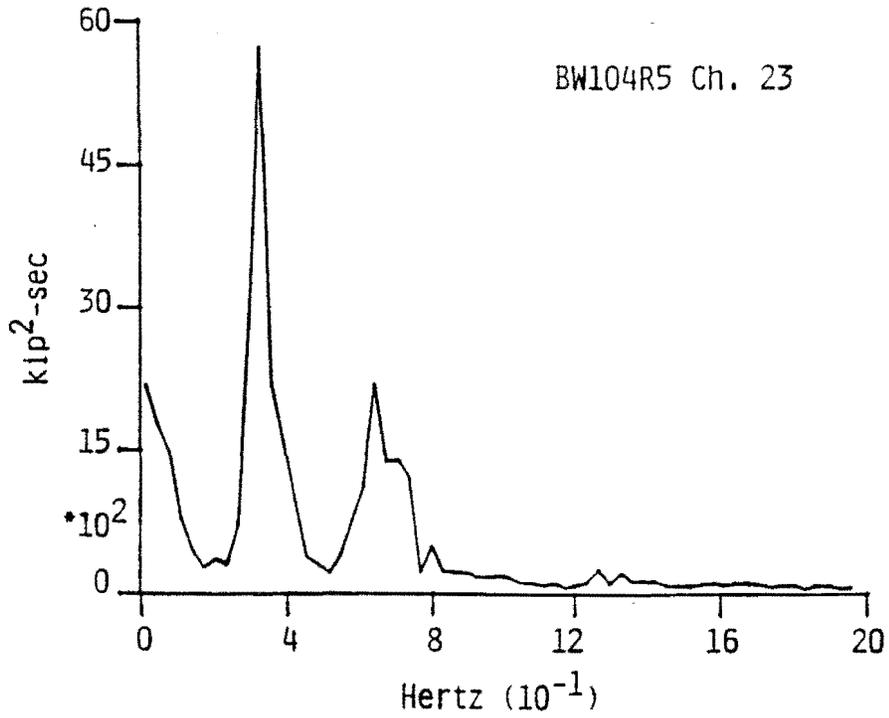
Figure 15. Resultant surge force between breakwater modules
