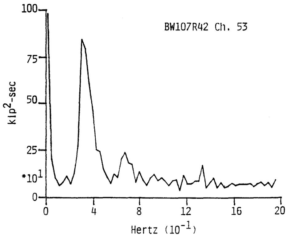
Figure 22. Sway shear force in west pontoon
