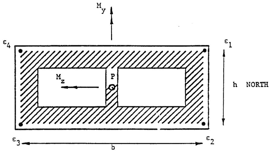
Figure 17. Typical breakwater cross-sections with longitudinal gages
