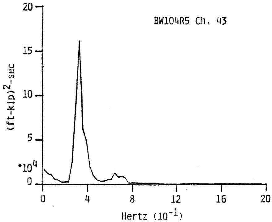
Figure 16. Resultant yaw moment between breakwater modules
