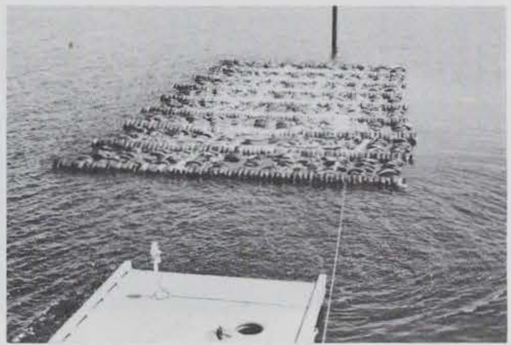
Photo B-22. Pipe-tire breakwater in position at the West Point test site.
