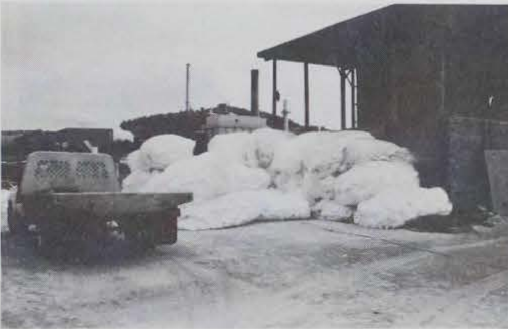
Photo A-15. Photo showing 600 cu ft of styrofoam that was "mined" from the end compartments of each float.
