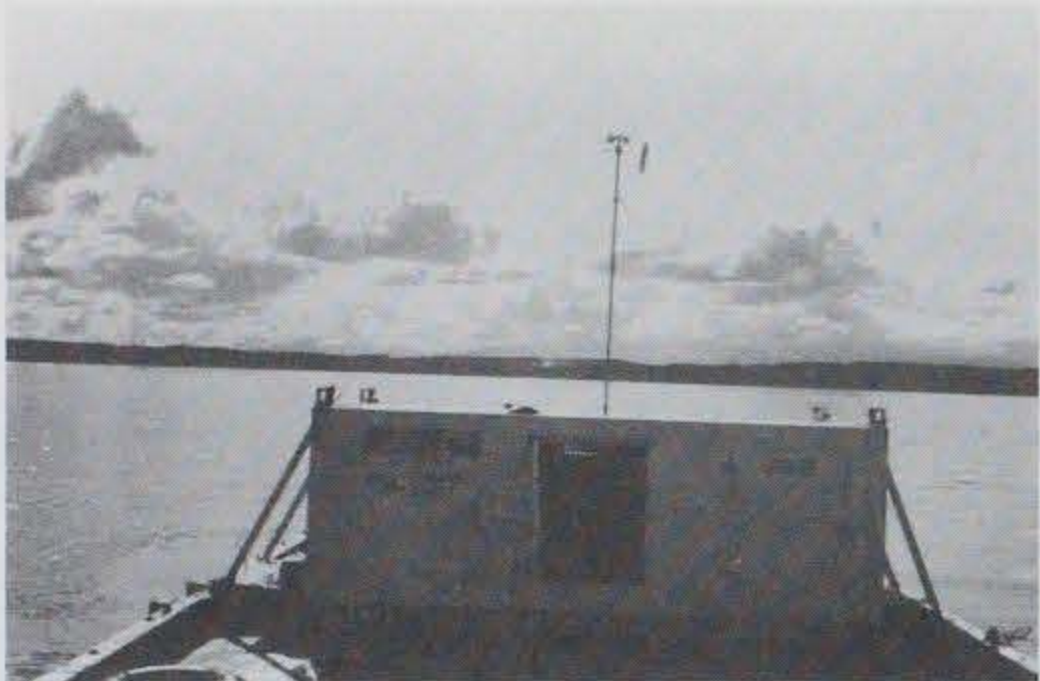
Photo F-21. Photo depicting deckhouse which greatly improved working conditions.
