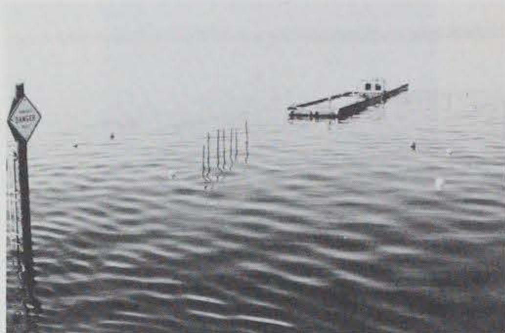
Photo F-22. Photo showing the wave array anchored in the vacant pipe-tire breakwater location.
