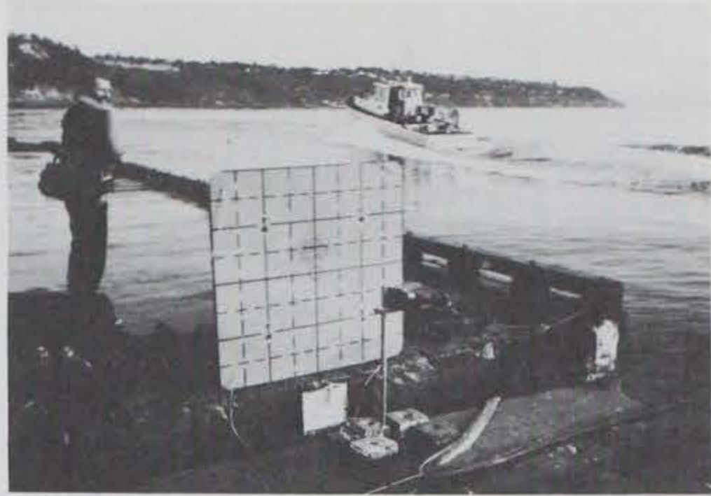
Photo E-2. A movie camera and target being used to record relative heave and sway motions.
