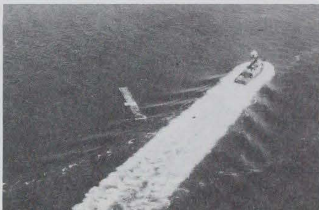
Photo E-10. Tug generating wake with crest perpendicular to breakwater.
