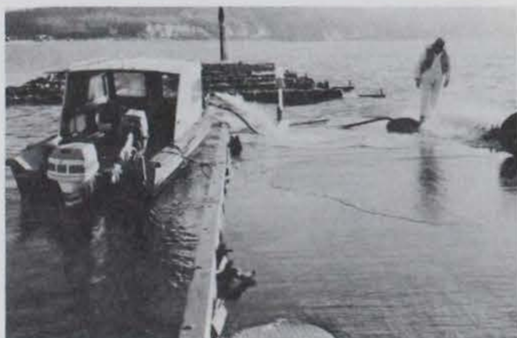
Photo A-23. Pumping out another end compartment (the deck is nearly awash).
