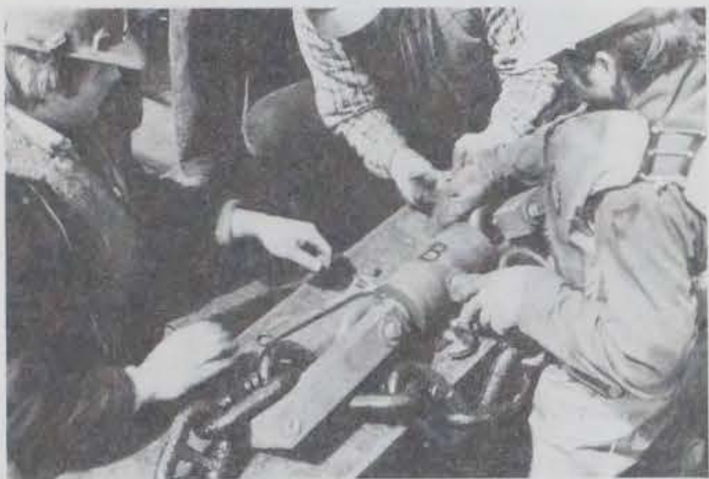
Photo F-3. Attaching anchor force load cell to anchor line.
