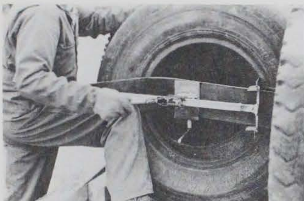
Photo B-9. A device, fashioned from an auto jack, being used to tighten belting.
