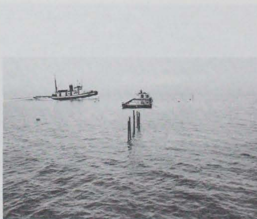
Photo E-12. 73-ft tug generating wake for test No. 4.
