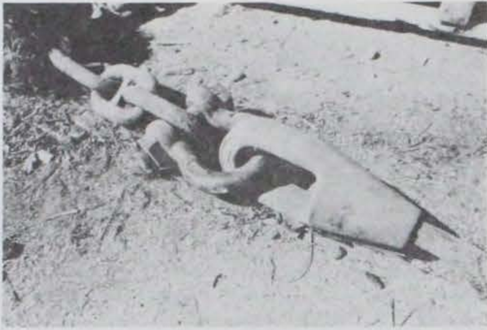
Photo C-19. Photo depicting good condition of anchor line hardware at test completion.
