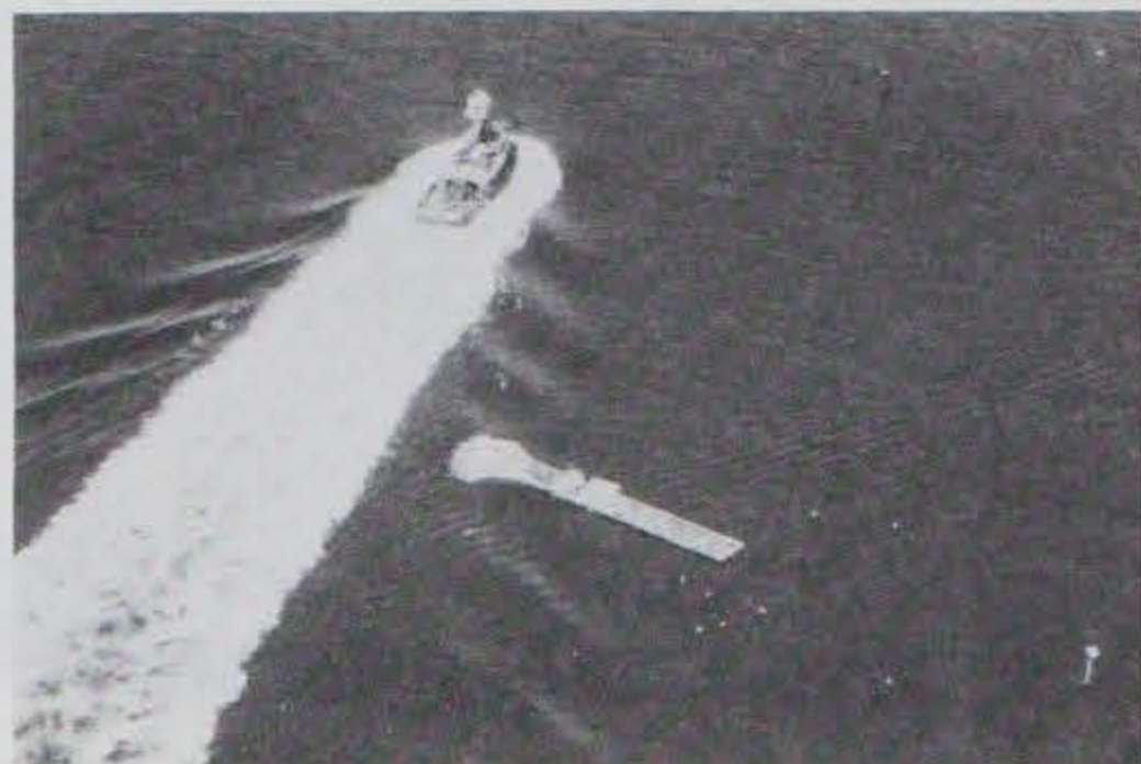
Photo E-8. Tug generating wake with crest nearly parallel to breakwater.
