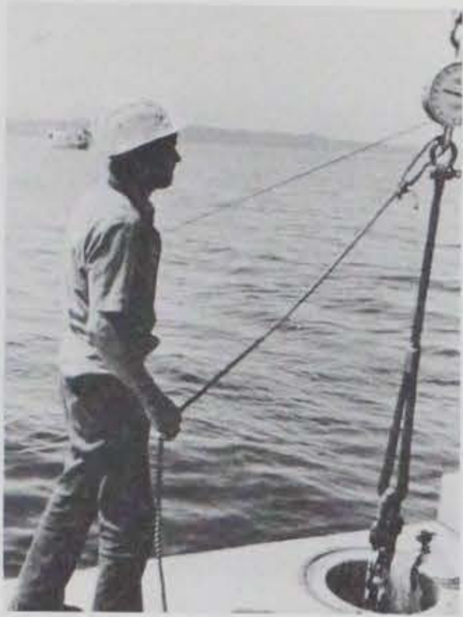
Photo C-13. Monitoring anchor line tension.
