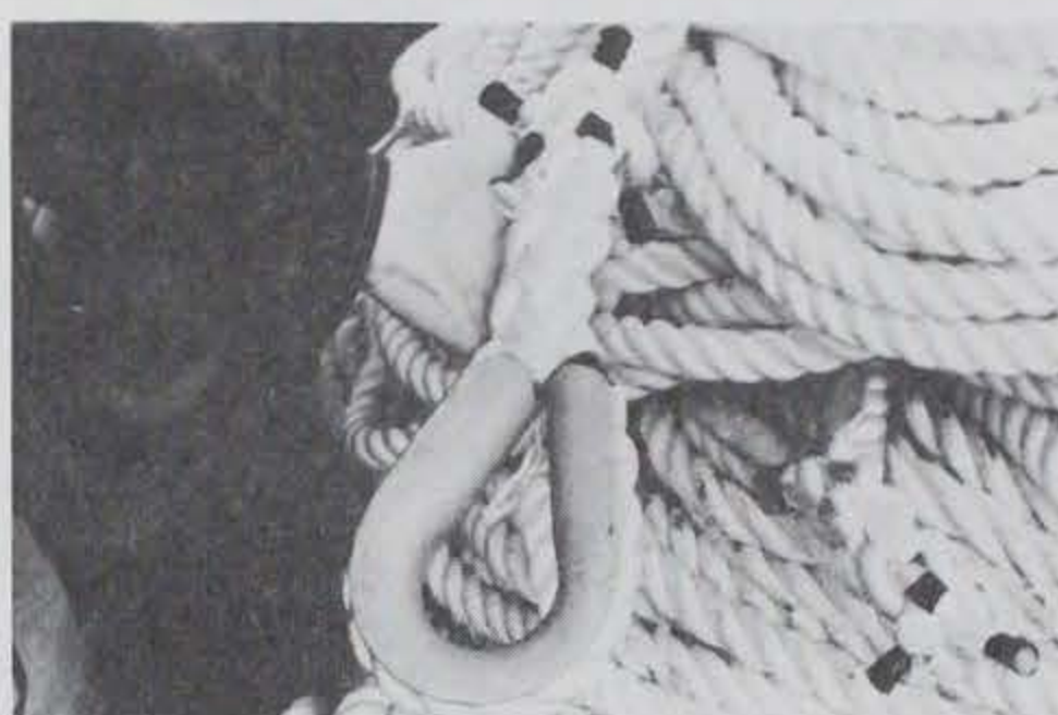
Photo C-4. Photo showing eye of splice and thimble in pipe-tire breakwater anchor line.
