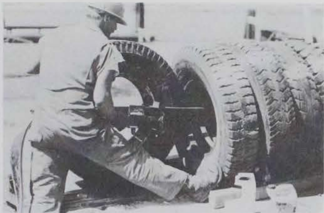
Photo 9. Tensioning of belting using a modified car jack.
