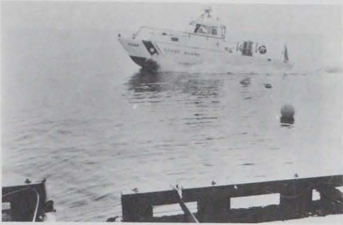
Photo E-1. 41-ft Coast Guard cutter being used in boat wake tests Nos. 1 and 2.
