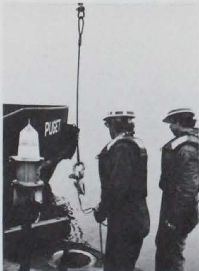
Photo C-35. Anchor line falling away after tripping release hook.
