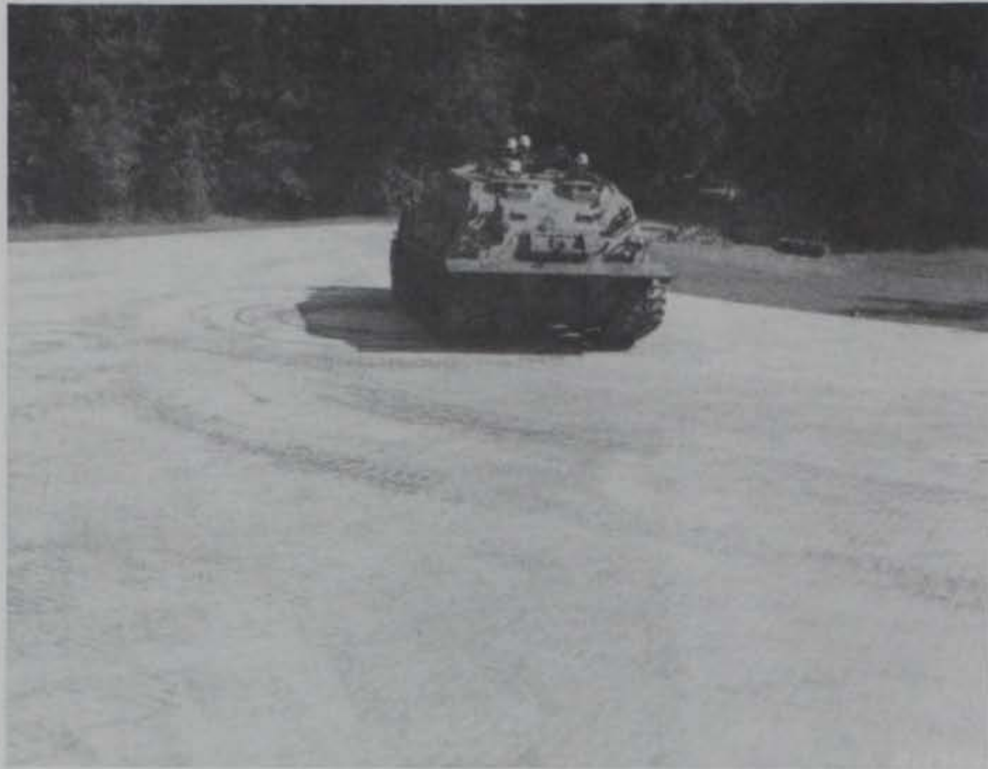
Figure 25. M-88 Tank Retriever performing 360-degree locked wheel turns
