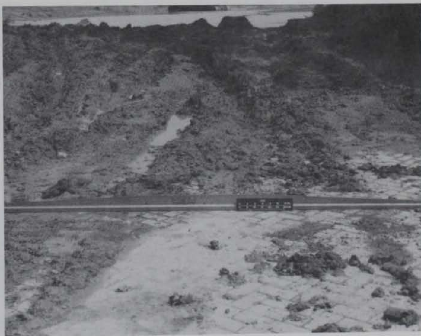
Figure 28. Straightedge measurements to check for pavement rutting (Note mud and water covered training area in background)
