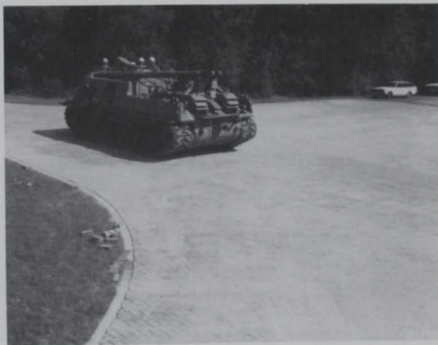
Figure 24. Initial traffic testing with M-88 Tank Retriever
