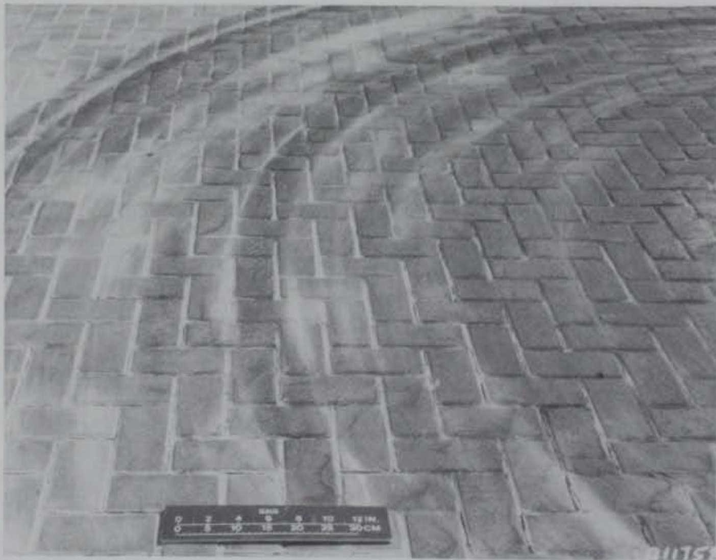
Figure 26. Rubber track marks left on top of undamaged paving block surface
