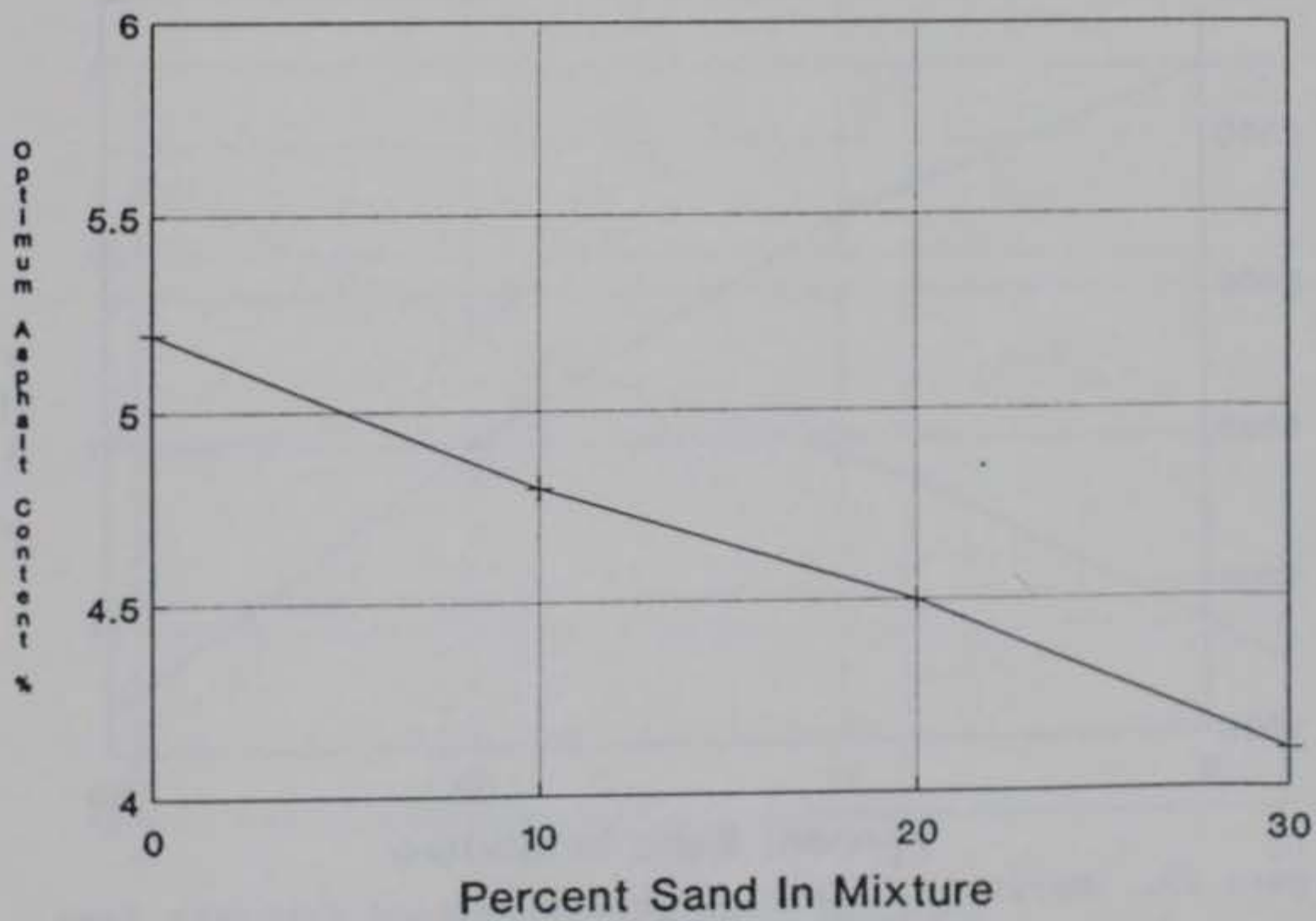
Figure 33. Optimum Asphalt Content Versus Percent Concrete Sand
