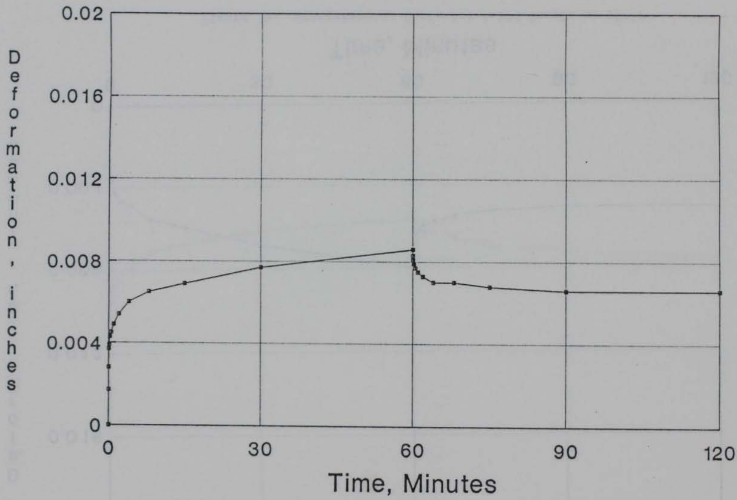
Figure 77. Creep-Rebound Curve for S-1C4 Sample at 104°F
