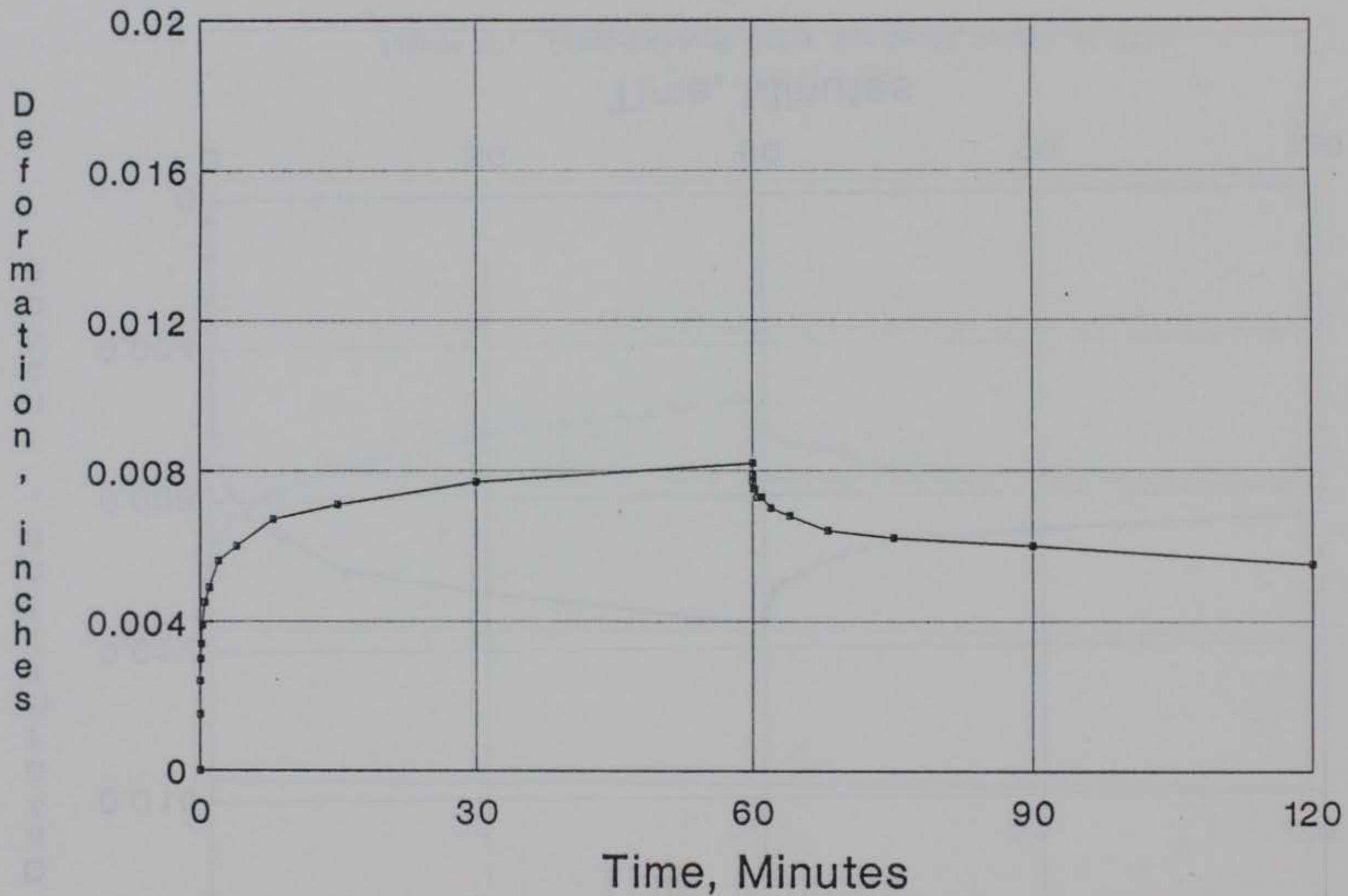
Figure 81. Creep-Rebound Curve for S-2C3 Sample at 77°F
