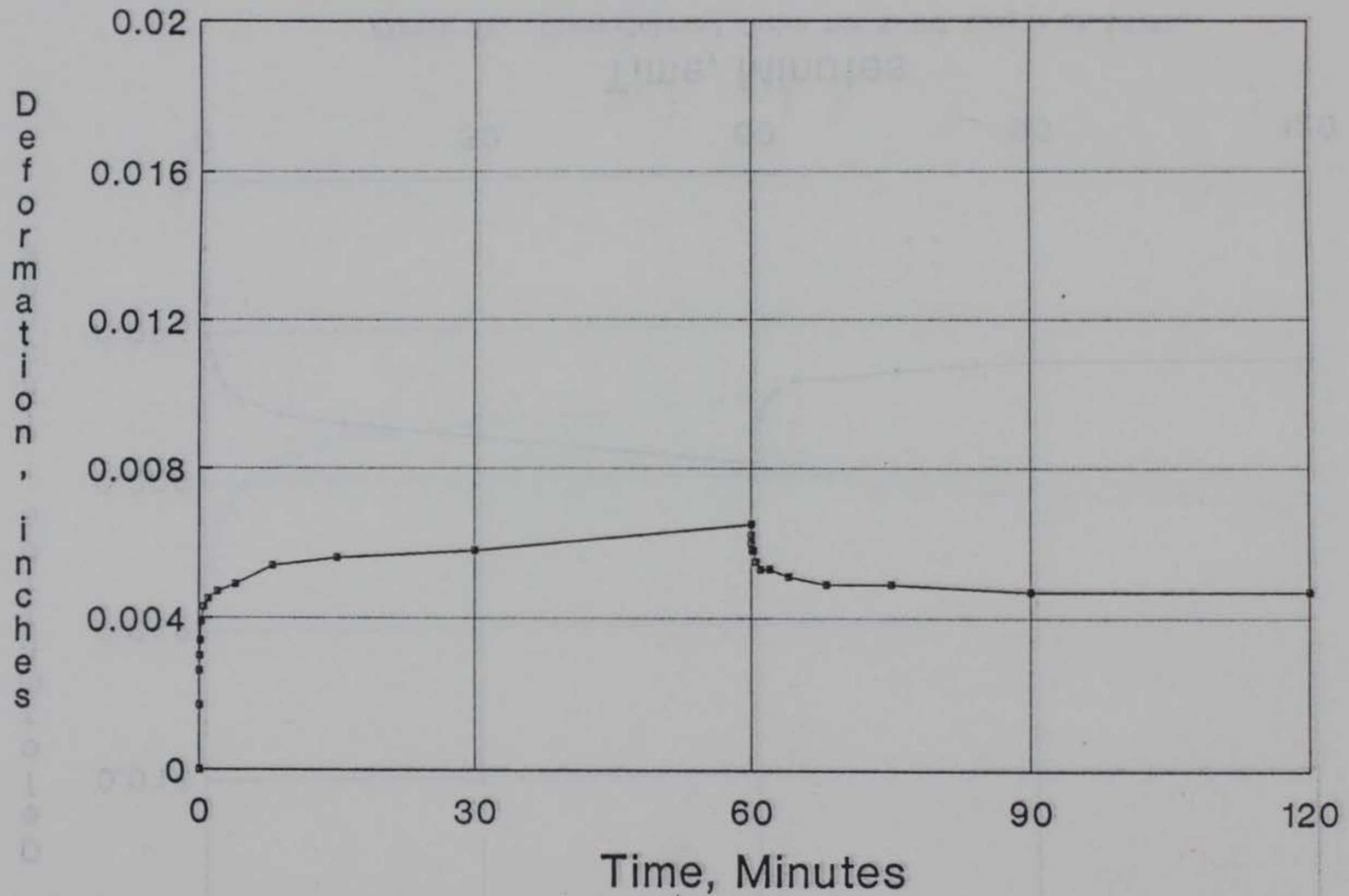
Figure 59. Creep-Rebound Curve for S-1M4 Sample at 104°F
