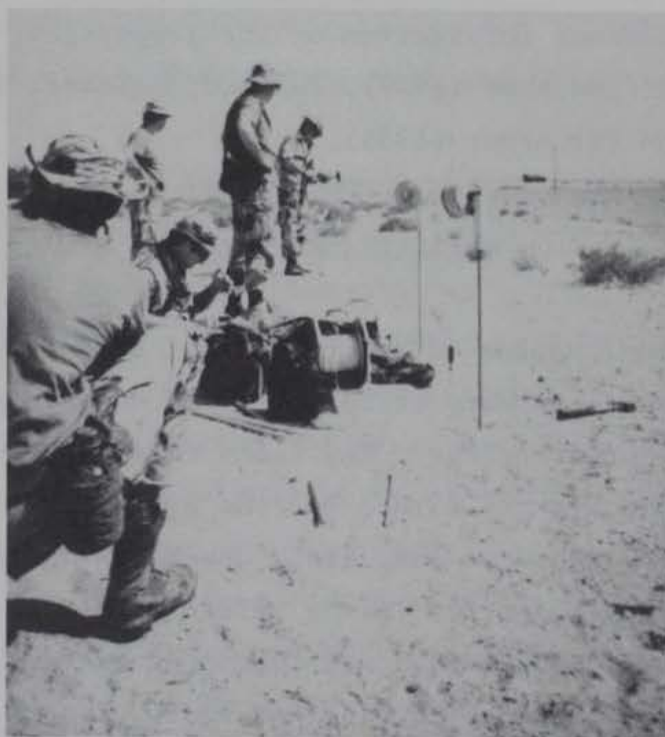
b. Electrical resistivity survey during Bright Star 85
