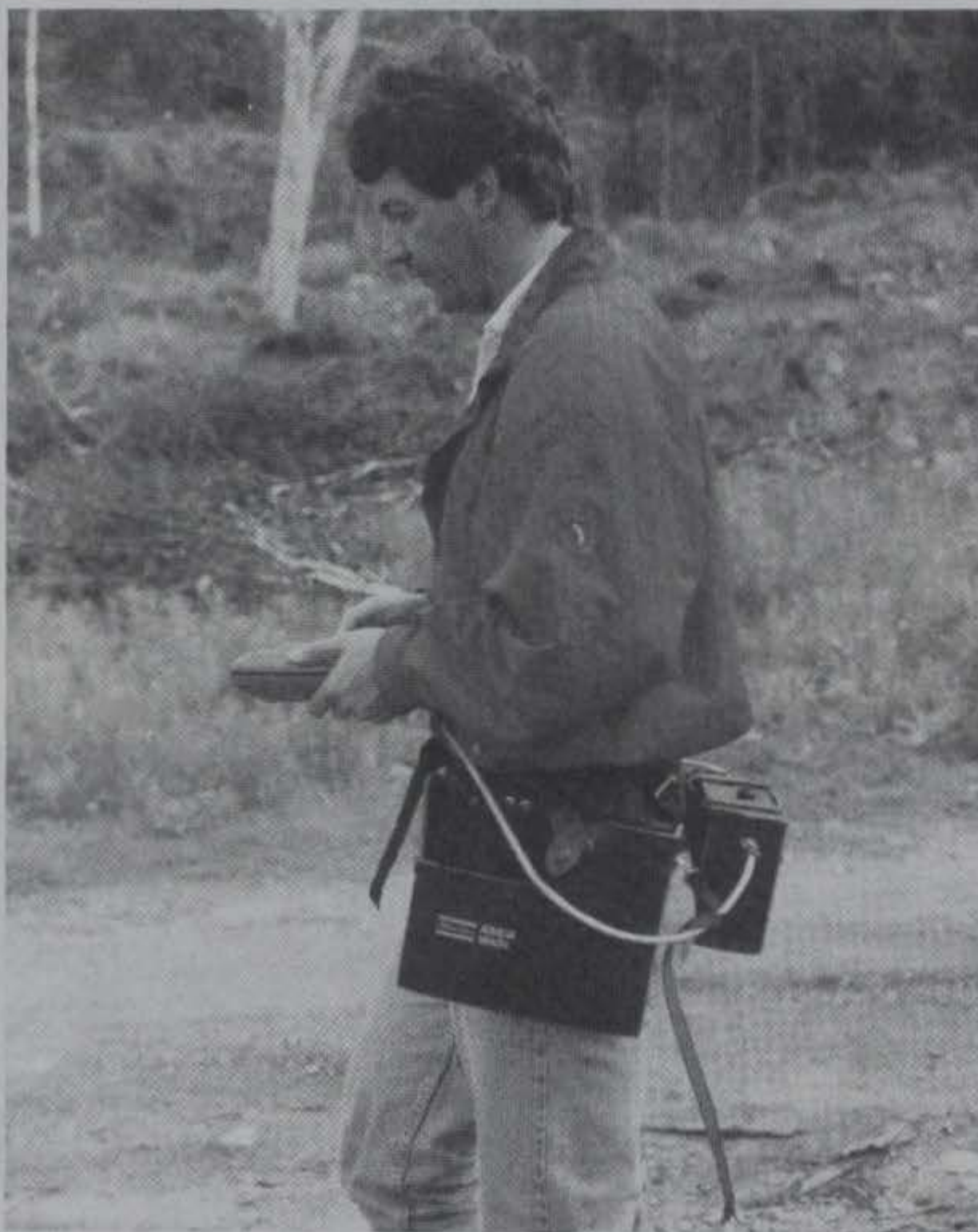
Figure 7. Very low frequency (VLF) electromagnetic equipment and survey in progress
