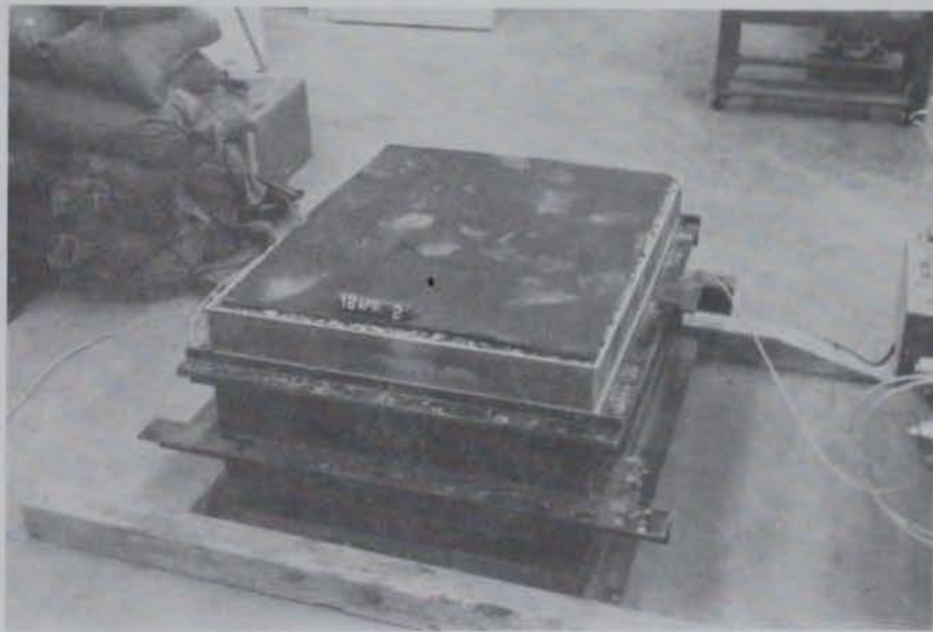
Photo 4. Pavement system prior to test
