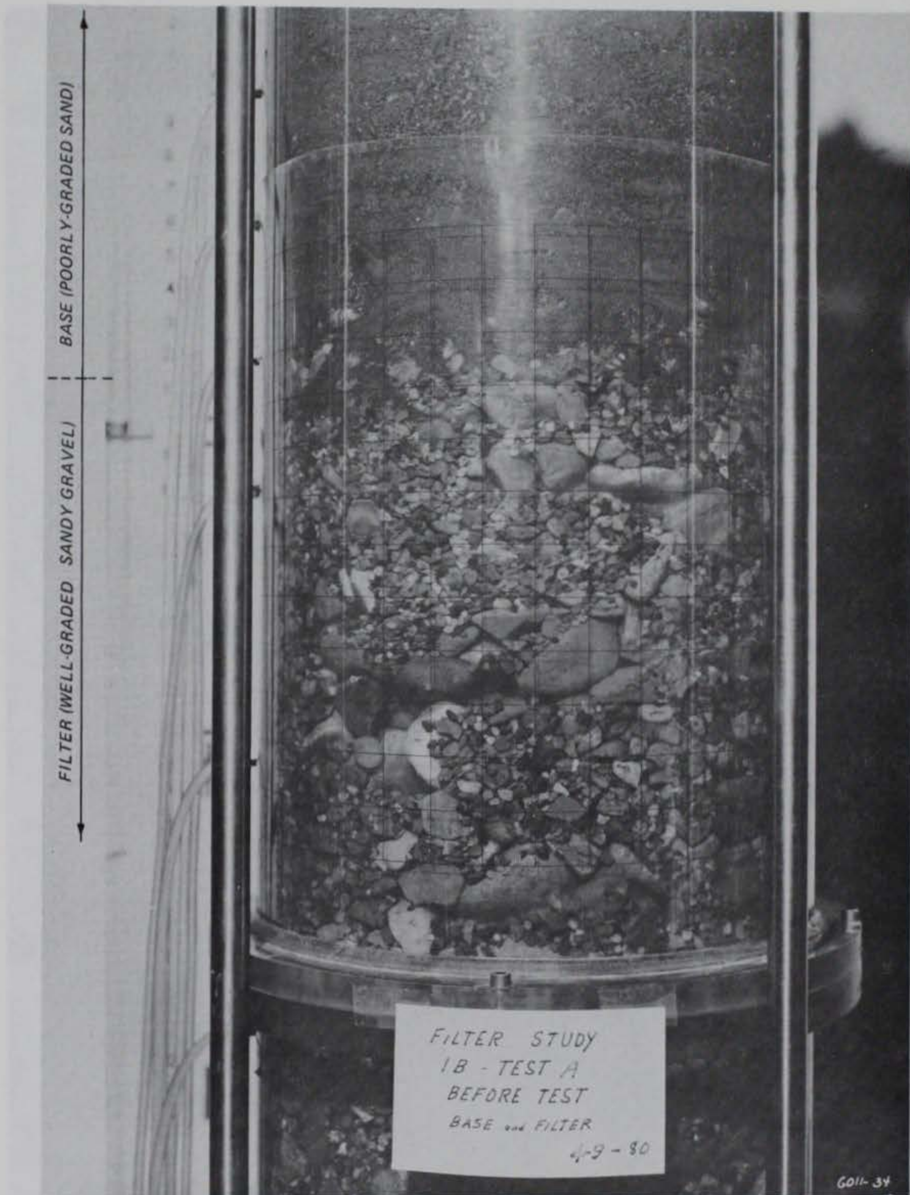
Figure 18. Top cylinder with grid before test for Test No. 1B-A
