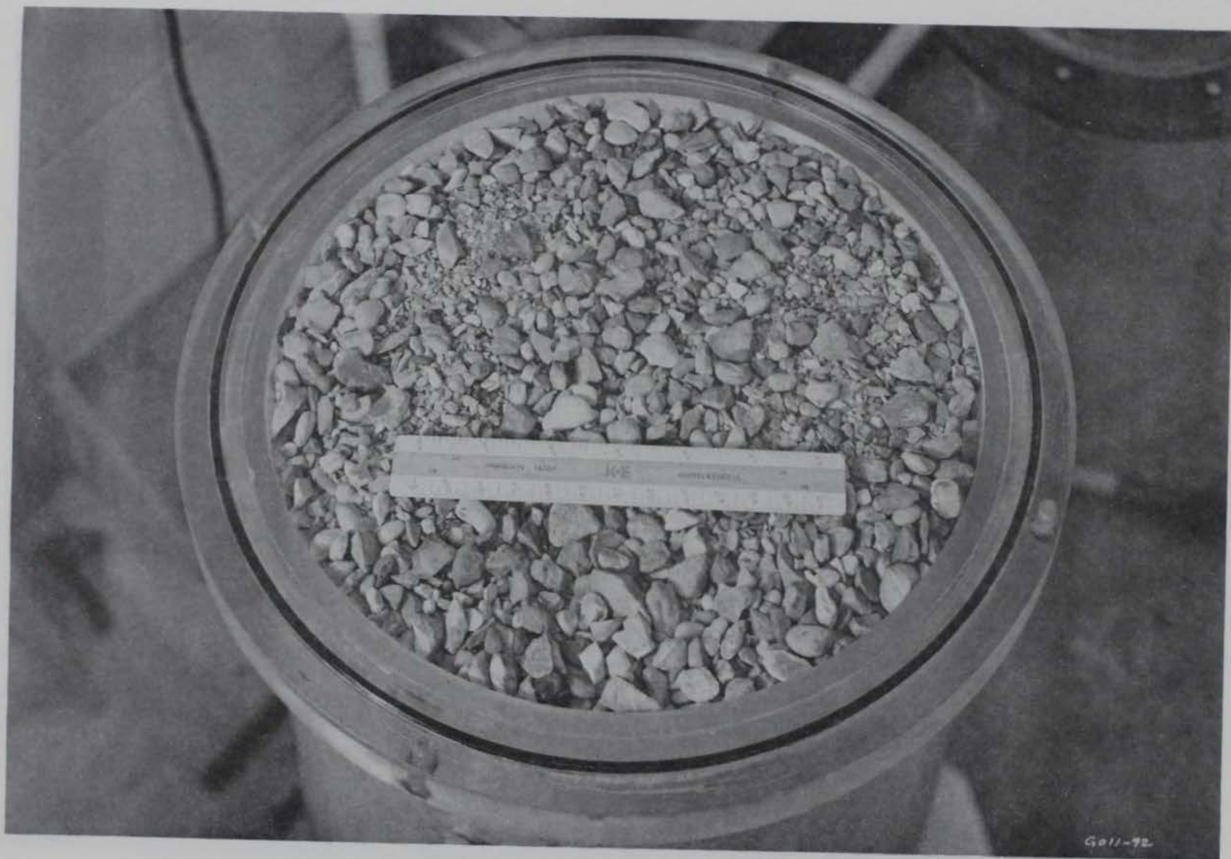
Figure 14. Bottom cylinder filled with O-ring in place (Material shown is a poorly-graded sandy gravel used in Test No. 3A as discussed in Part IV.)
