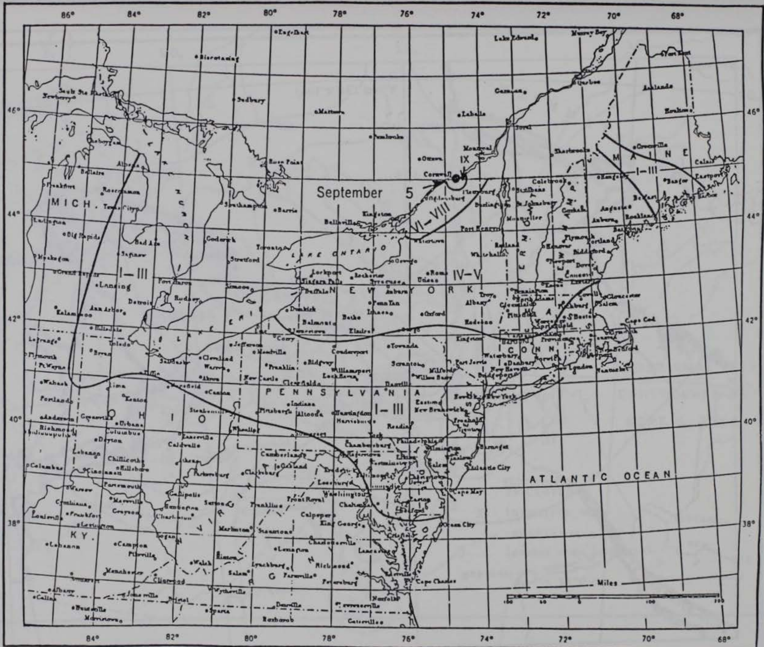
Figure 3. Isoseismal map of the United States portion of the 1944 Massena-Cornwall earthquake (Bodle, 1946).
