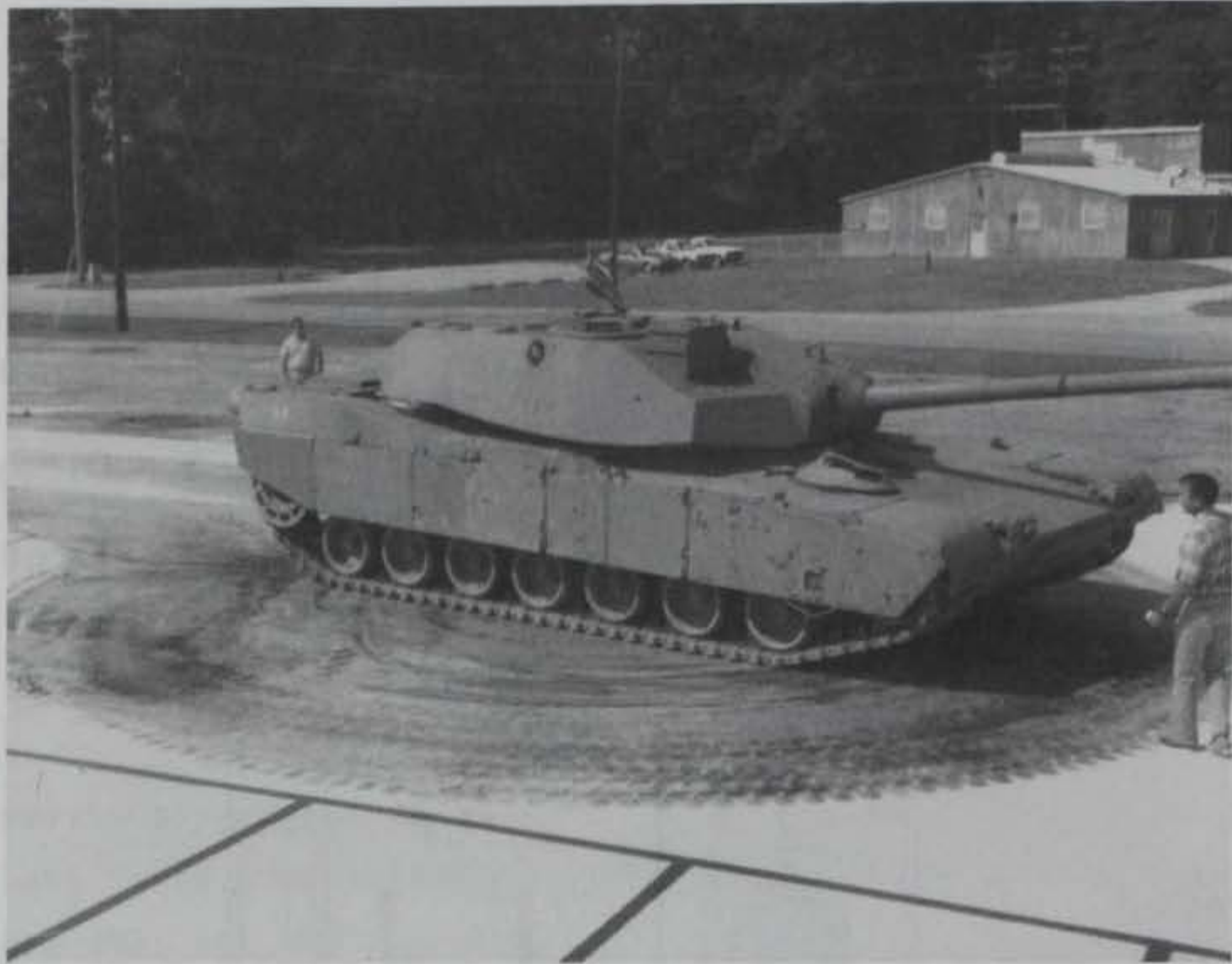
Figure 12. M1 tank performing pivot steer turns on RMP test strip (note rubber on pavement surface)
