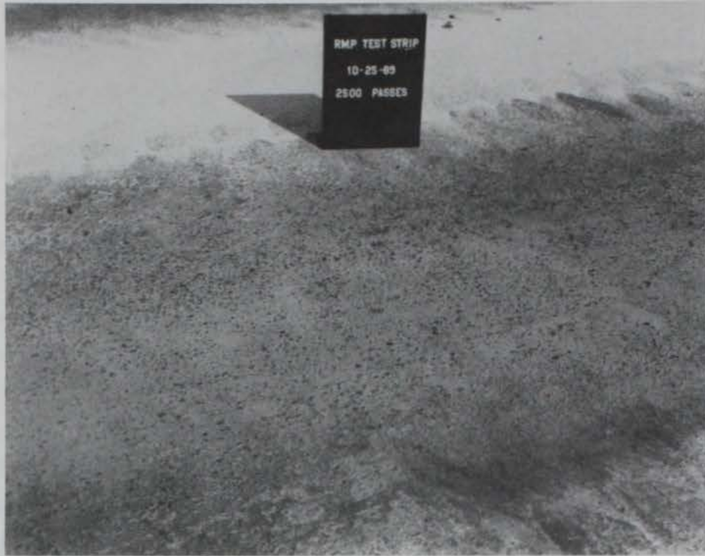
Figure 19. RMP after 2,500 straight passes
