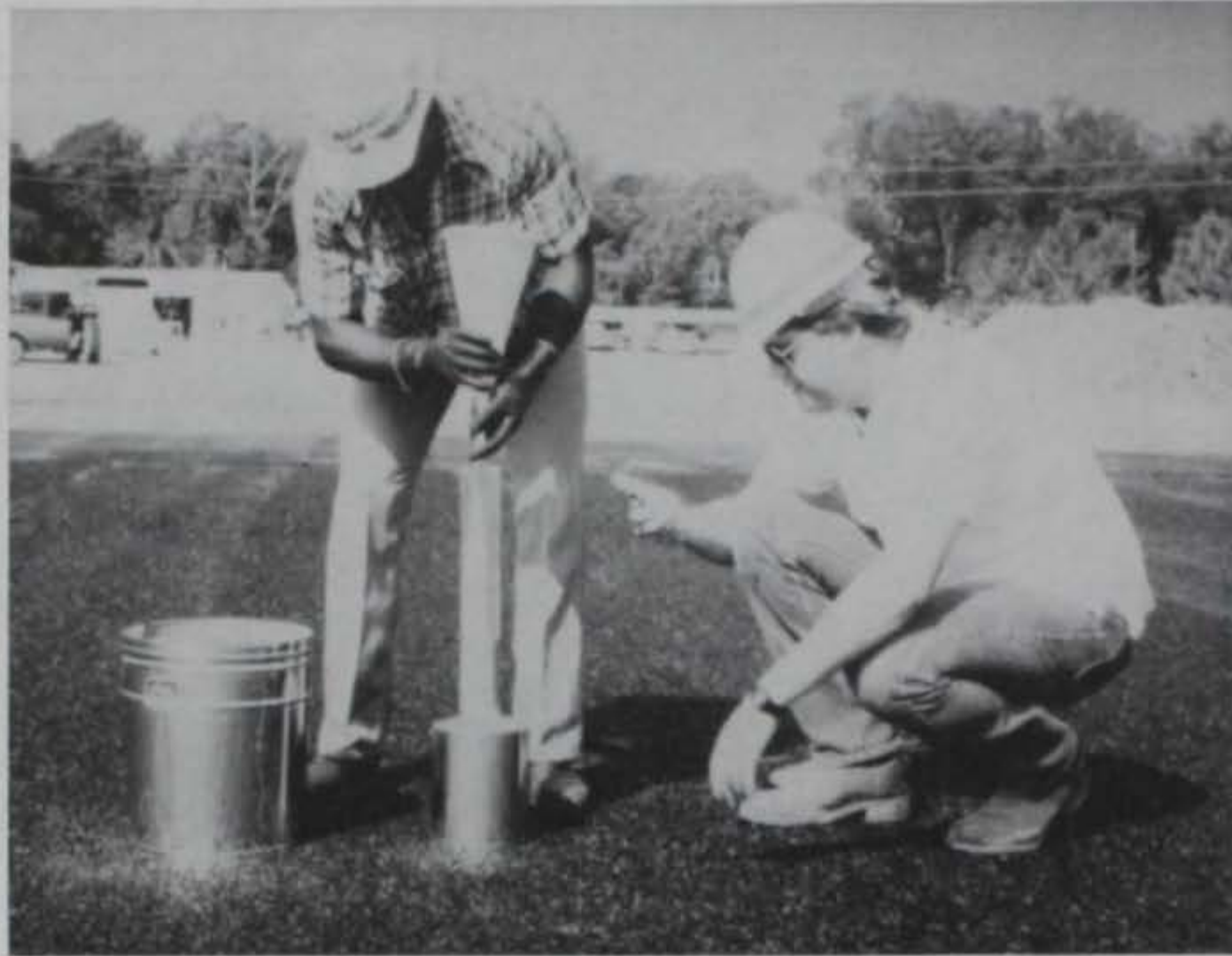
Figure 8. Testing slurry grout with Marsh flow cone
