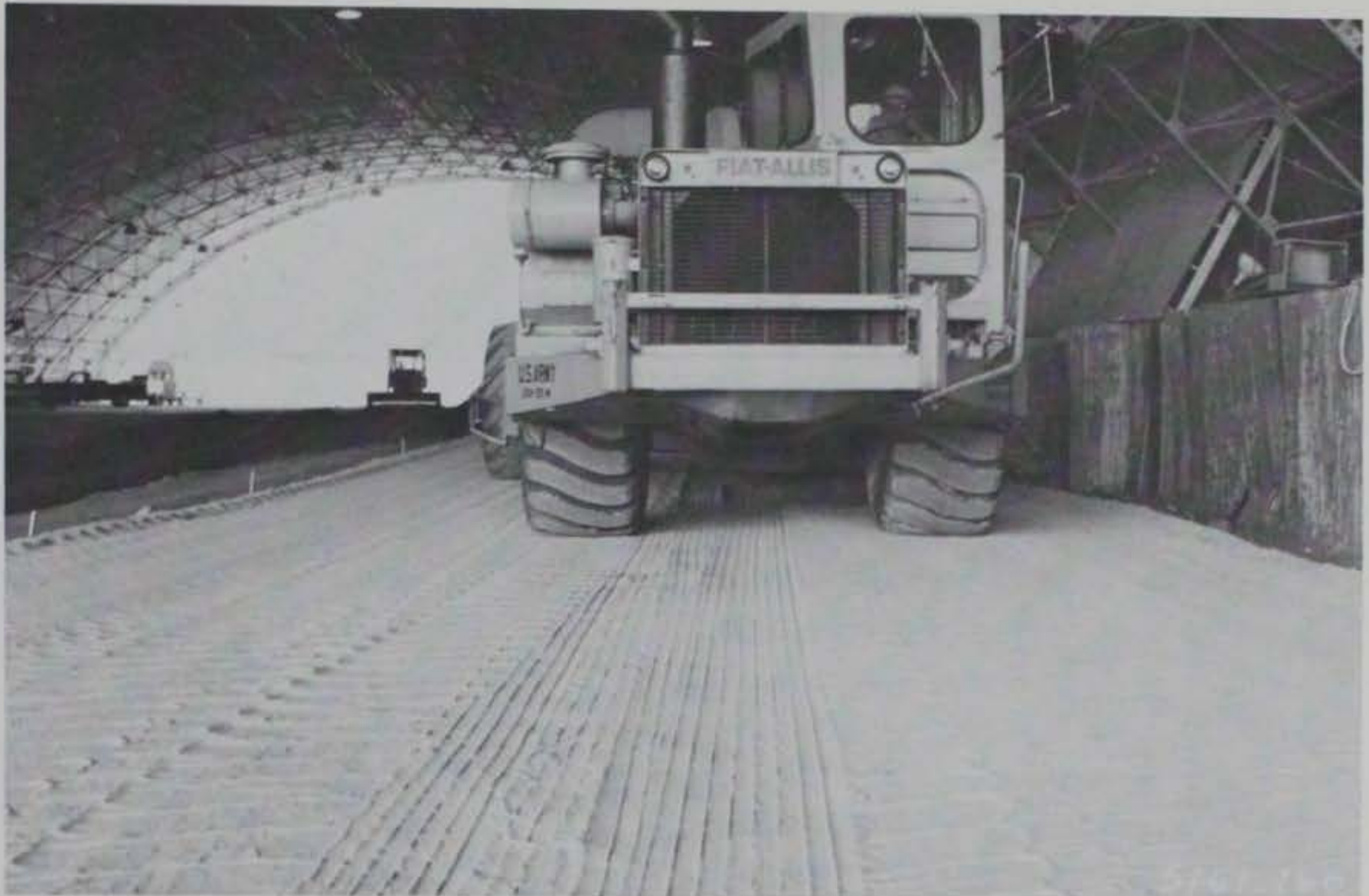
Photo 89. Traffic being applied with 70-kip, single-tandem gear test cart
