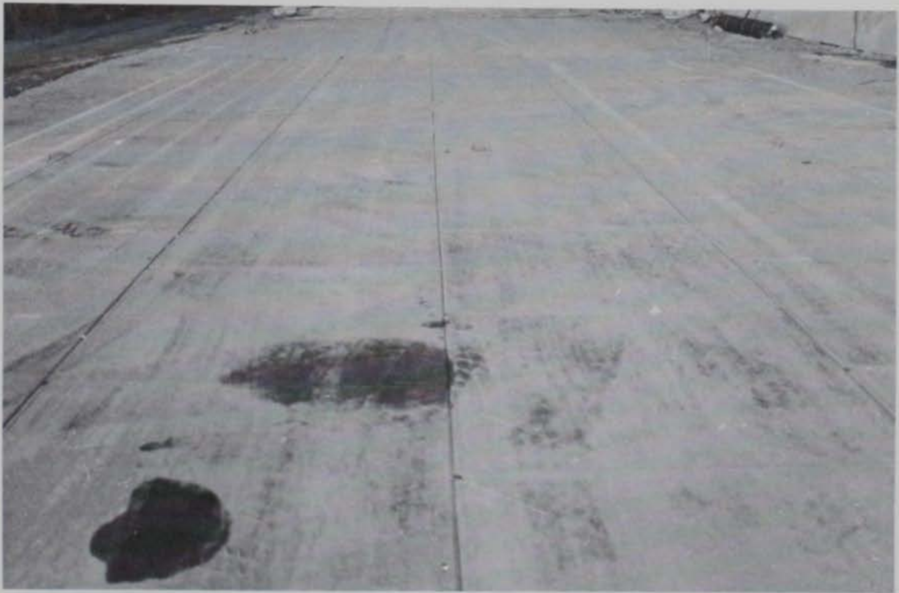
Photo 6. General view of XML9 landing mat, Test Section No. 1, item 1, after traffic
