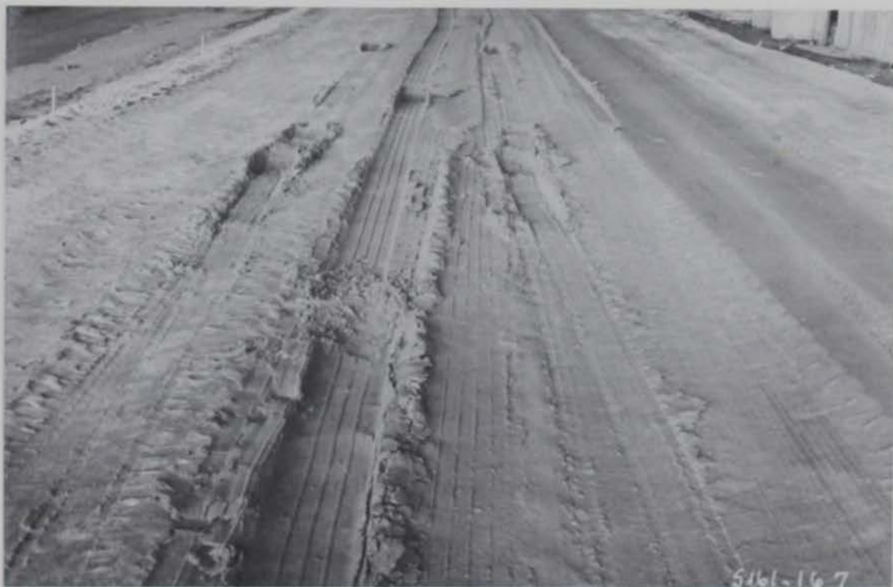
Photo 94. General view of Test Section No. 5 after four passes of F-4C load cart
