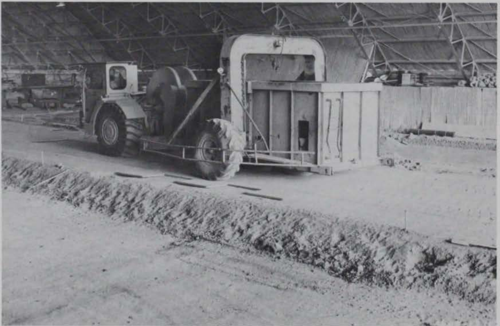
Figure 2. Seventy-kip single-tandem test cart
