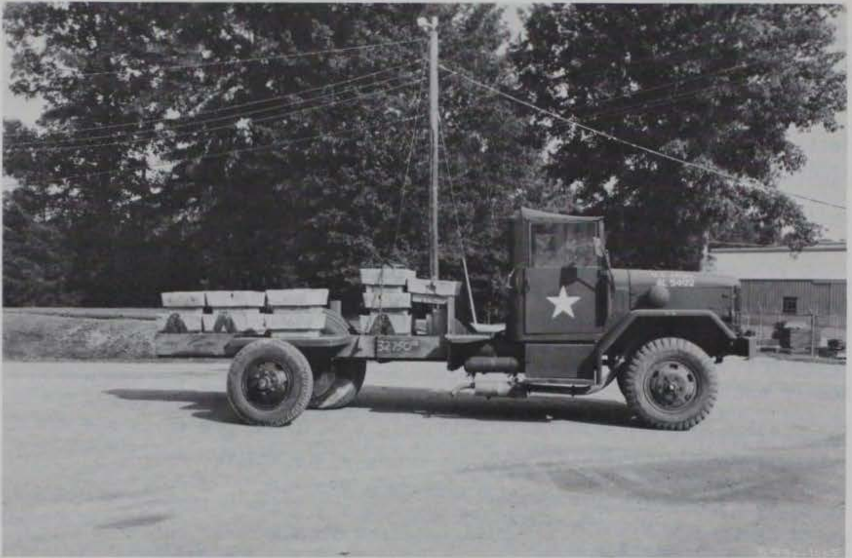
Figure 1. Thirty-five-kip single-wheel test cart
