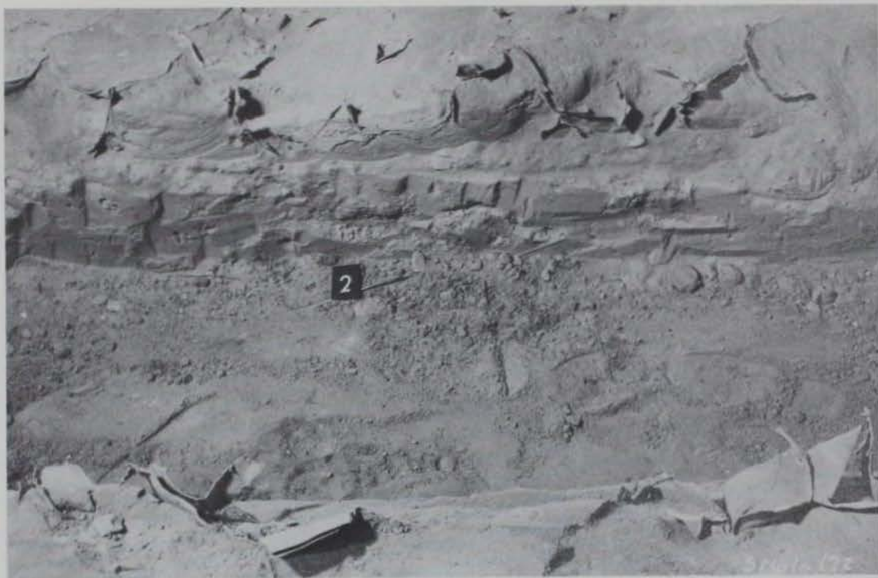
Photo 99. Trench in Test Section No. 5, item 2, after traffic
