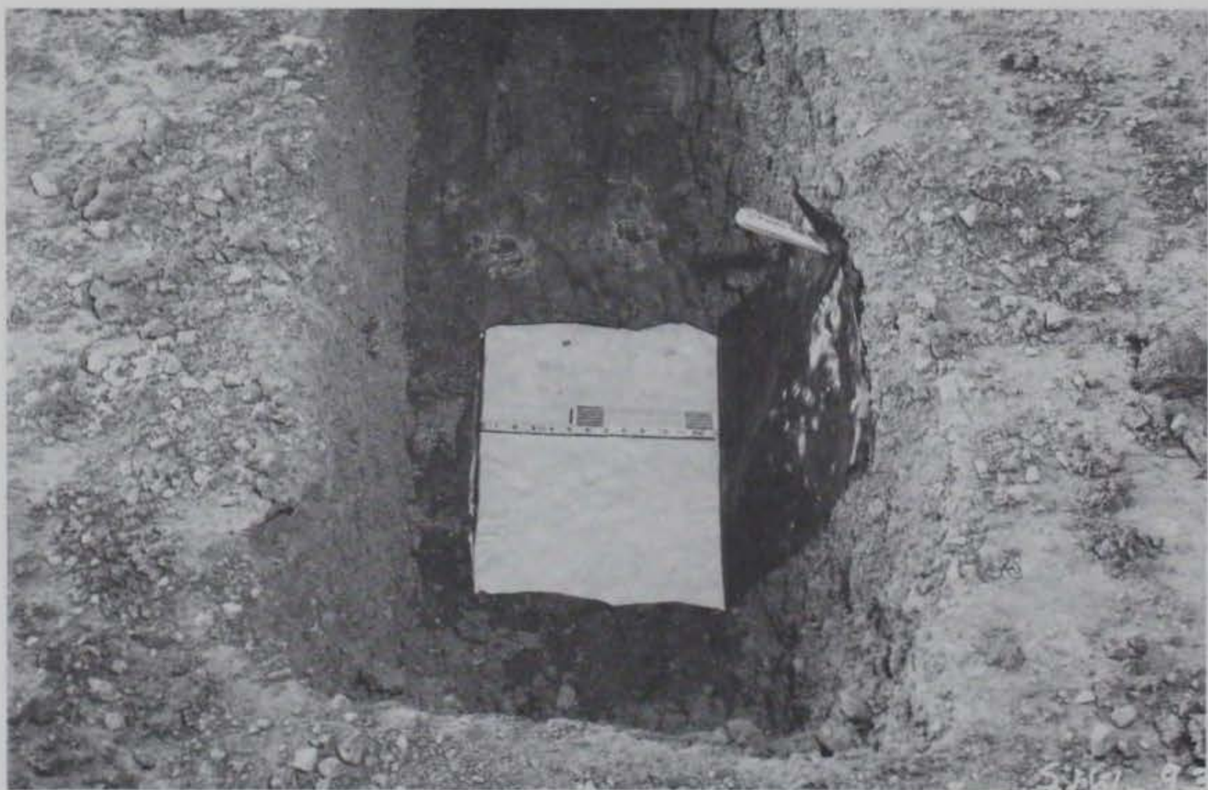
Photo 72. Surface of Styrofoam, Test Section No. 4., item 1, after 480 passes
