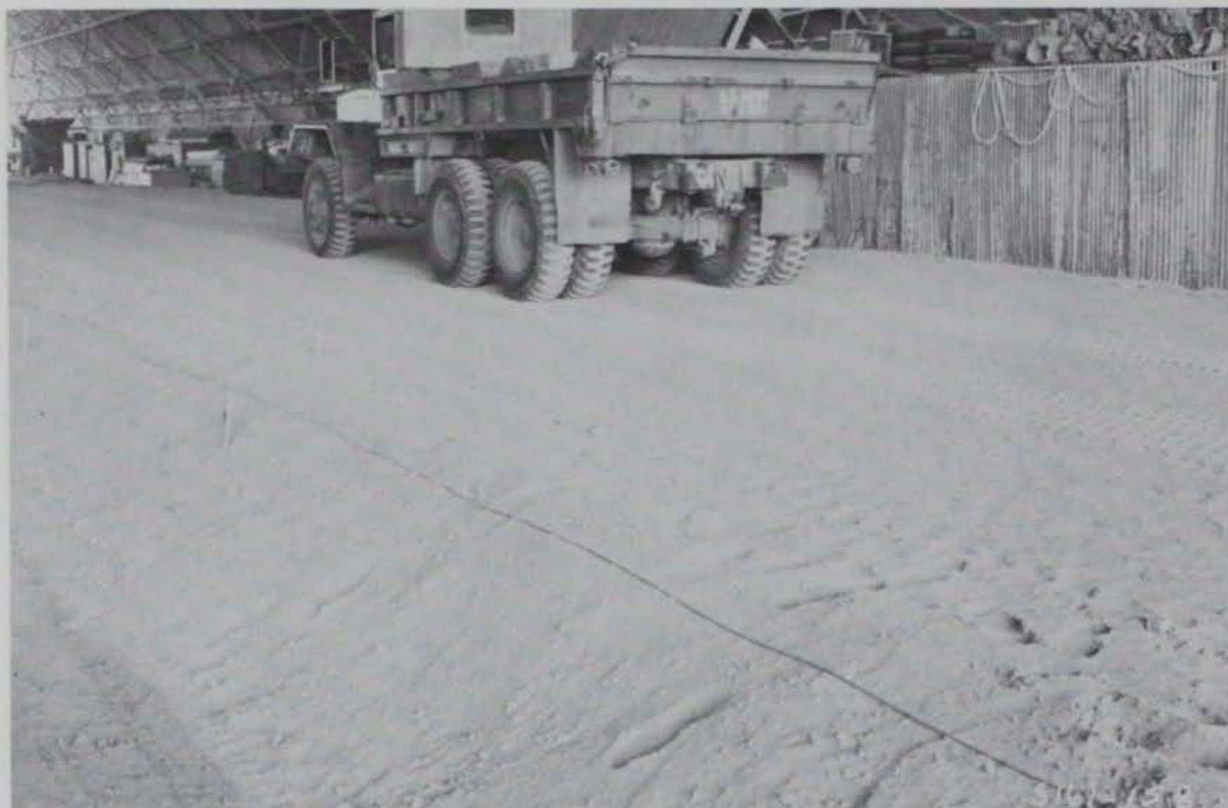
Photo 87. Traffic being applied with 40-kip, 6 x 6 military truck
