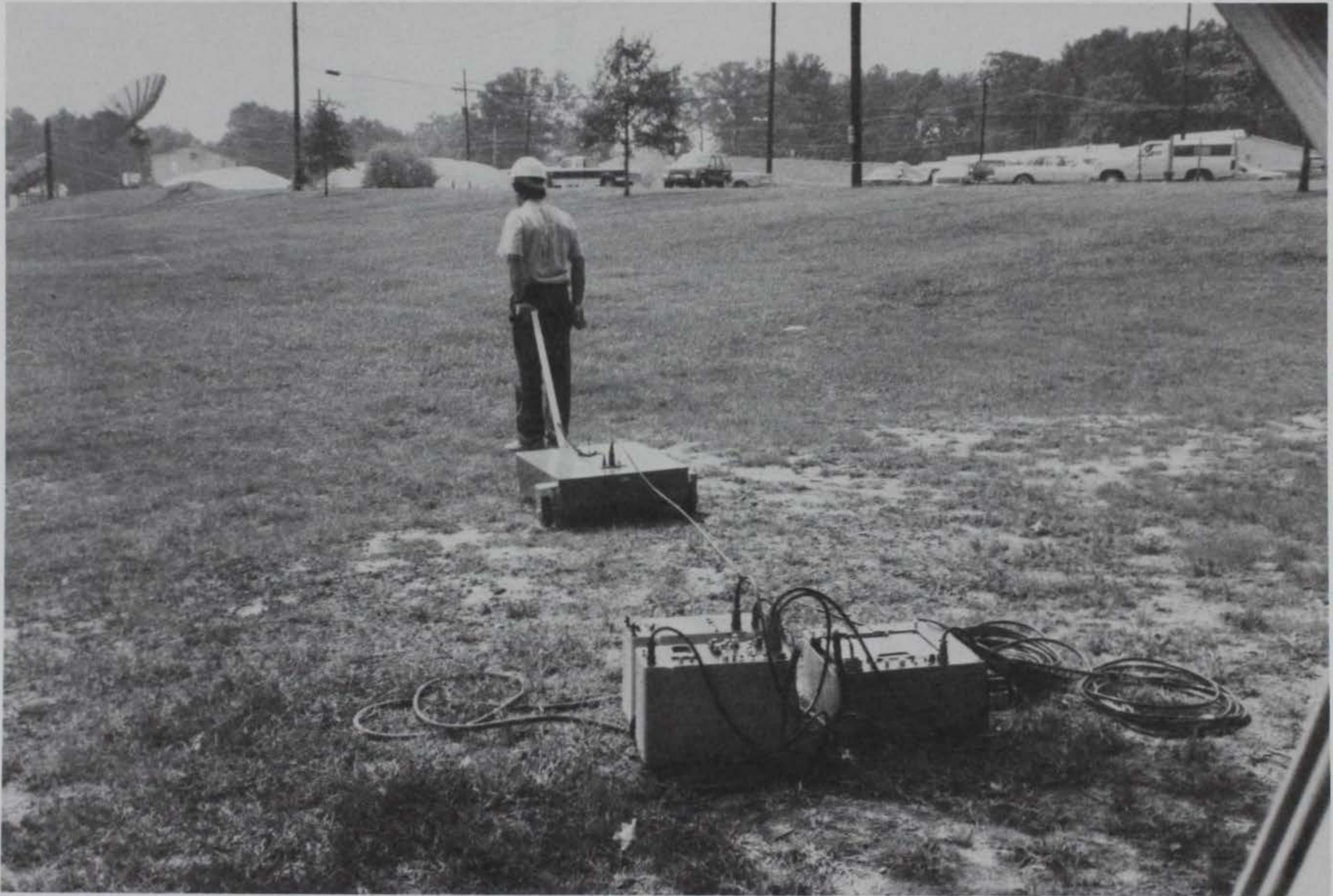
Figure 6. GSSI System 8 GPR with 300 Mhz antenna
