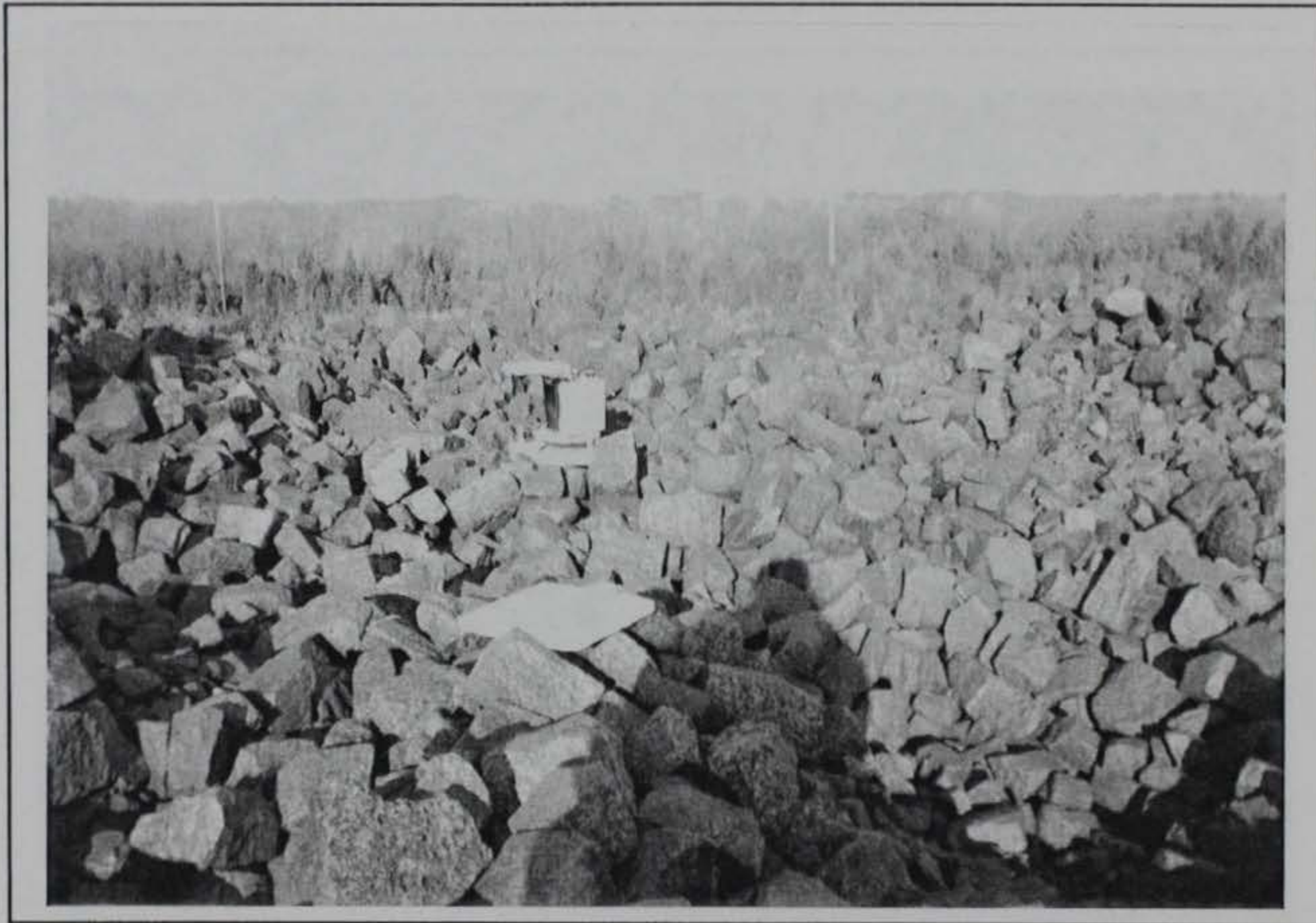
Figure 6. Microgravity stations positioned on top of ferromanganese pile
