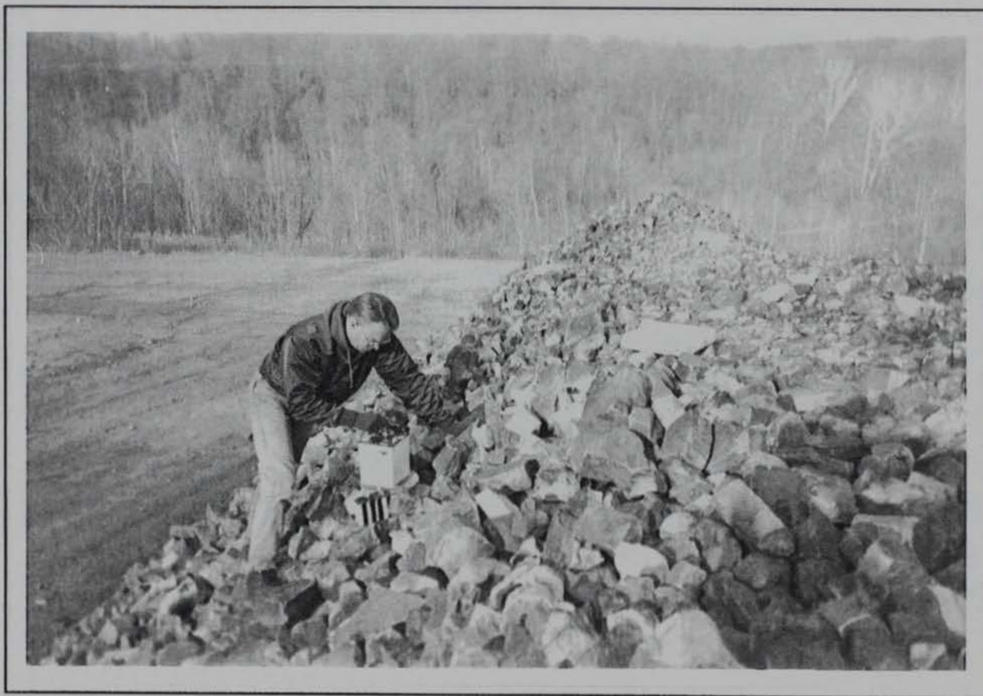
Figure 10. Microgravity measurement near the crest of an ore pile
