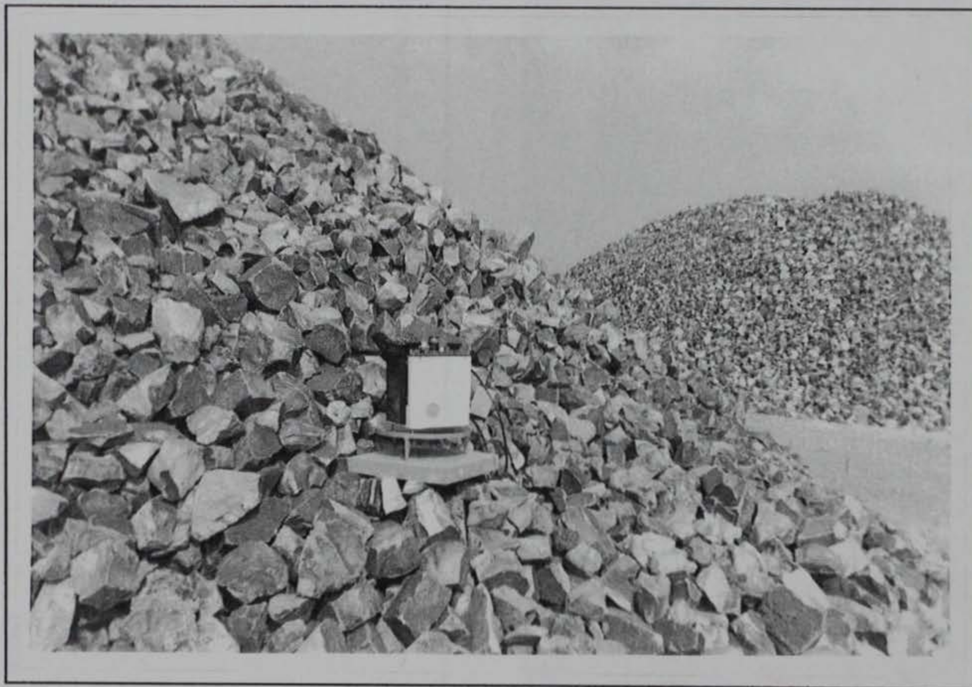
Figure 4. Microgravity measurement station on Pile #56, New Haven Depot, IN
