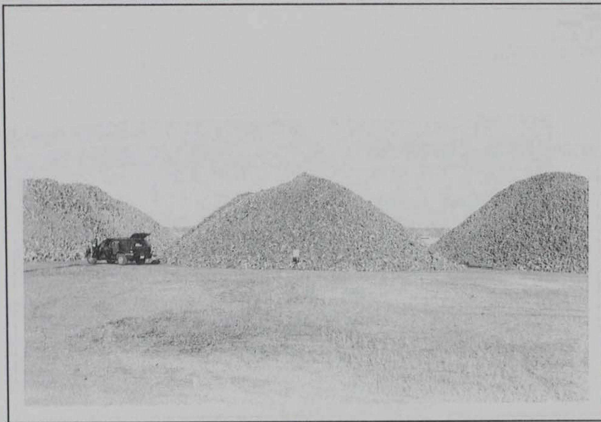
Figure C-27. Pile #3, Warren Depot, OH. Pile is composed of high-carbon ferrochrome
