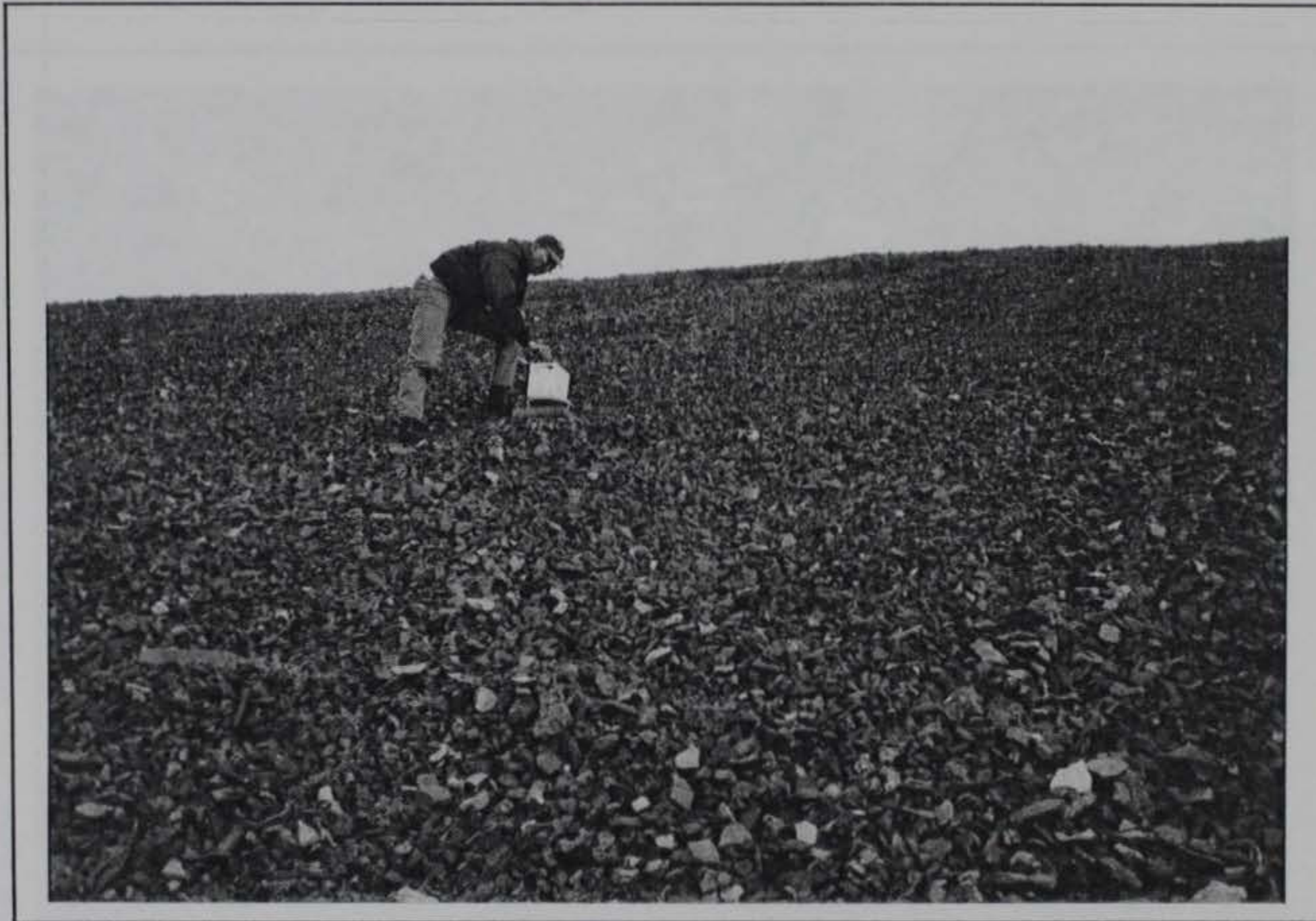
Figure 9. Microgravity measurement on side slope of pile
