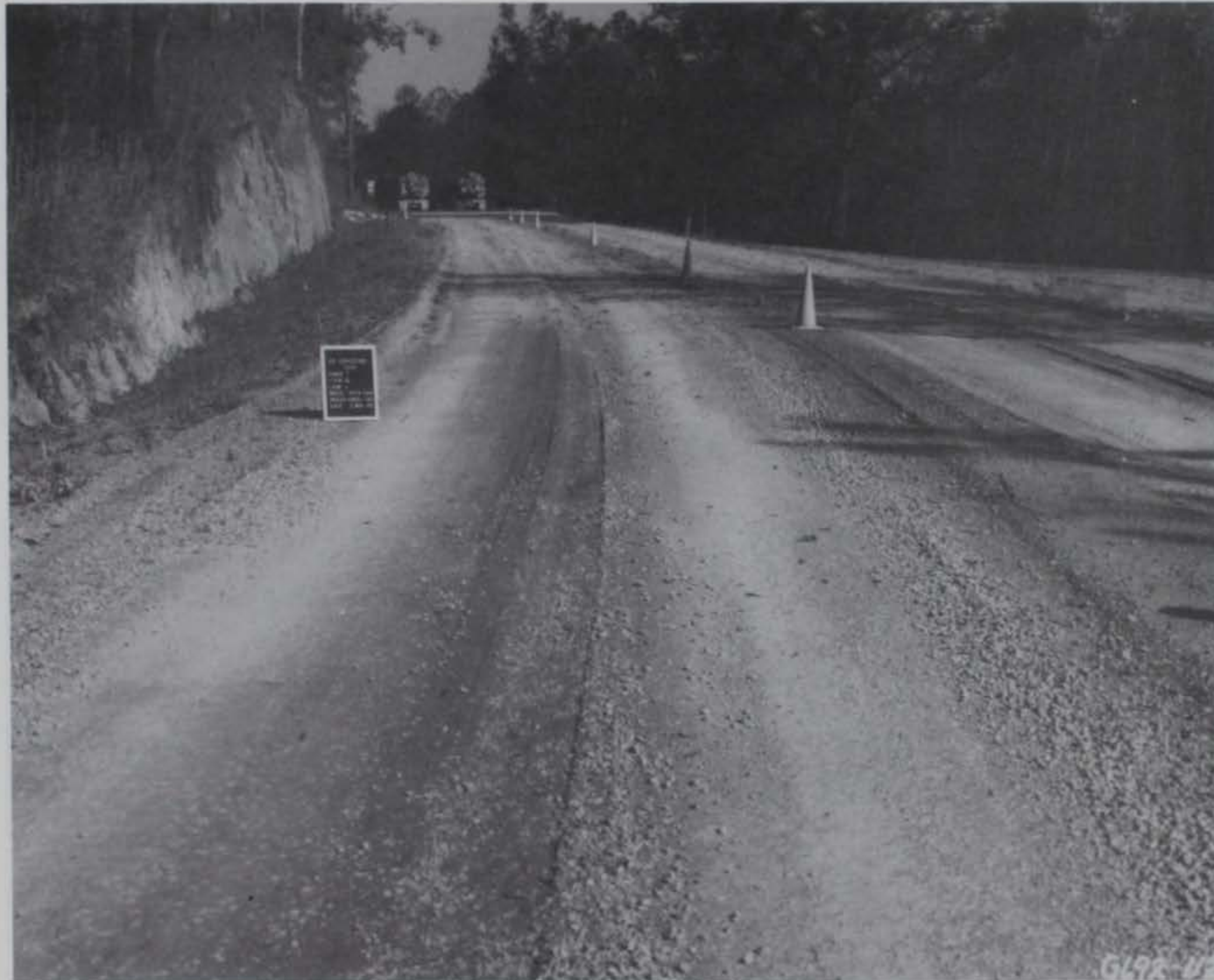
Photo 57. Item 14, low-pressure tire lane, general view after 130 passes during the induced failure plan
