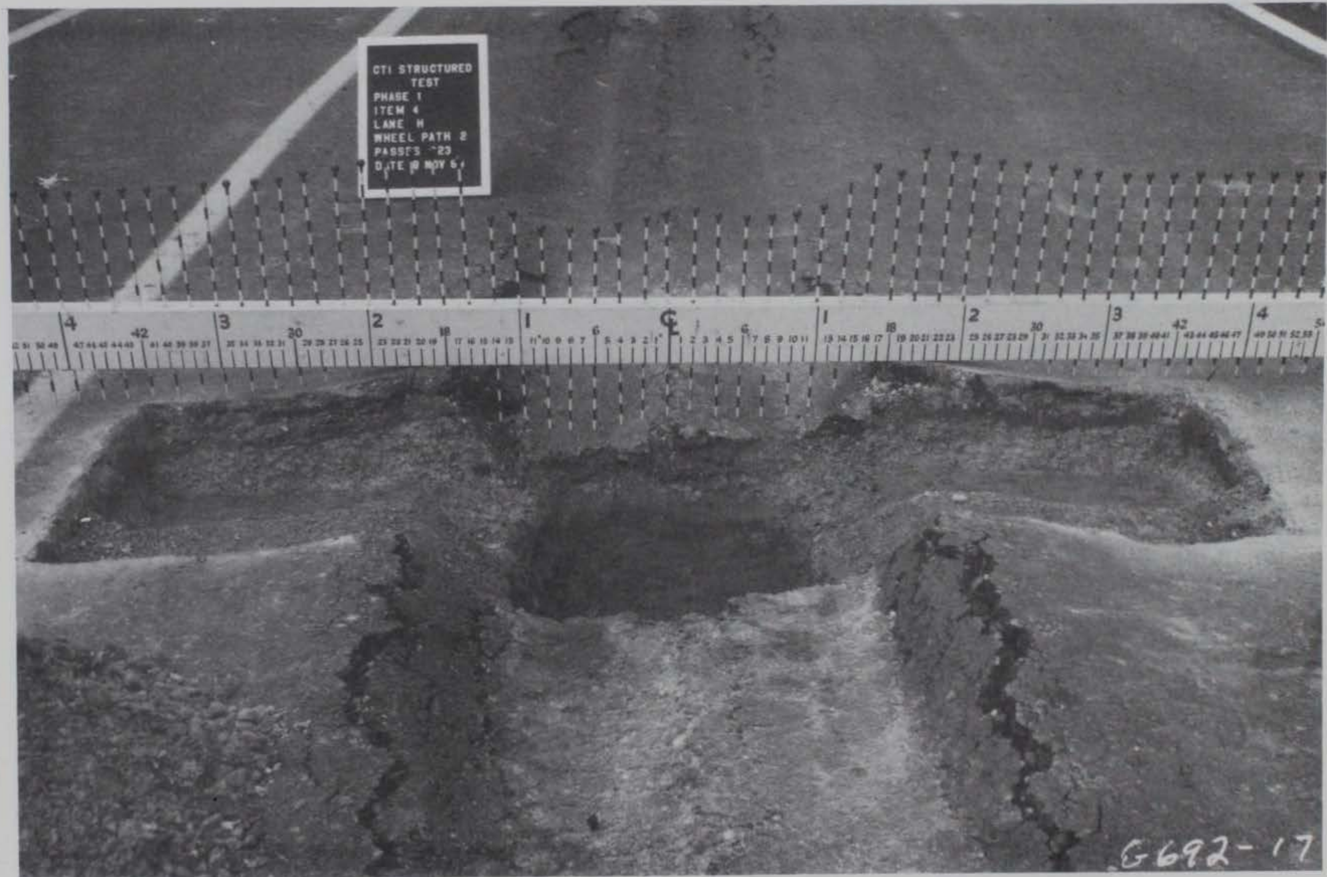
Photo 15. Item 4, wheel path 2, test trench after 323 passes
