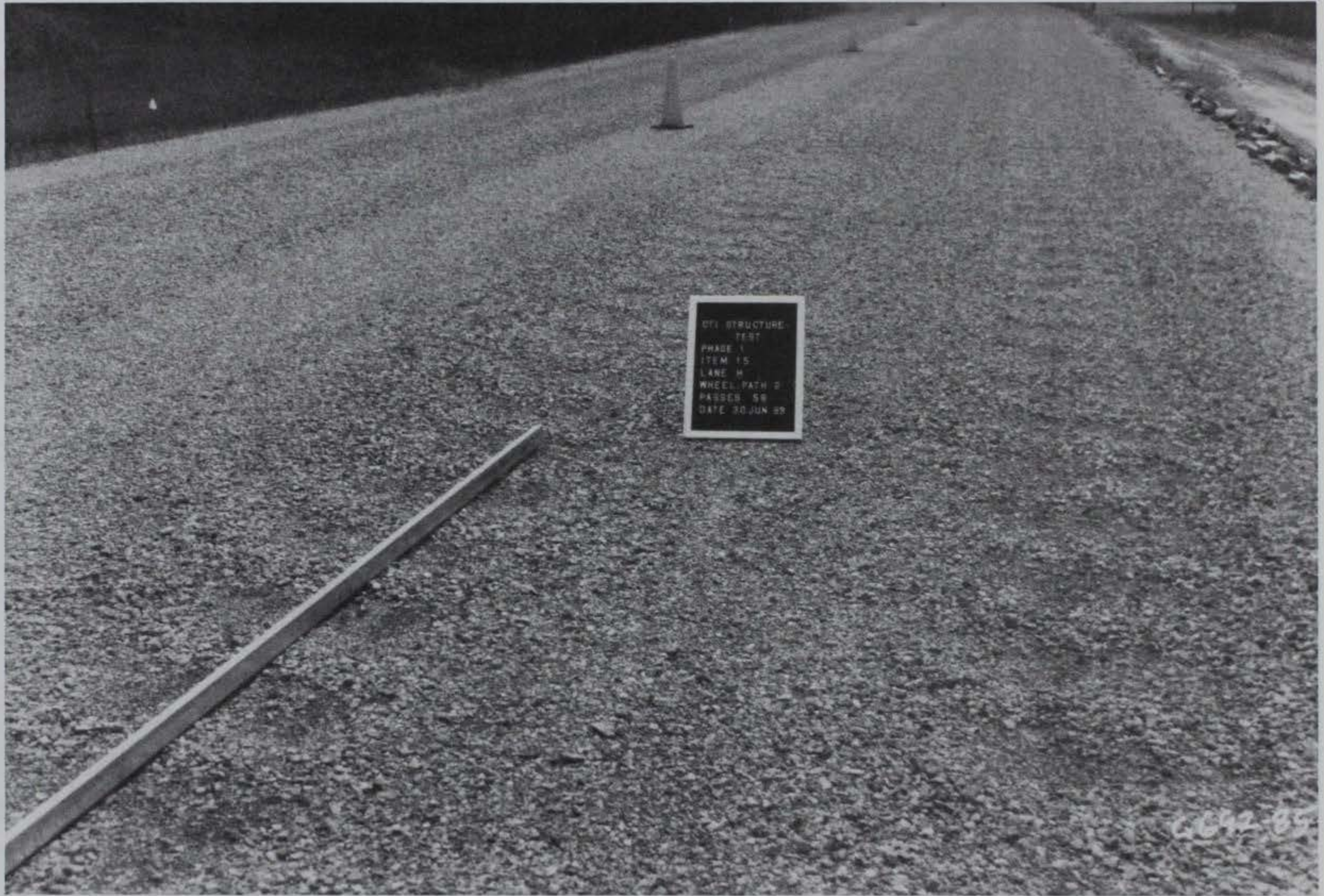
Photo 46. Item 15, high-pressure tire lane, low-severity washboarding after 58 passes
