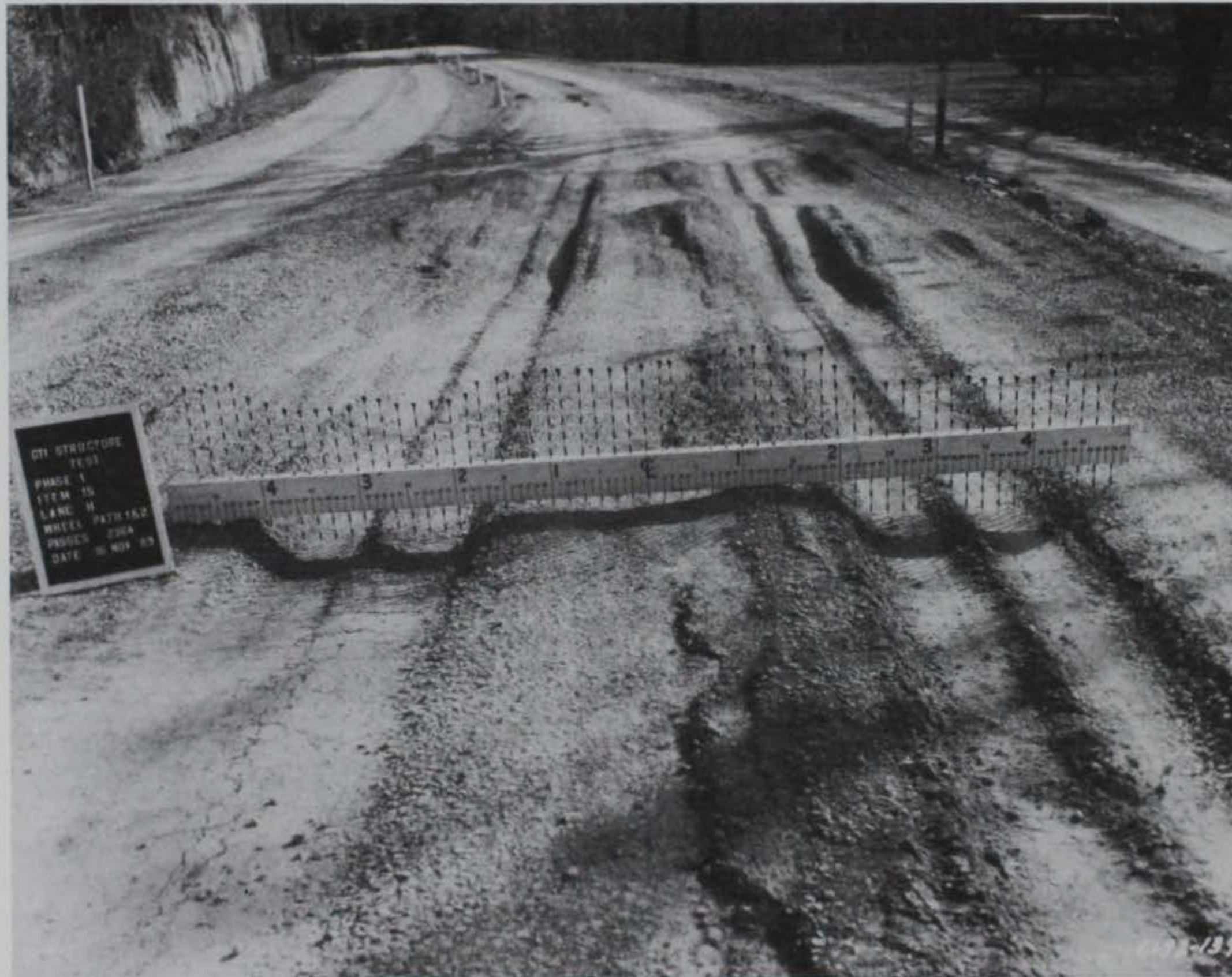
Photo 67. Item 15, high-pressure tire lane, severe rutting and loose aggregate after 913 passes of induced traffic for a total of 2364 loaded passes
