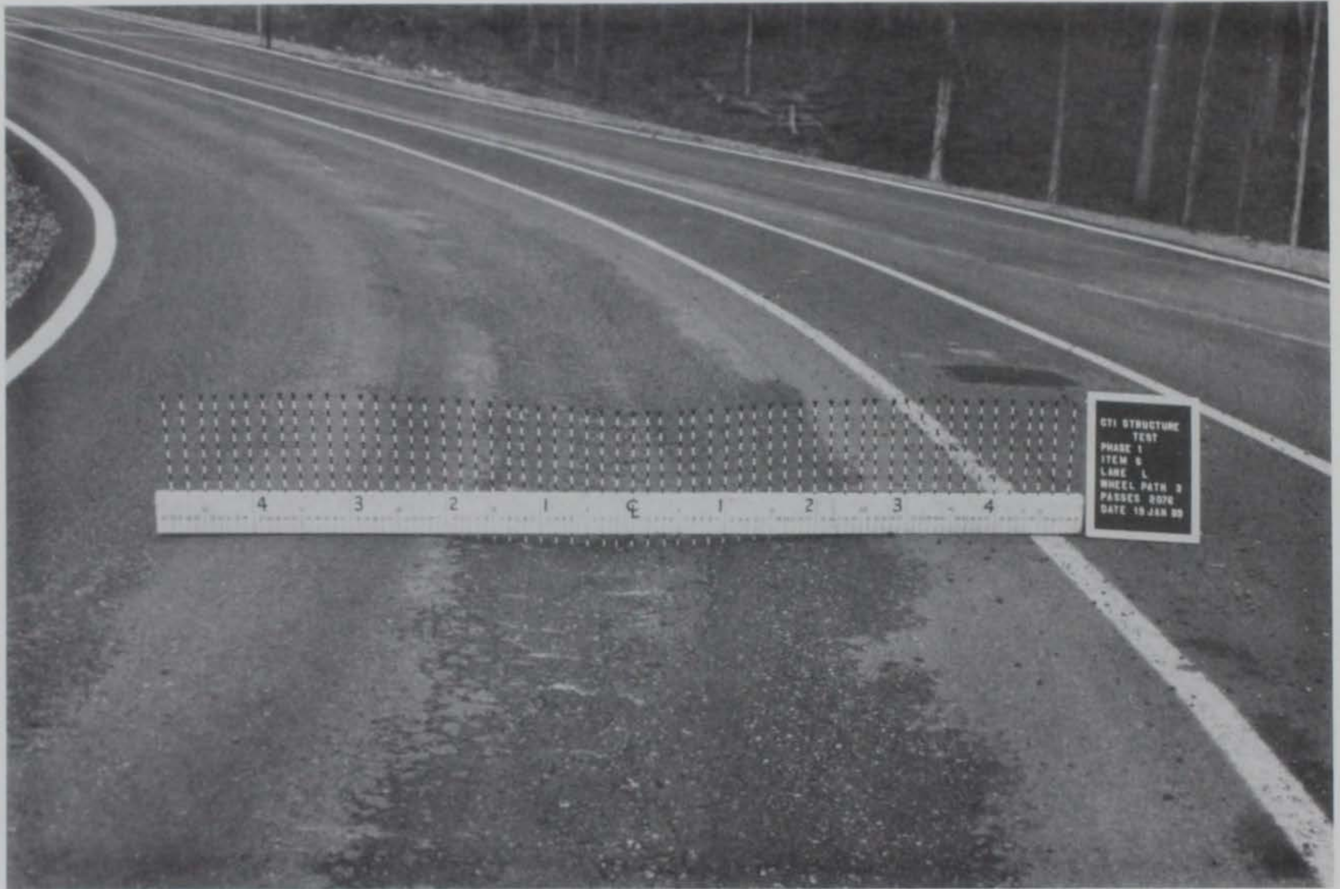
Photo 22. Item 6, wheel path 3, general failure after 2,076 passes
