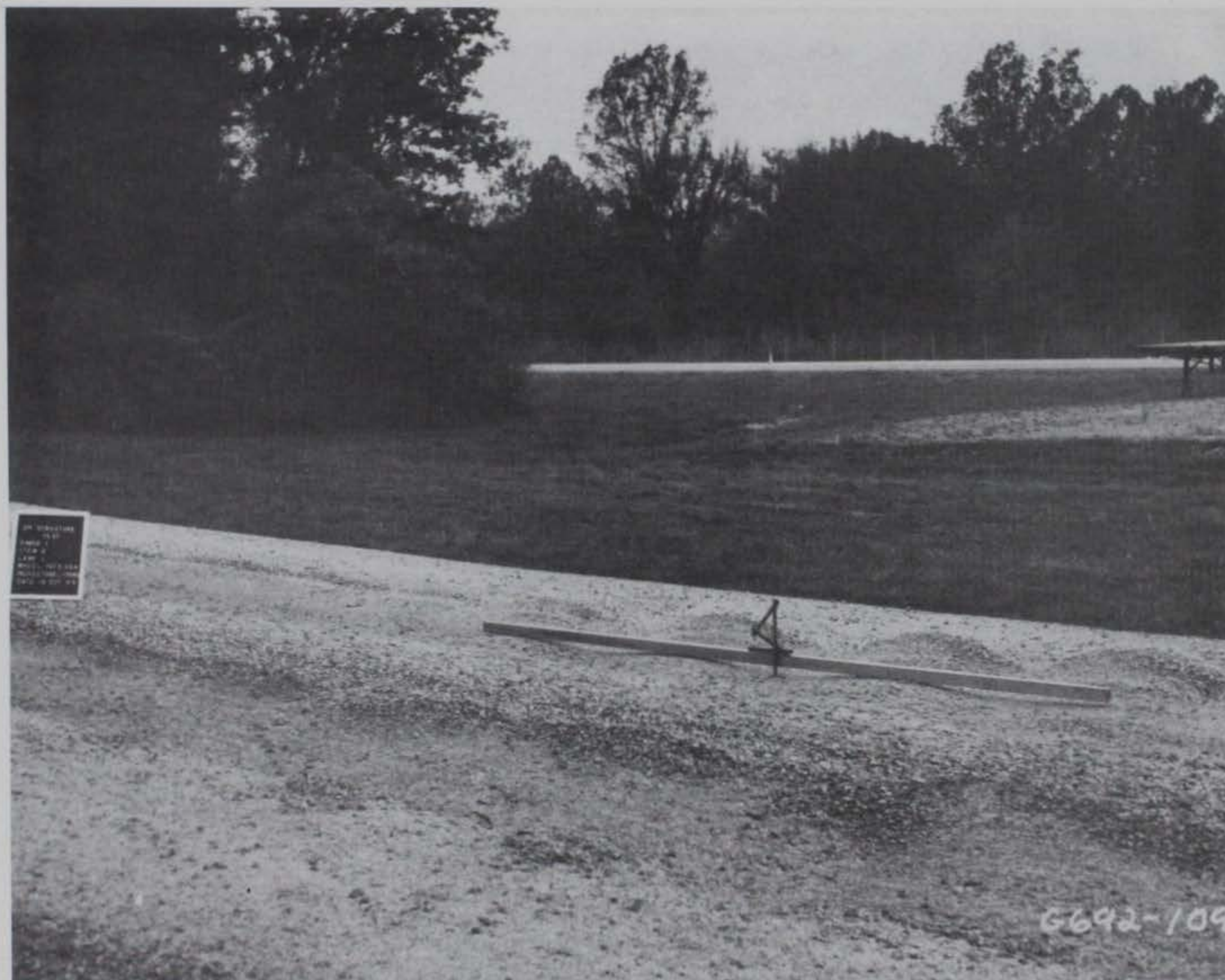
Photo 49. Item 2, low-pressure tire lane, long intervals between corrugation
