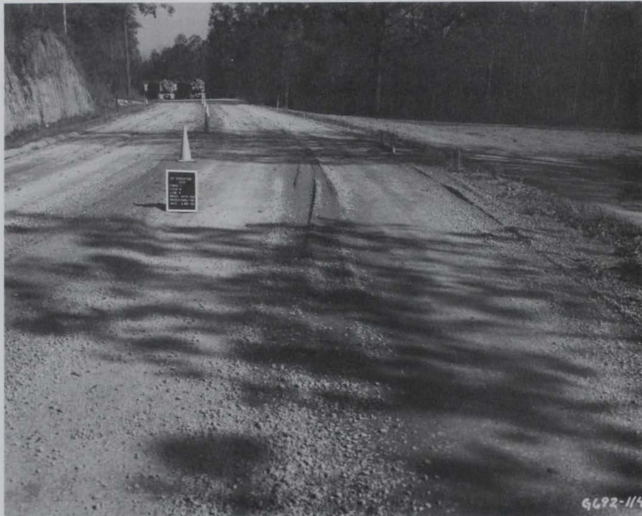
Photo 60. Item 14, high-pressure tire lane, general view after 139 passes during the induced failure plan
