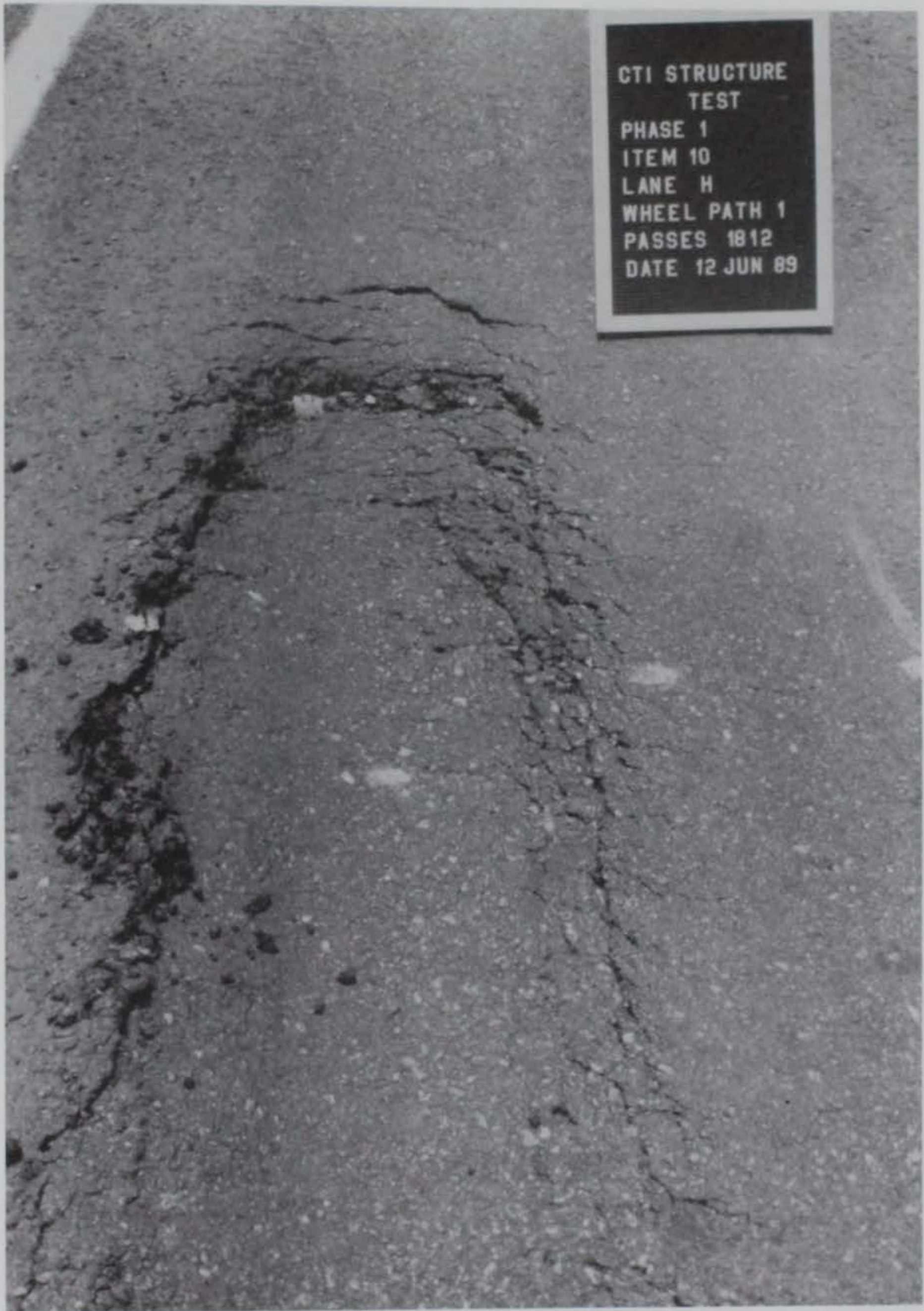
Photo 31. Item 10, wheel path 1, high-severity shoving after 1,812 passes
