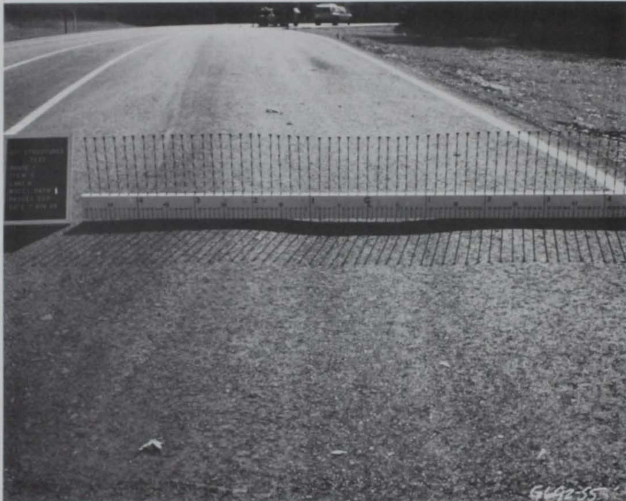
Photo 16. Item 5, high-tire pressure lane, maximum 1-in. rutting after 323 passes
