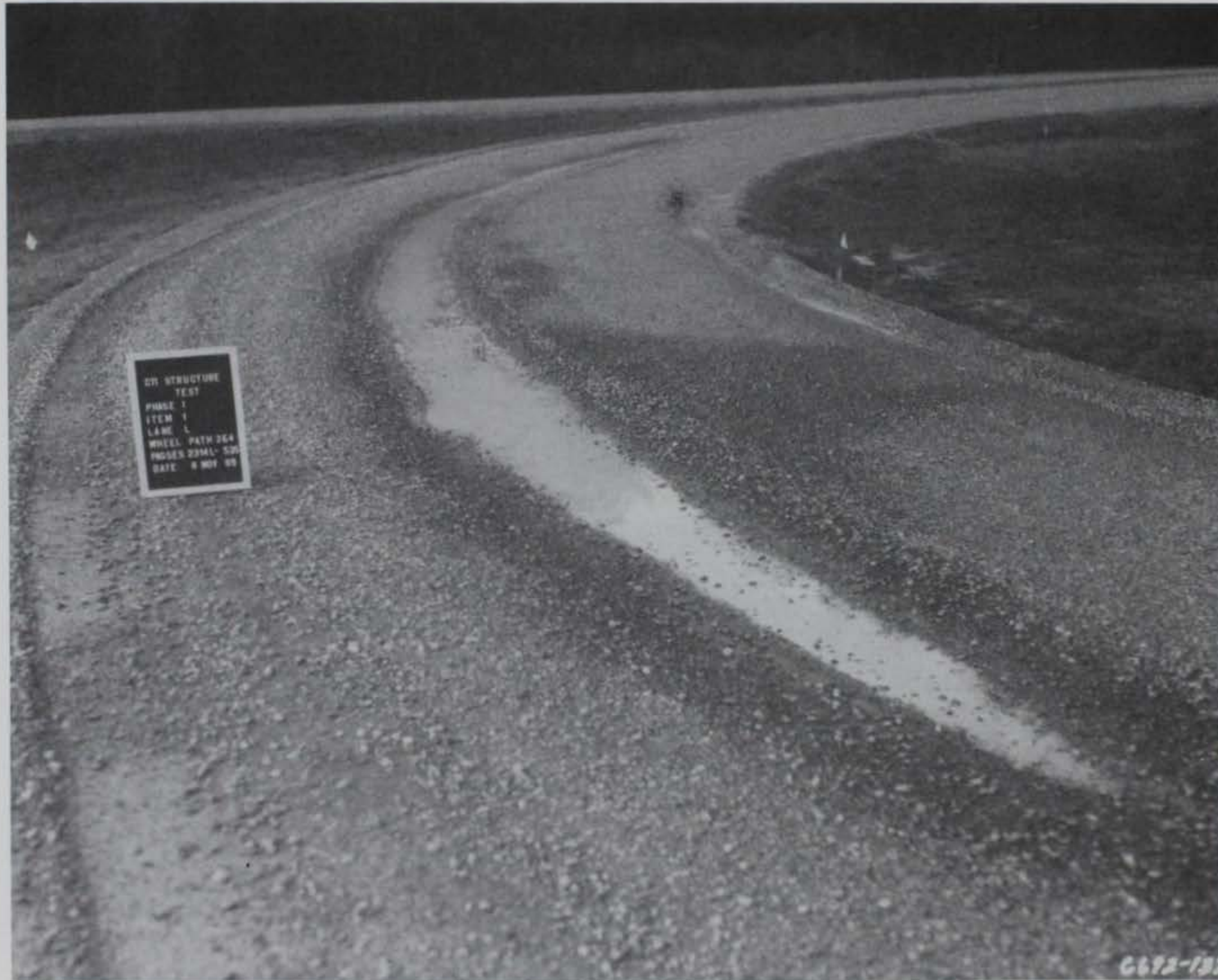
Photo 51. Item 1, low-pressure tire lane, low-severity rutting at the end of traffic
