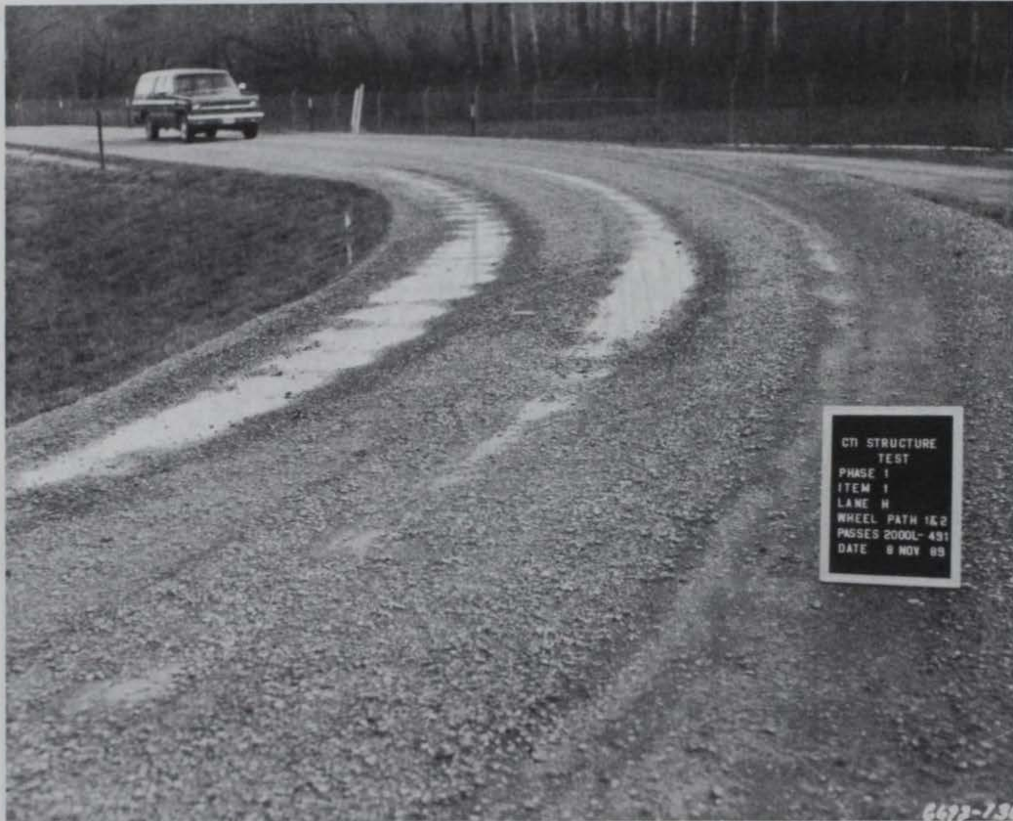
Photo 50. Item 1, high-pressure tire lane, low-severity rutting and washboarding at the end of traffic
