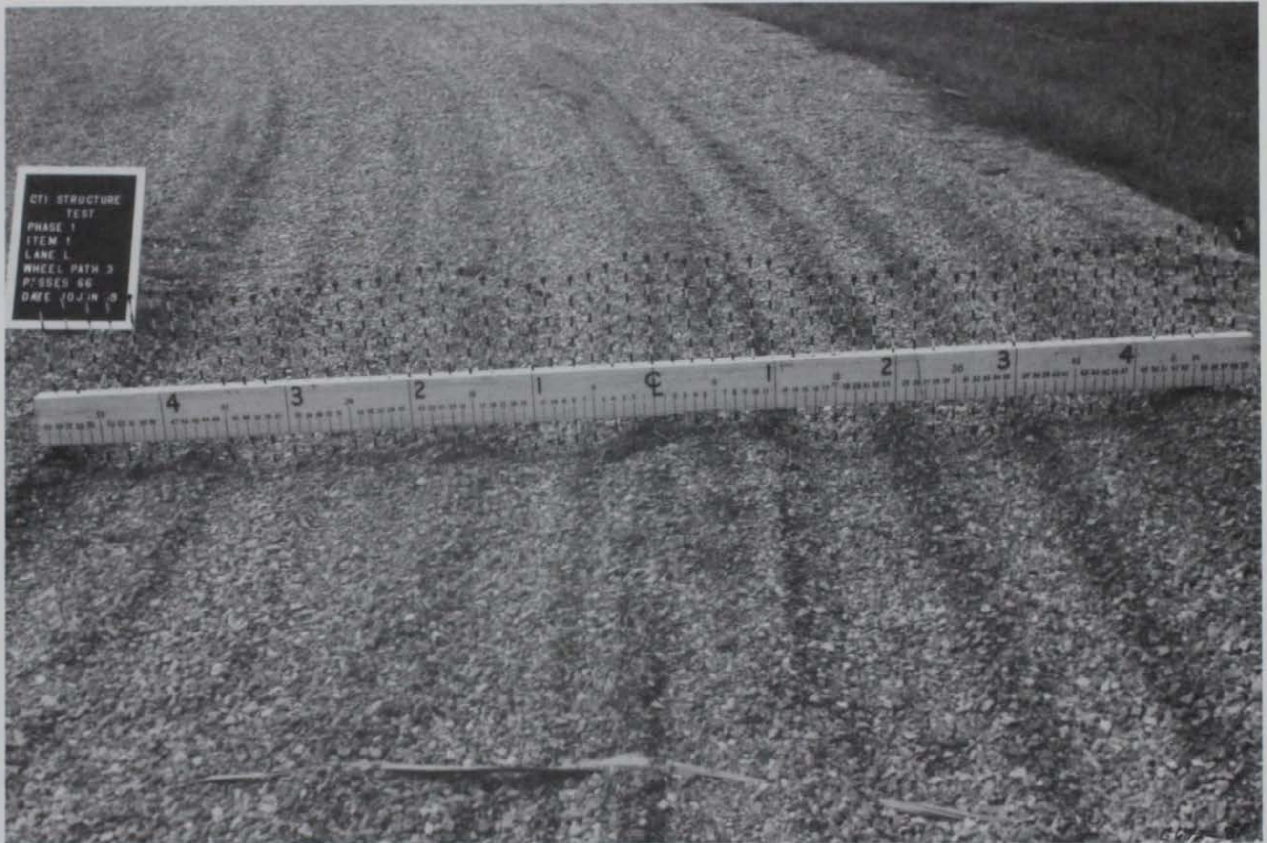
Photo 42. Item 1, low-pressure tire lane, failure after 66 passes
