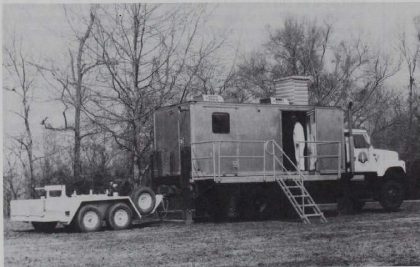
Figure 1. WES site characterization and analysis penetrometer system (SCAPS) truck
