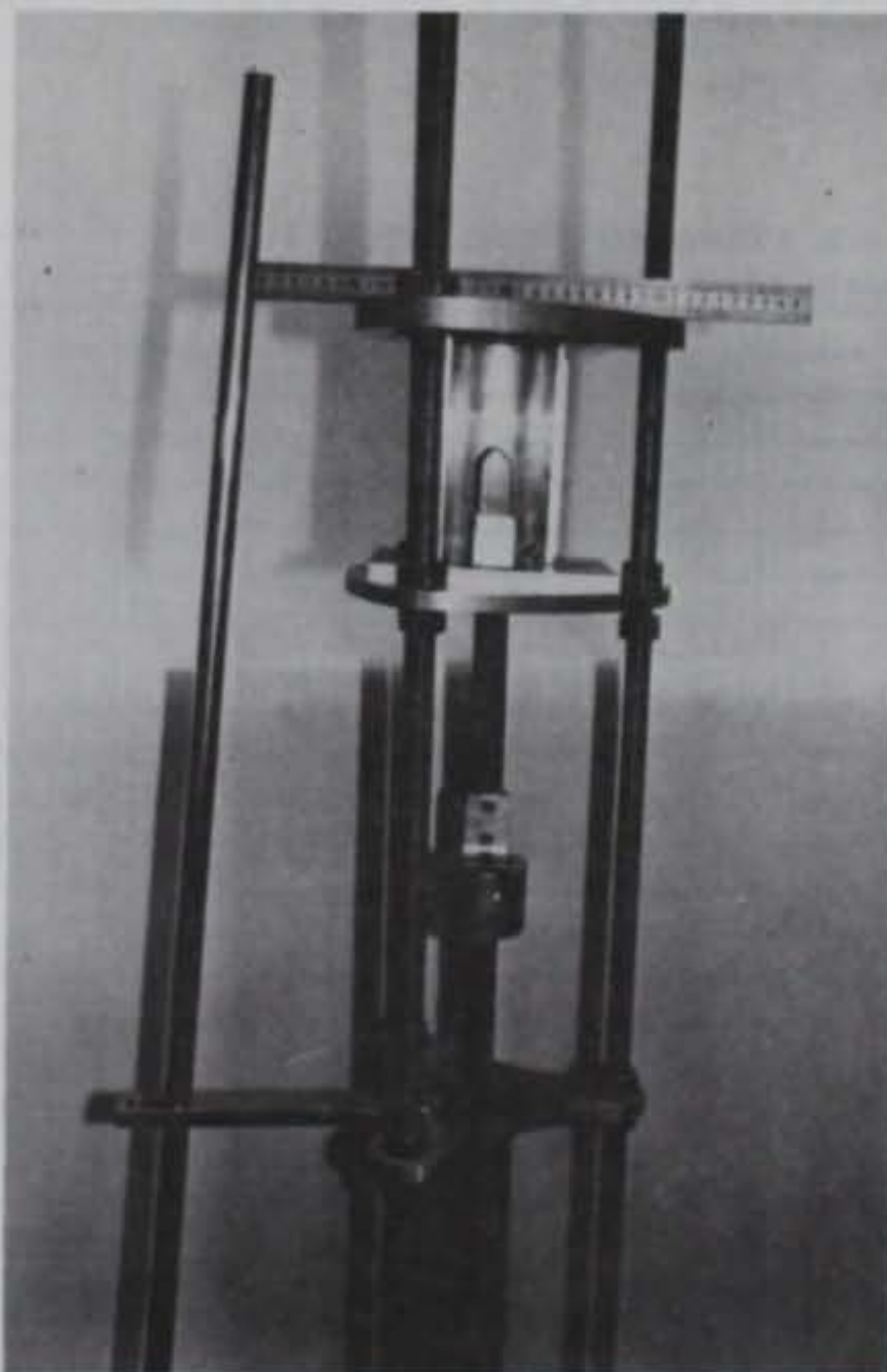
Fig. 5 Photographs of a) mold used to prepare reconstituted specimens showing the nozzle insert and b) specimen extruder modified to form a crack in the erosion specimen.
