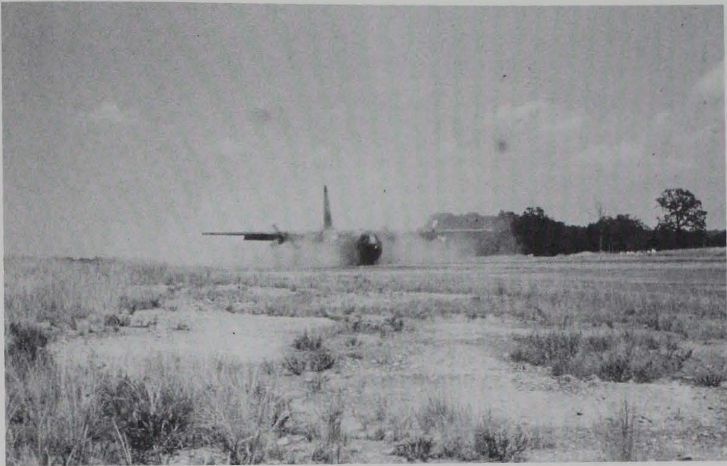
Figure 5. Dust engulfing C-130 aircraft landing on assault airstrip at Fort Chaffee
