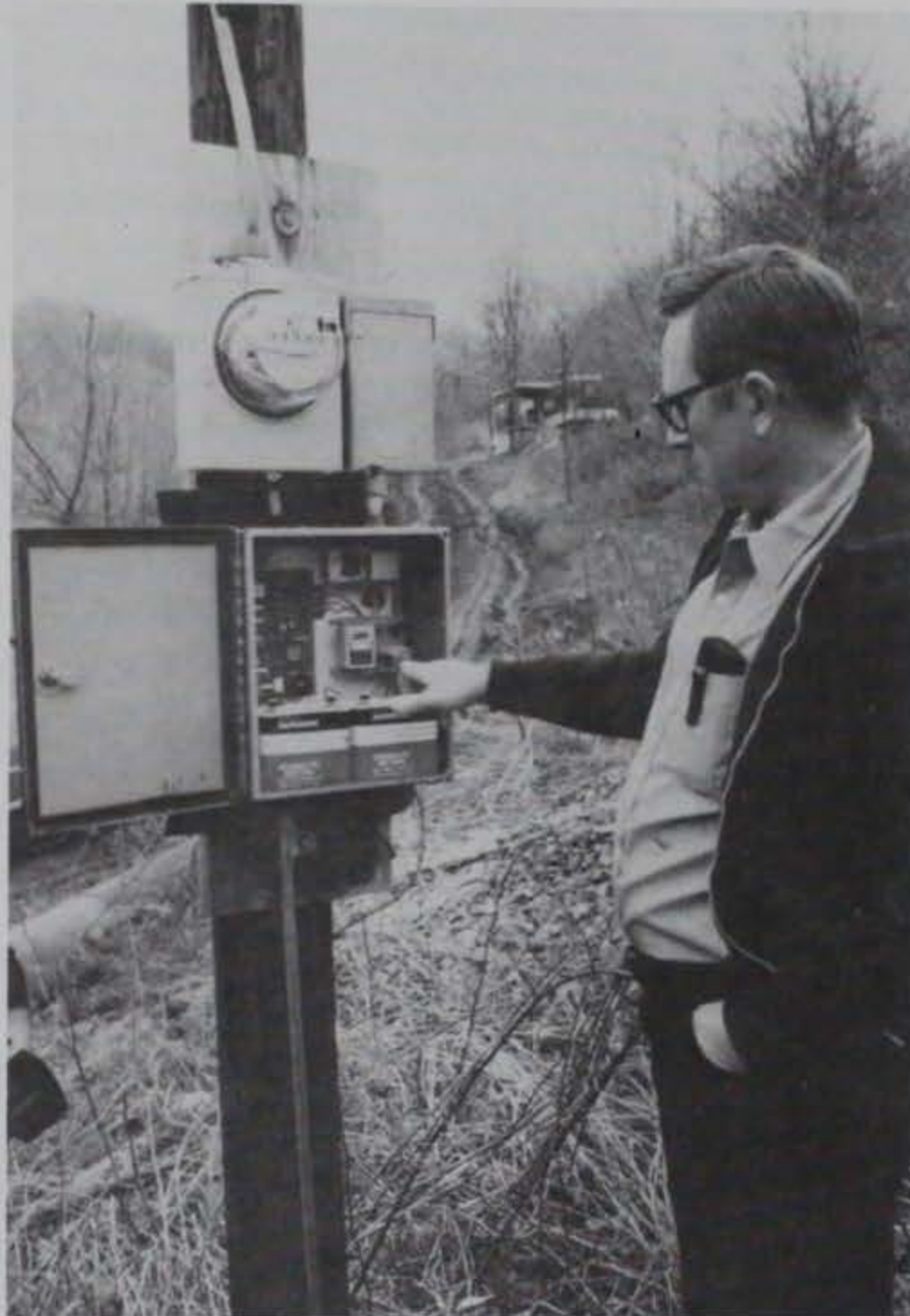
Figure 8. Signal-conditioning equipment used in the CONOCO seismic location system
