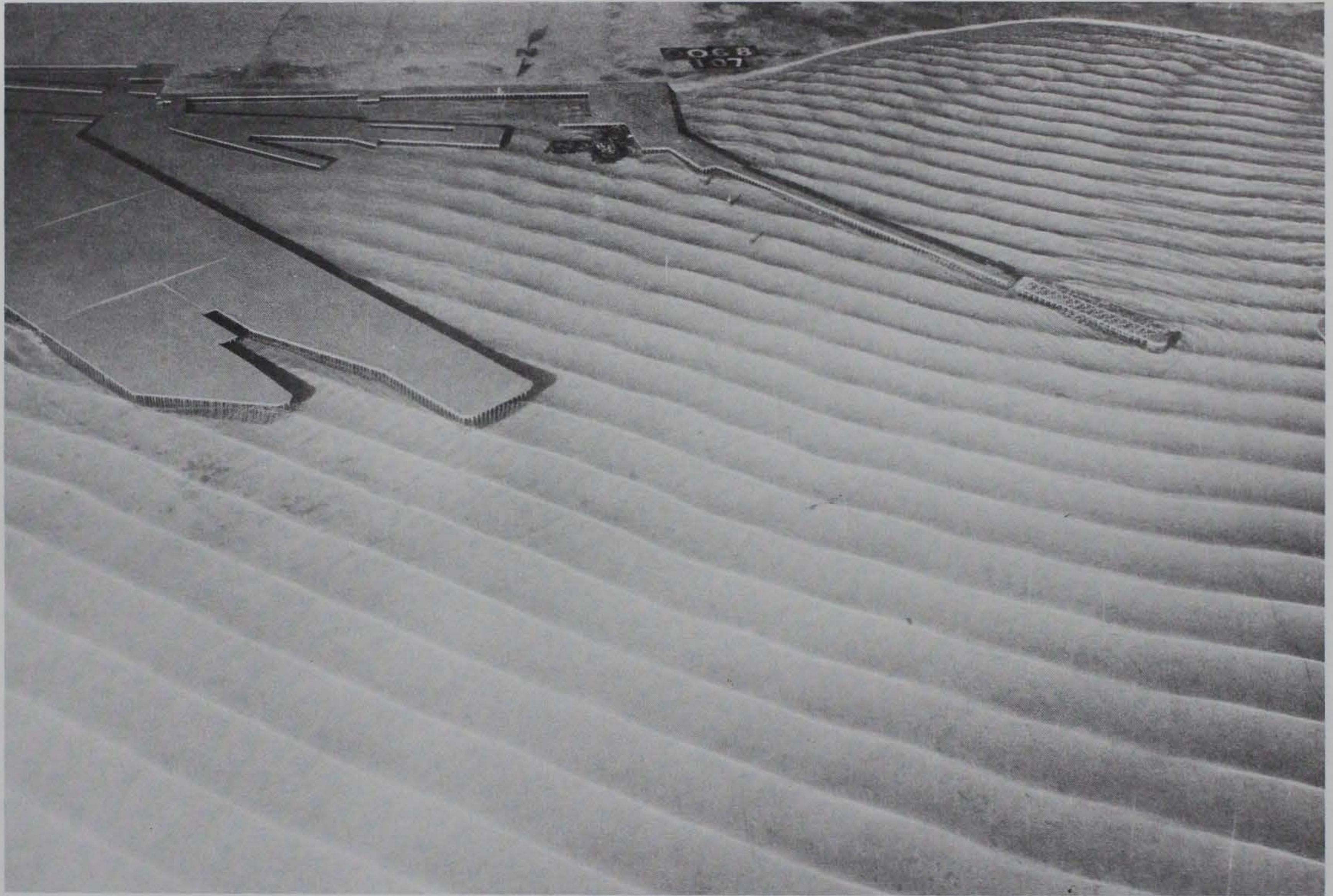
Photo 4. Typical wave patterns for existing conditions; 4.2-sec, 4.8-ft waves from north-northeast; +5.7 ft swl
