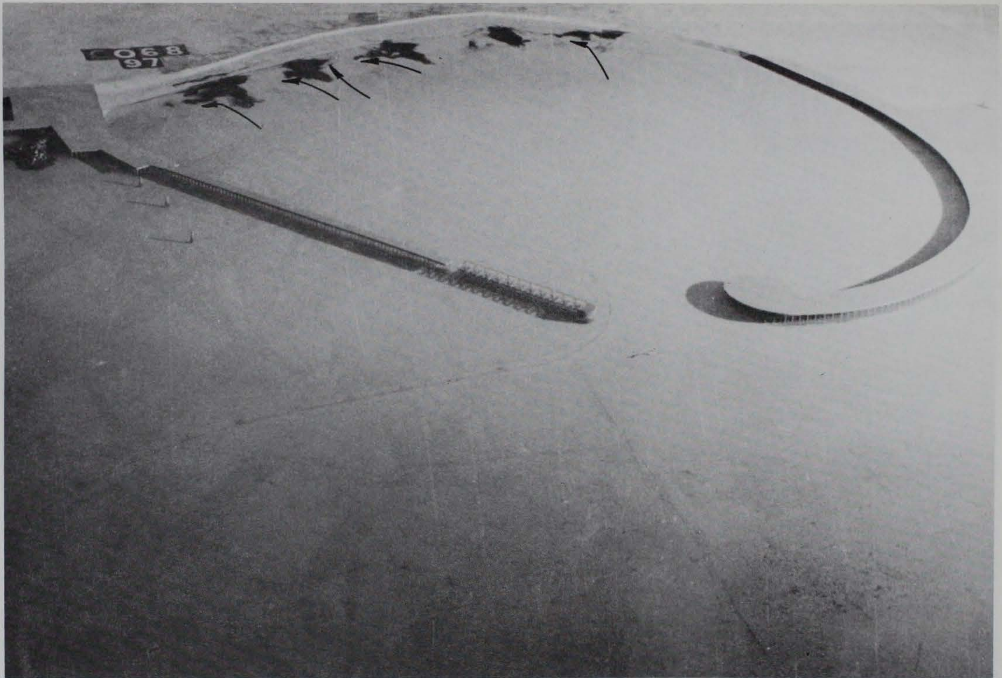
Photo 29. General movement of tracer material for existing conditions; 10-sec, 3-ft waves from west-northwest; 0.0-ft swl
