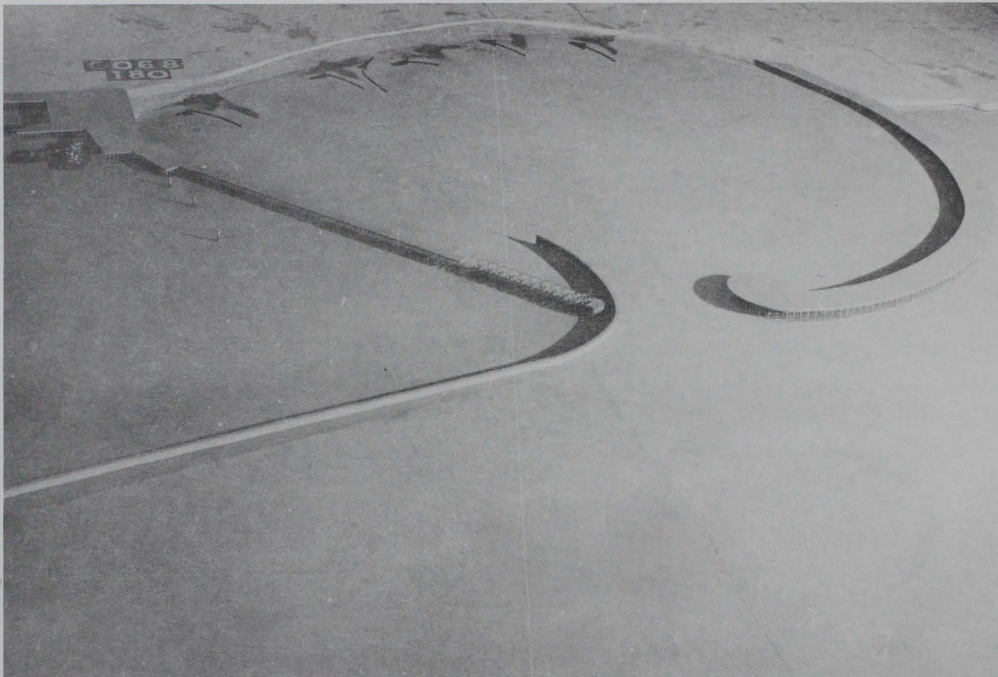
Photo 100. General movement of tracer material for Plan 38; 10-sec, 3-ft waves from west-northwest; 0.0-ft swl
