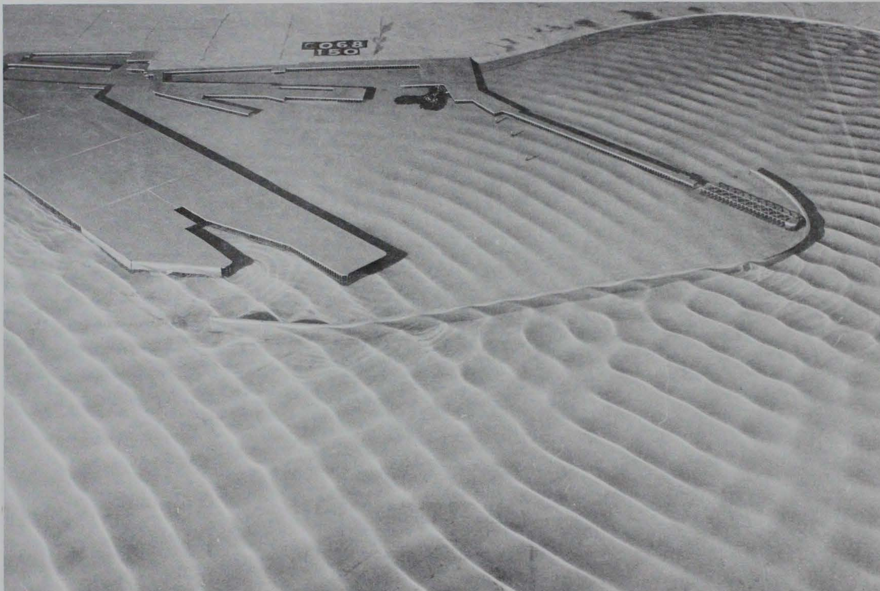
Photo 66. Typical wave patterns for Plan 34; 3.9-sec, 3.3-ft waves from northeast; +5.7 ft swl
