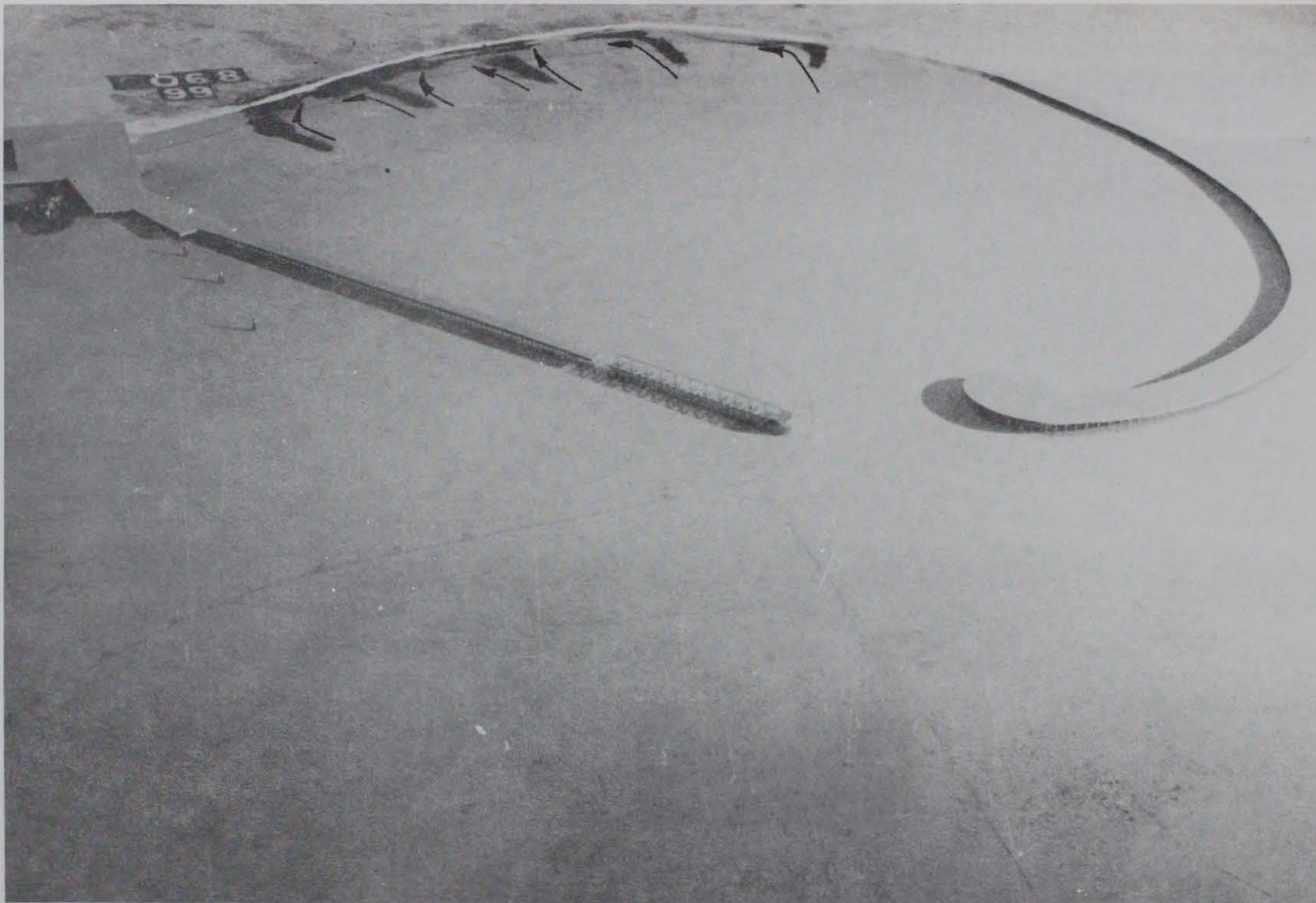
Photo 28. General movement of tracer material for existing conditions; 10-sec, 2-ft waves from west-northwest; +5.7 ft swl
