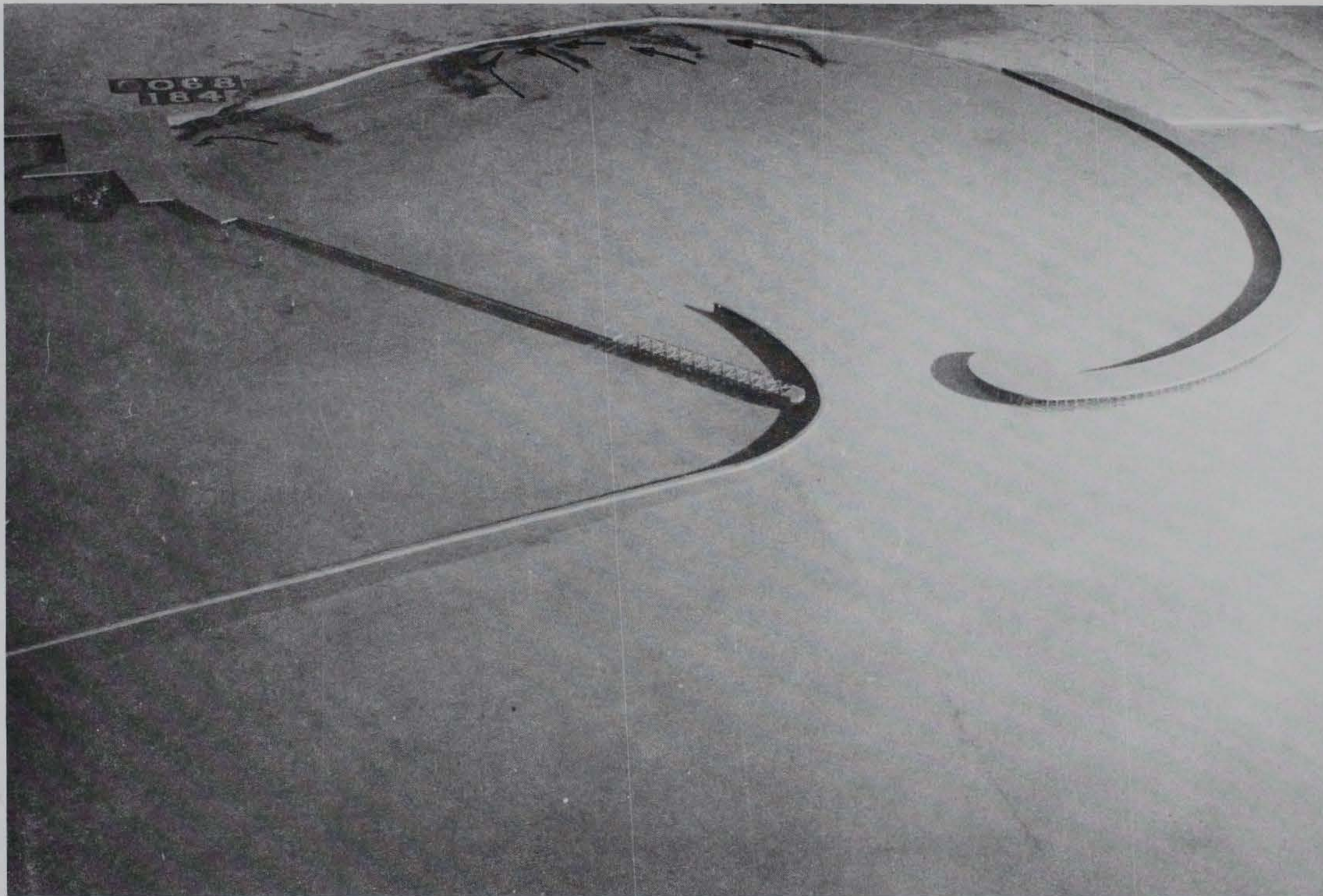
Photo 101. General movement of tracer material for Plan 38; 10-sec, 3-ft waves from west-northwest; +5.7 ft swl
