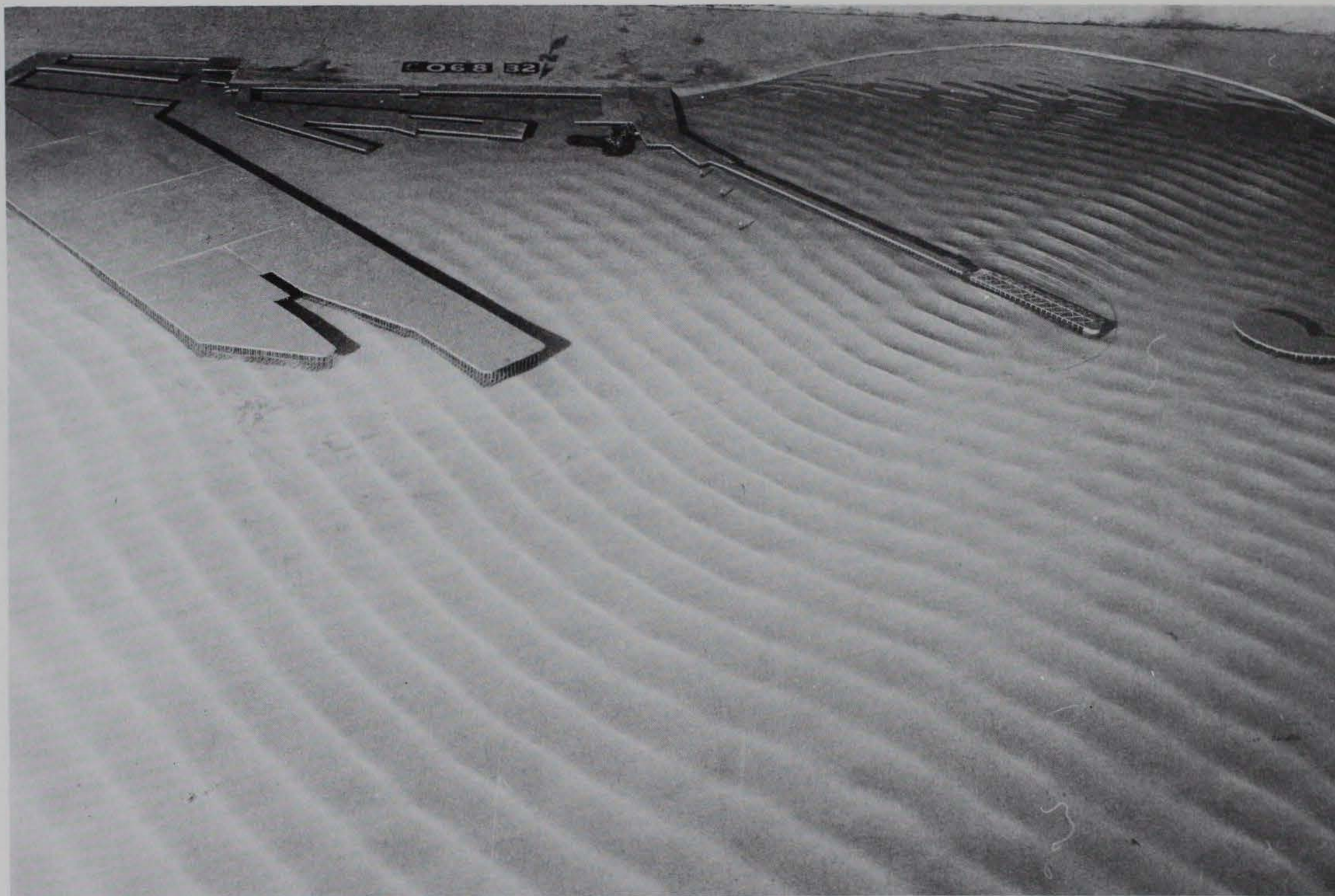
Photo 1. Typical wave patterns for existing conditions; 3.6-sec, 2-ft waves from northeast; +5.7 ft swl
