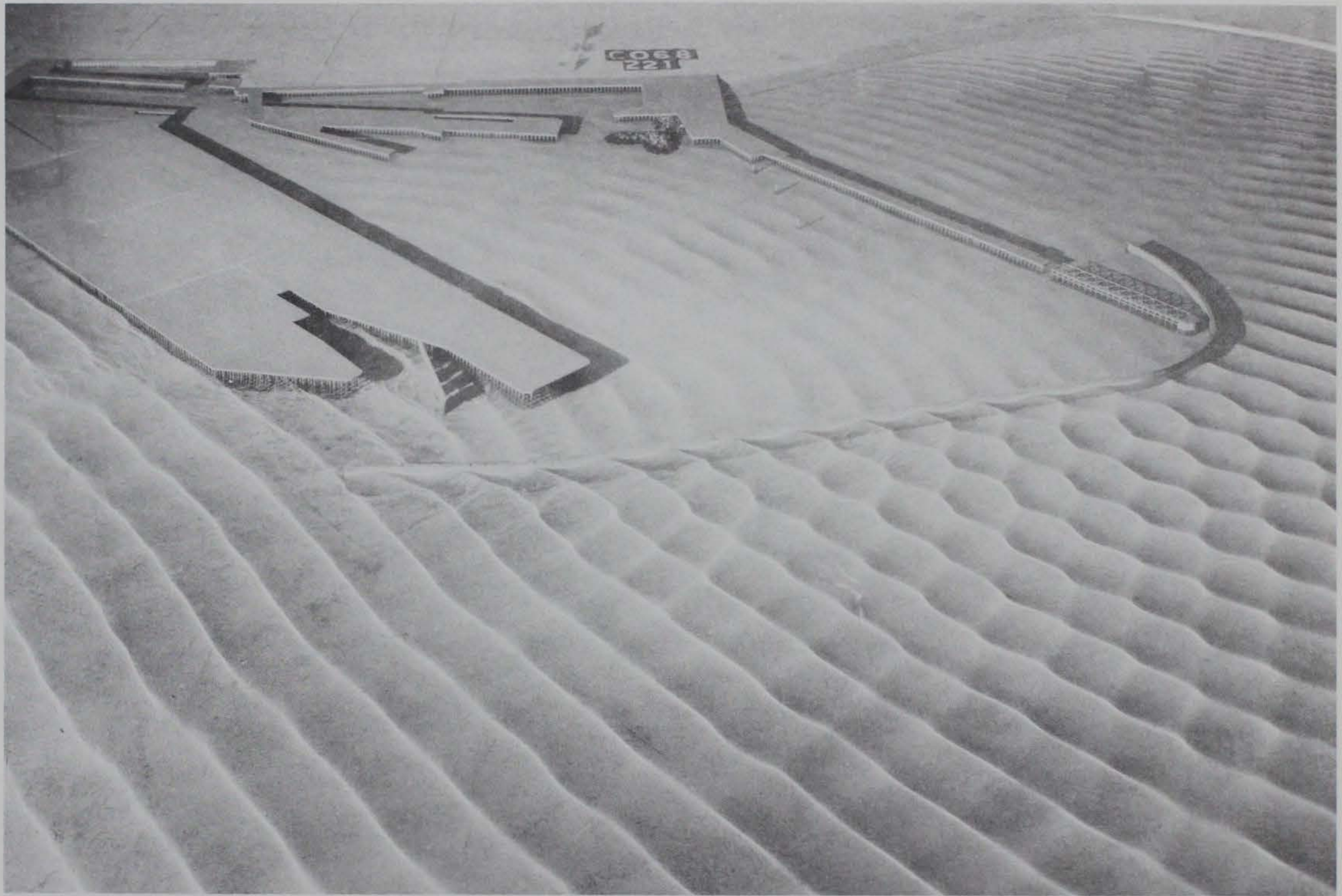
Photo 138. Typical wave patterns for Plan 78; 3.9-sec, 3.3-ft waves from northeast; 0.0-ft swl
