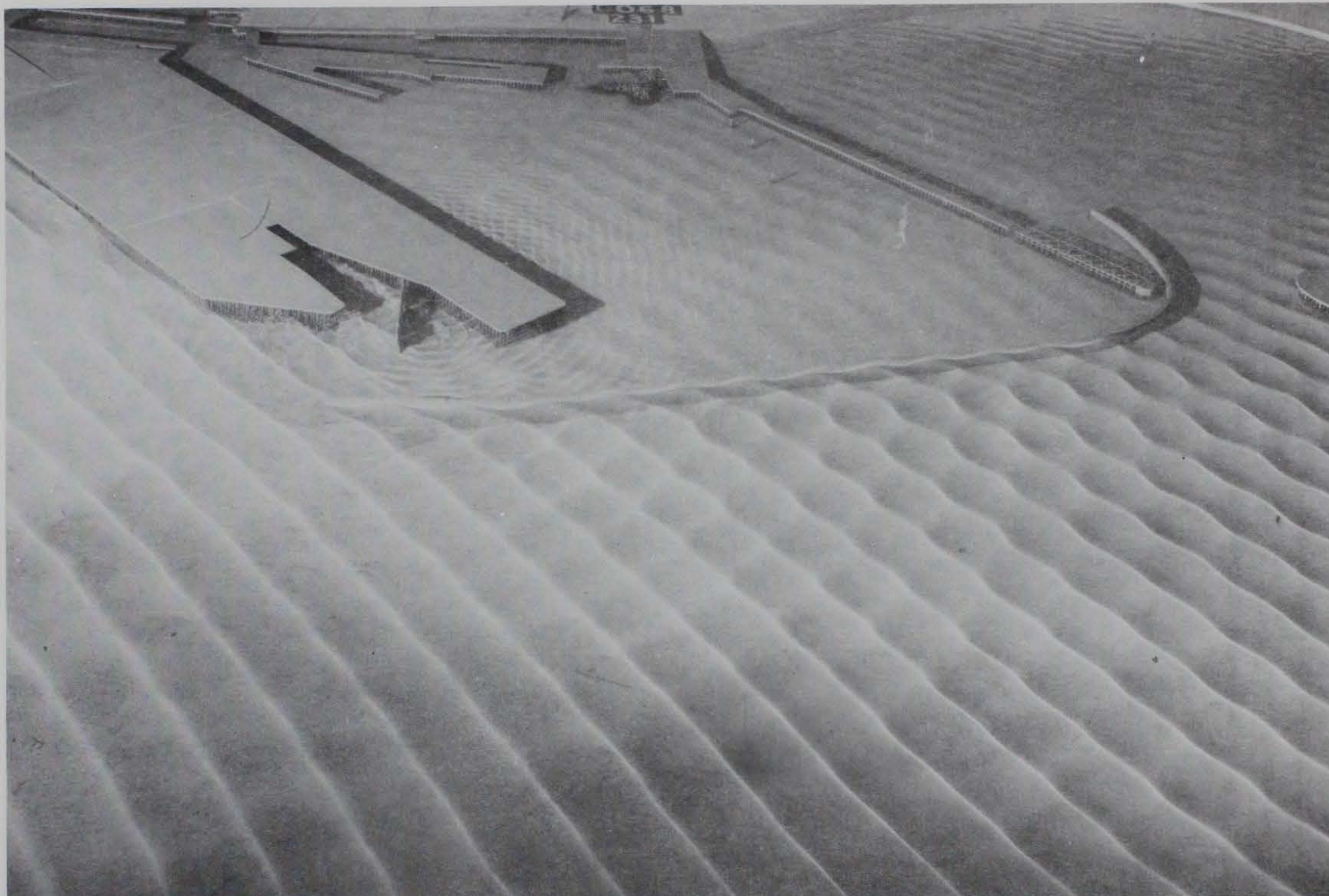
Photo 148. Typical wave patterns for Plan 88; 3.9-sec, 3.3-ft waves from northeast; 0.0-ft swl
