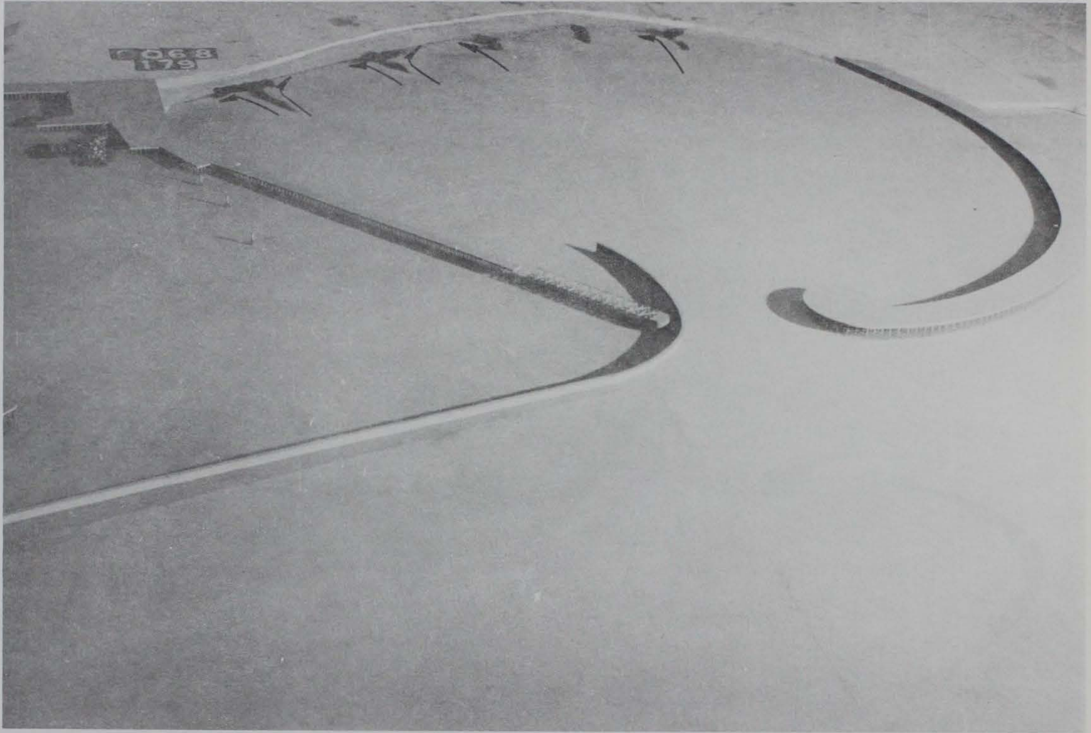
Photo 98. General movement of tracer material for Plan 38; 10-sec, 2-ft waves from west-northwest; 0.0-ft swl
