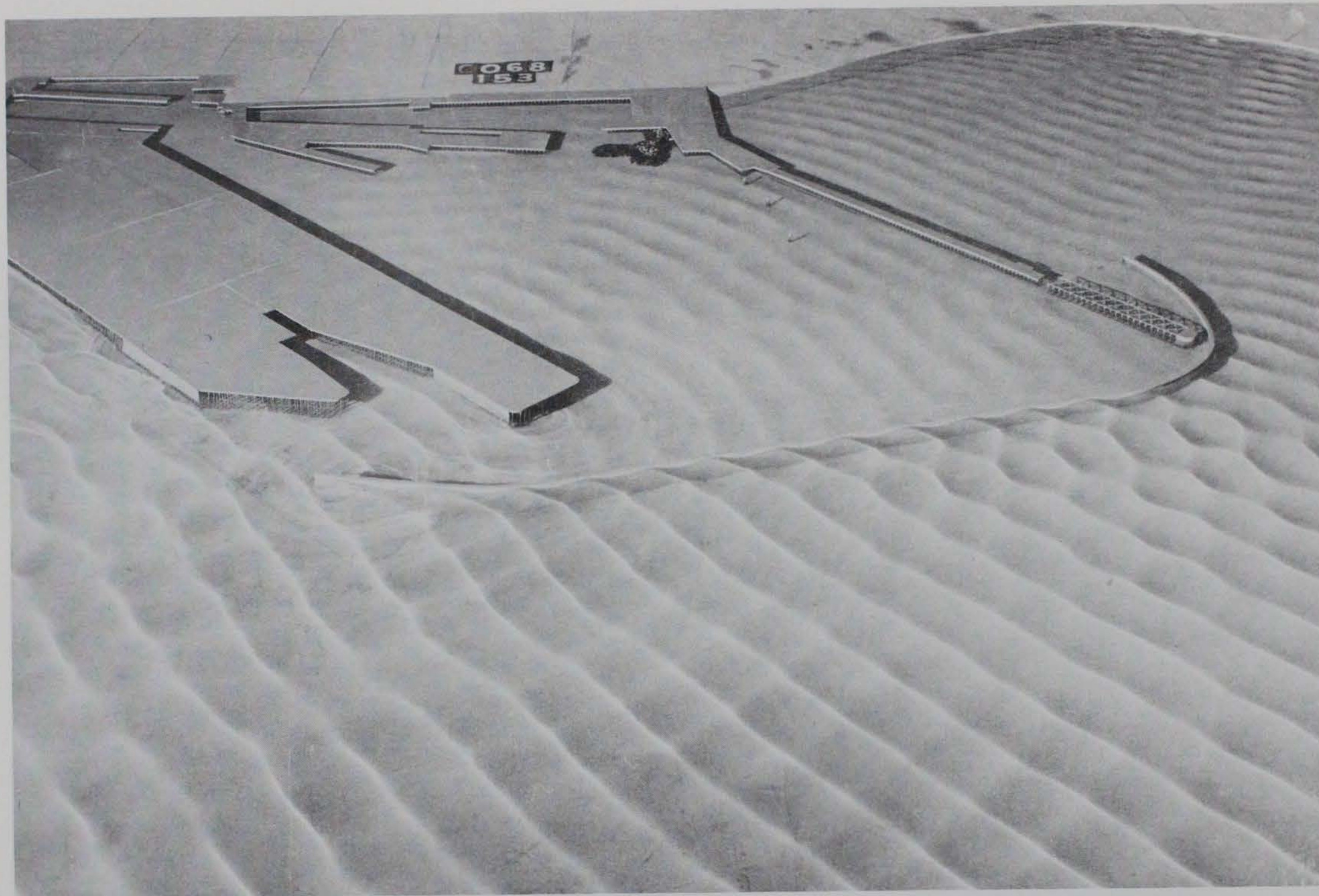
Photo 68. Typical wave patterns for Plan 36; 3.9-sec, 3.3-ft waves from northeast; +5.7 ft swl
