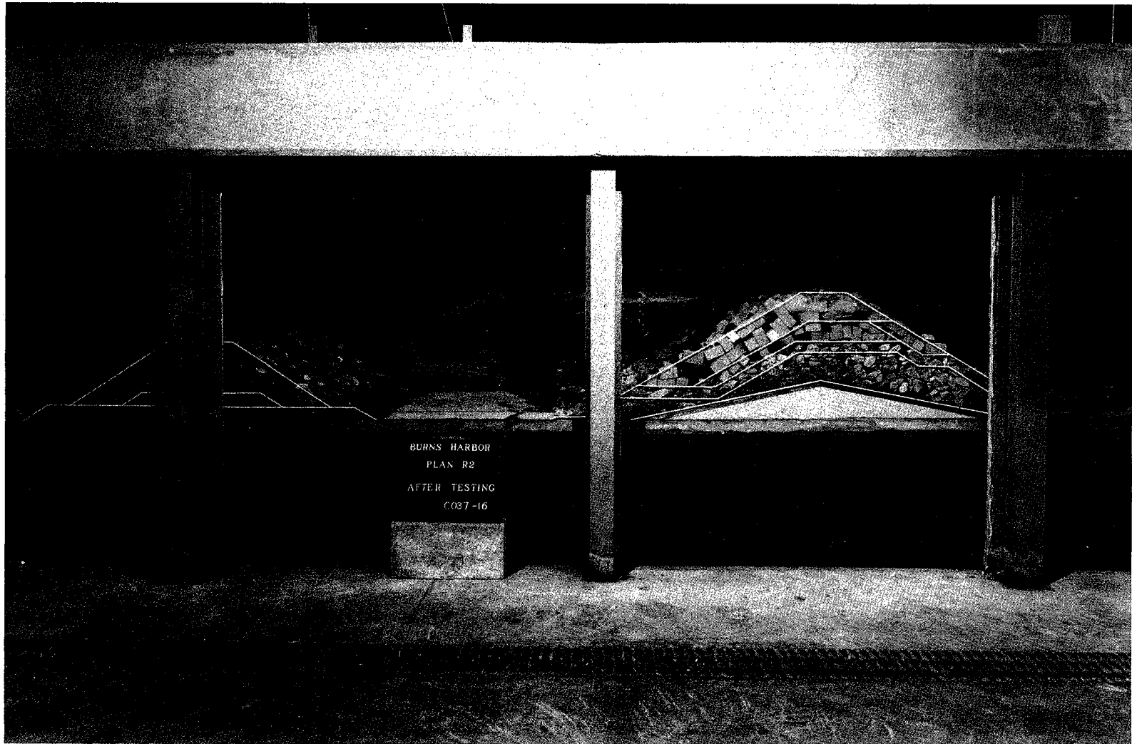
Photo 6. End view of Plan R2 (reef and existing breakwater) after wave attack
