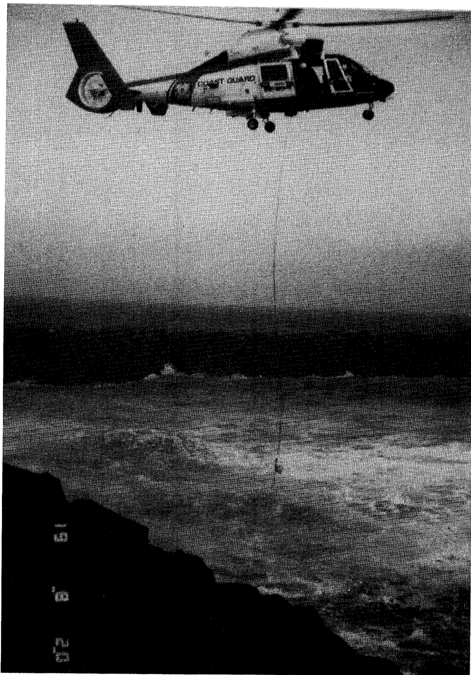
Figure 19. Airborne Coastal Current Measurement System in operation near structure
