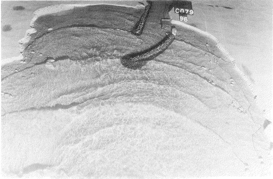
Photo 25. Typical wave patterns for Plan 43; 17-sec, 20-ft waves from west; swl = +7.0 ft
