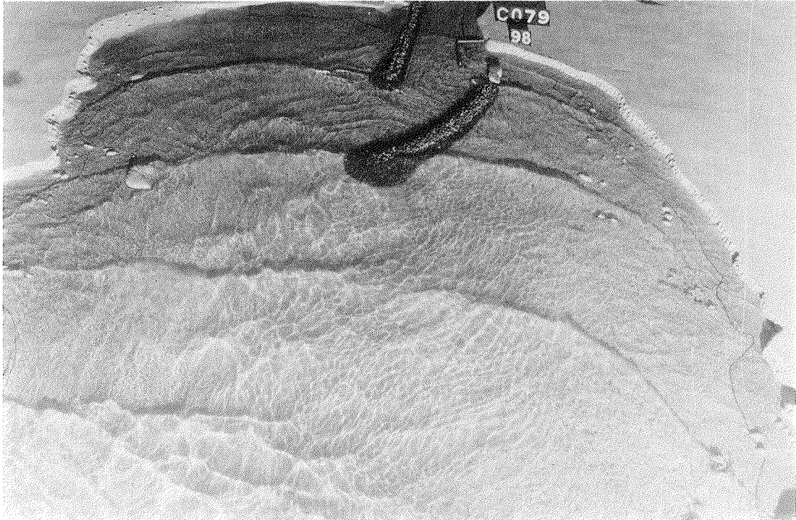
Photo 21. Typical wave patterns for Plan 43; 17-sec, 22-ft waves from northwest; swl = +7.0 ft
