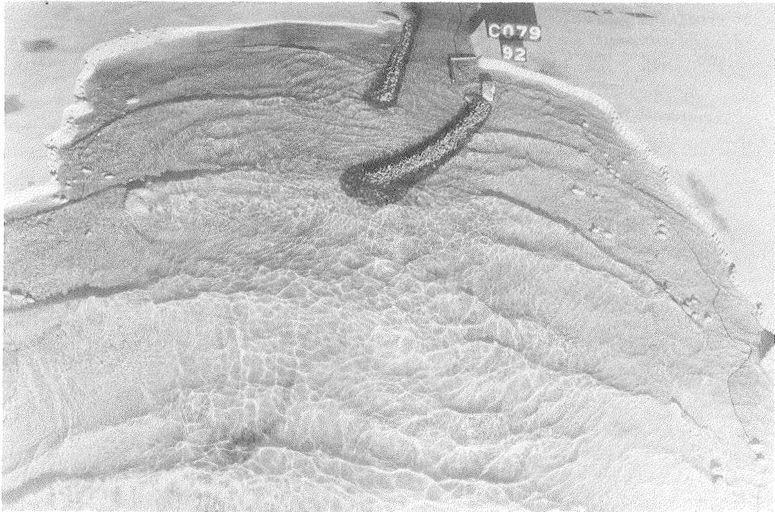
Photo 29. Typical wave patterns for Plan 43; 15-sec, 32-ft waves from southwest; swl = +7.0 ft
