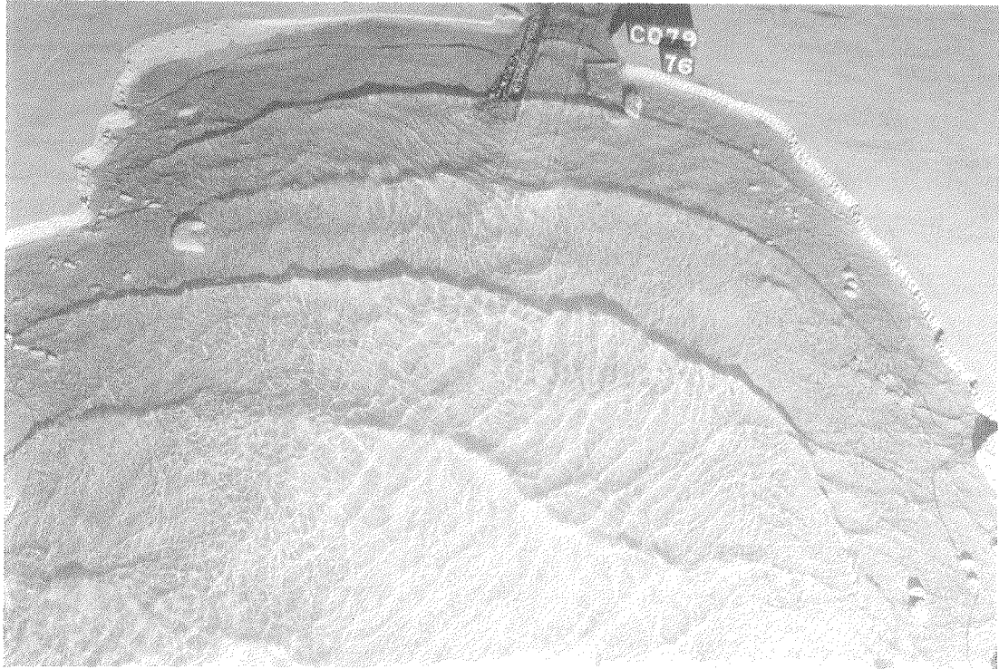
Photo 15. Typical wave patterns for Plan 2; 13-sec, 22-ft waves from west-northwest; swl = +6.2 ft
