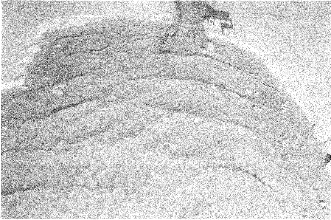
Photo 3. Typical wave patterns for existing conditions; 11-sec, 12-ft waves from west; swl = +6.2 ft
