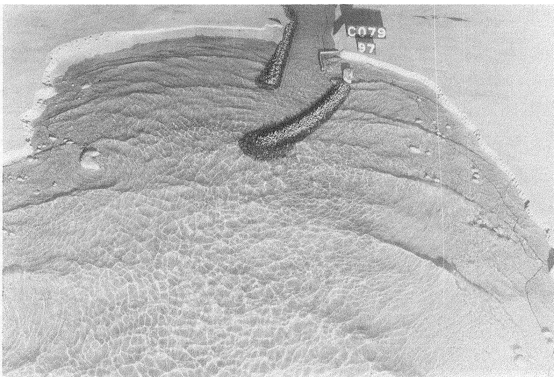
Photo 20. Typical wave patterns for Plan 43; 13-sec, 12-ft waves from northwest; swl = +7.0 ft
