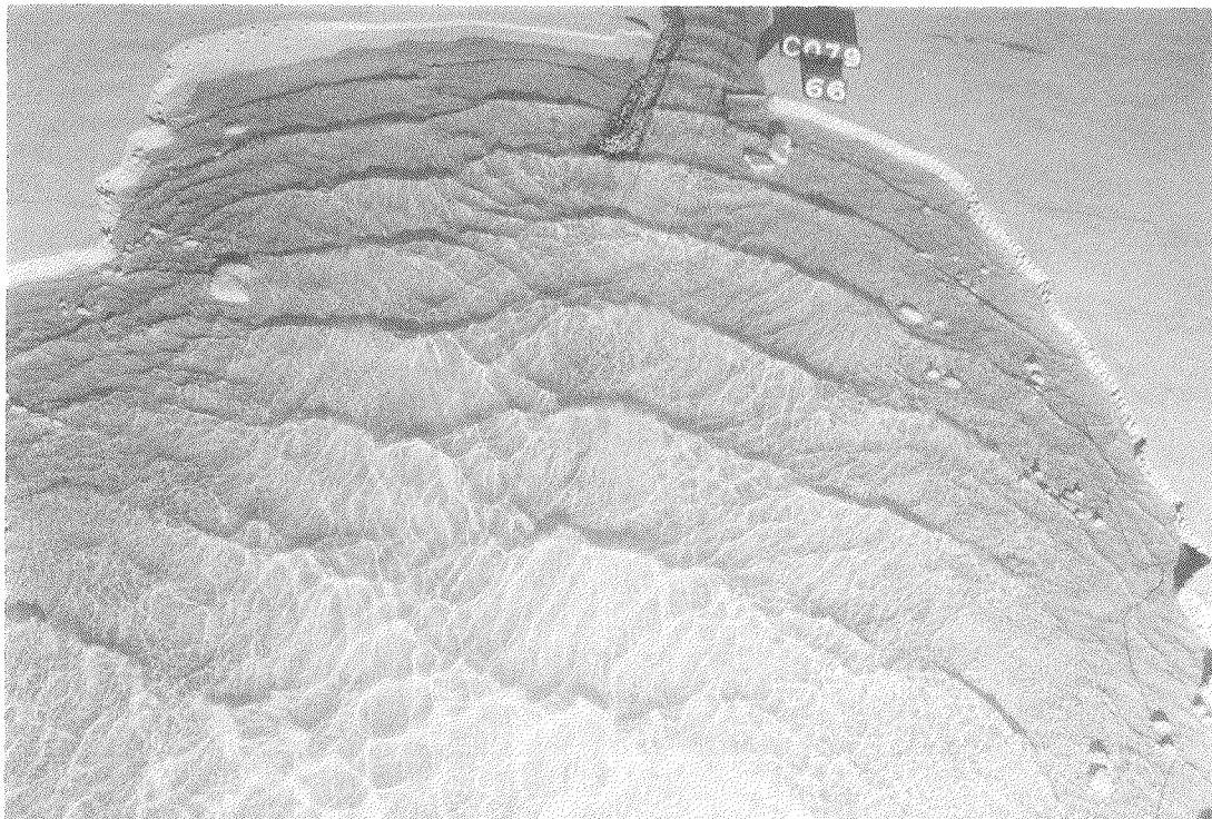
Photo 14. Typical wave patterns for Plan 2; 9-sec, 20-ft waves from northwest; swl = +6.2 ft
