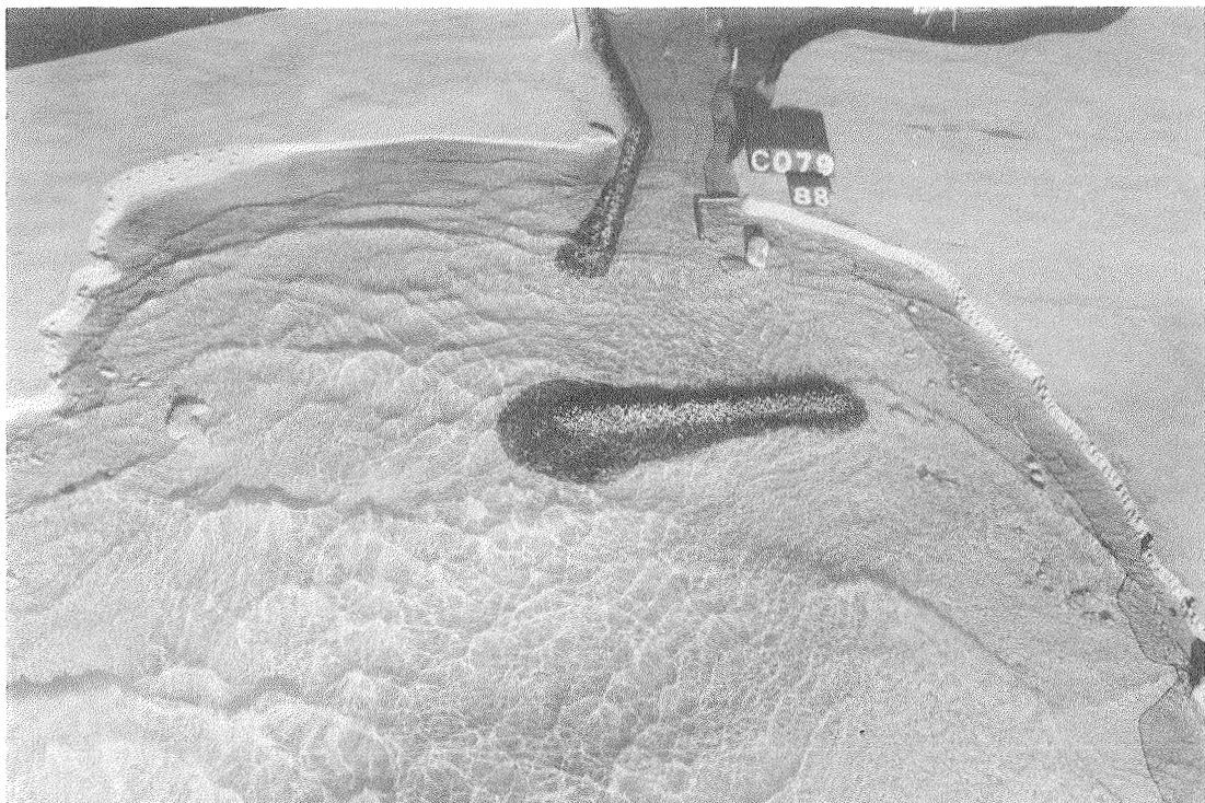
Photo 18. Typical wave patterns for Plan 3A; 17-sec, 20-ft waves from west-northwest; swl = +7.0 ft
