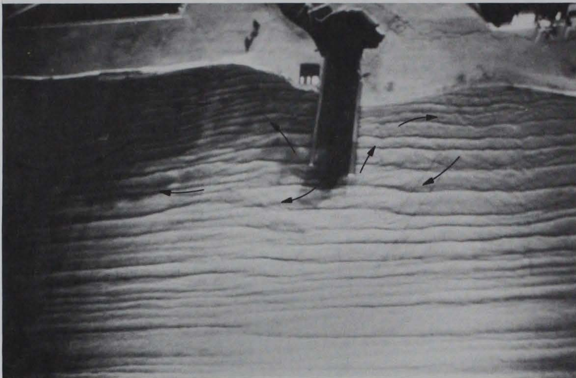
Photo 11. Current patterns and movement of creek plume for existing conditions for test waves from 343 deg during fall conditions
