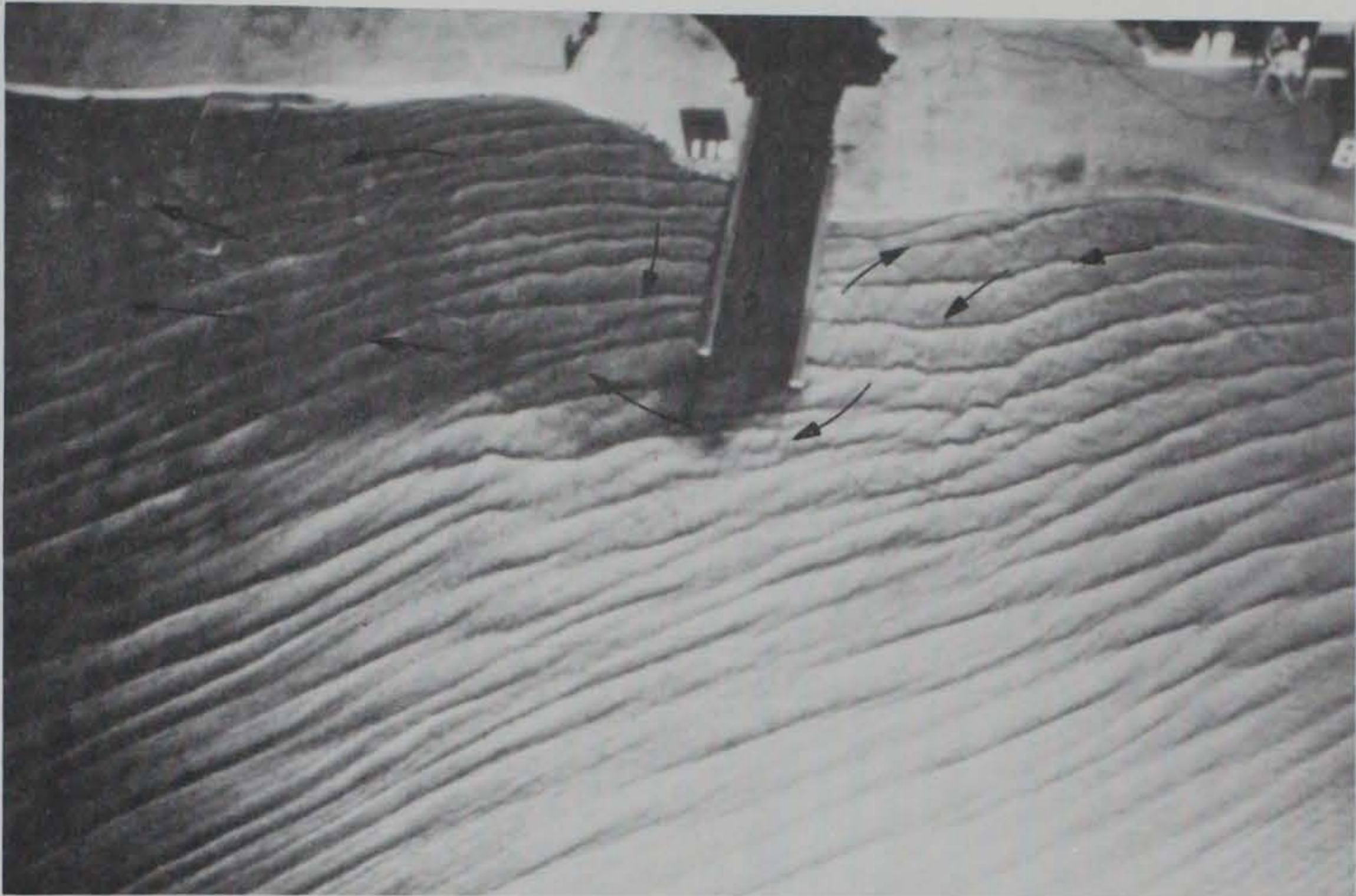
Photo 13. Current patterns and movement of creek plume for existing conditions for test waves from 313 deg during fall conditions
