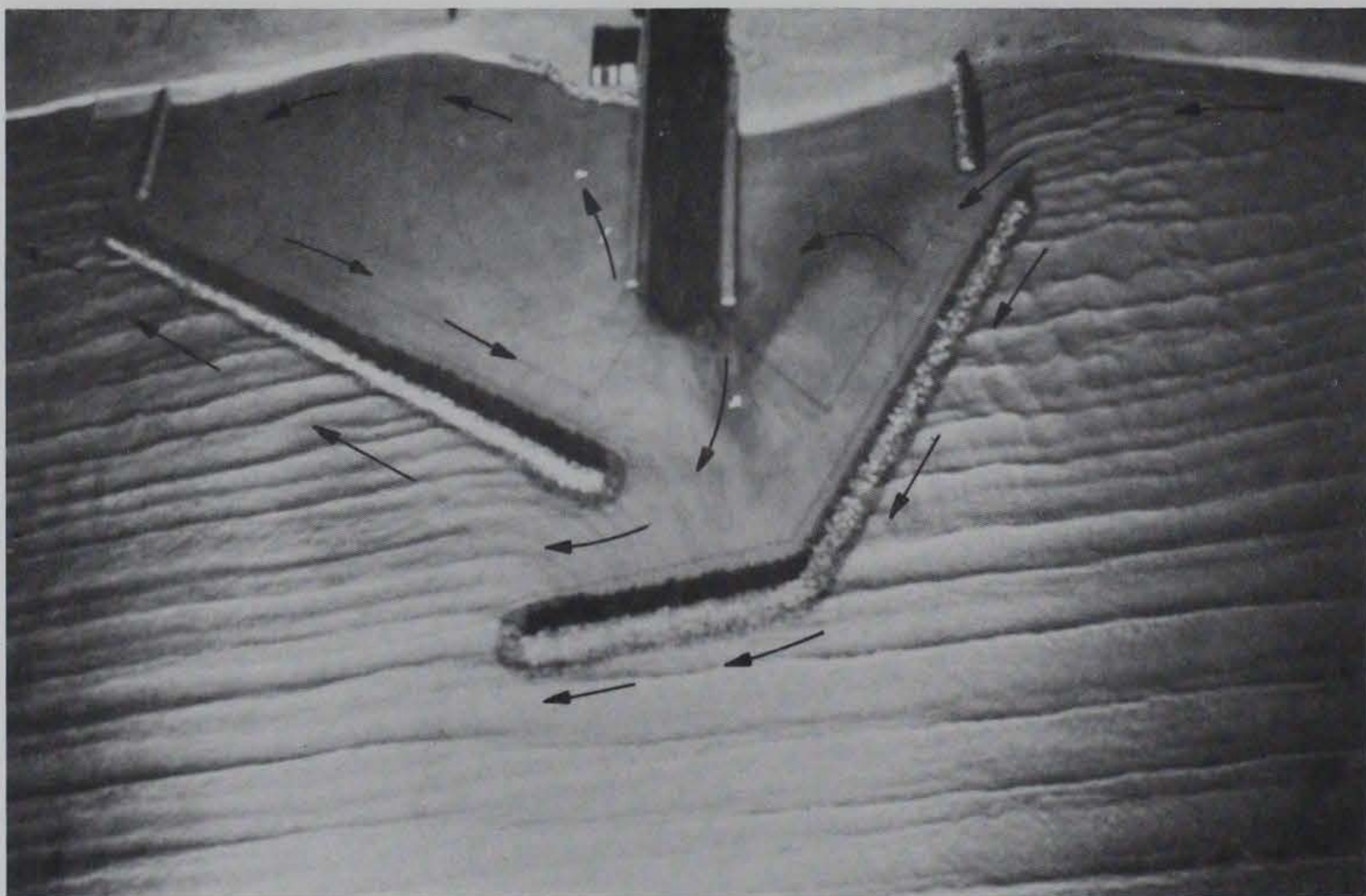
Photo 12. Current patterns and movement of creek plume for Plan 19 for test waves from 343 deg during fall conditions
