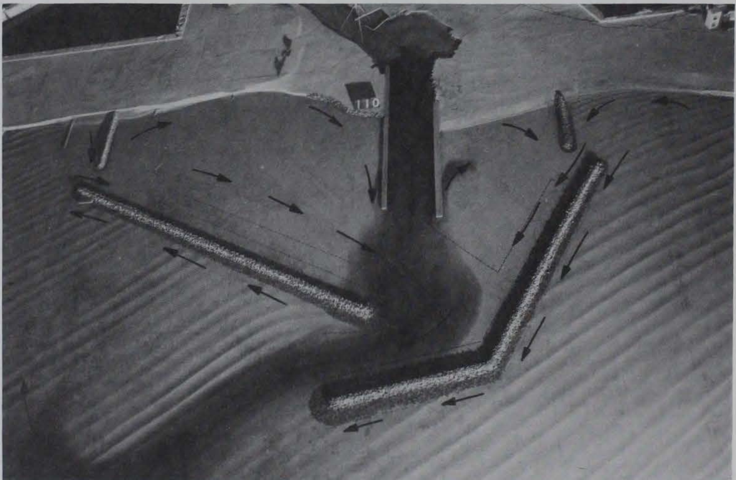
Photo 8. Current patterns and movement of creek plume for Plan 19 for test waves from 313 deg during spring conditions
