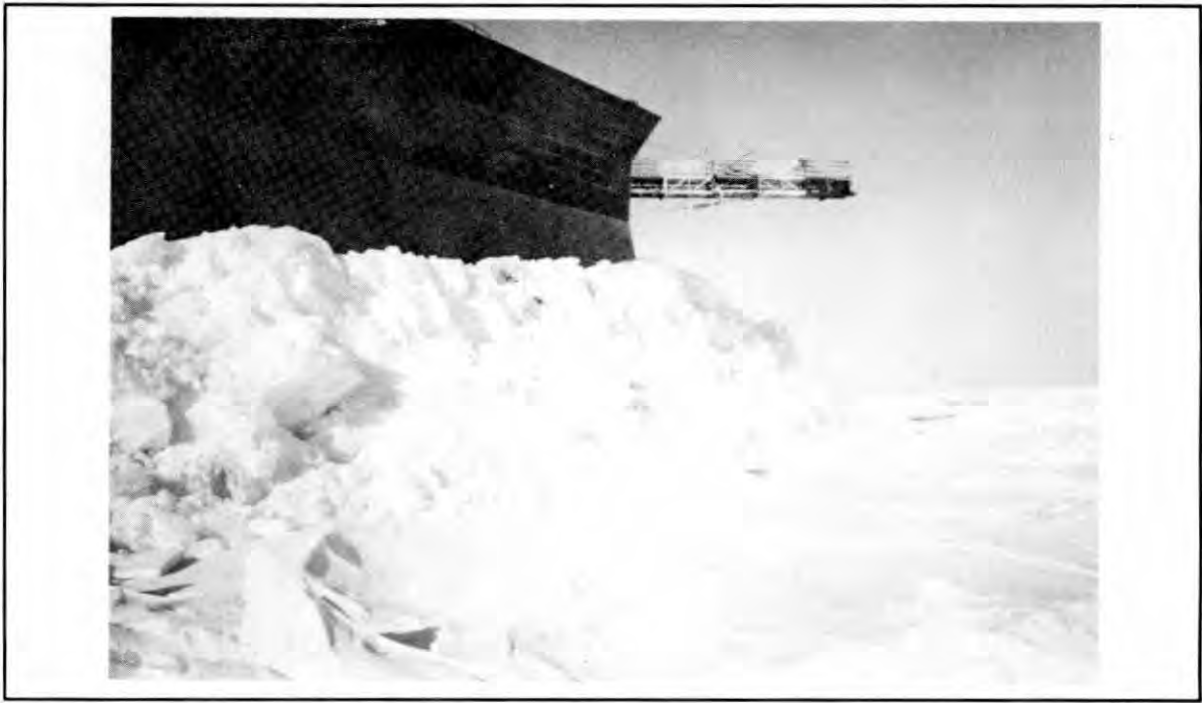
PLATE 12. SIDE VIEW OF THE FAILURE BY CRUSHING OF A COLD MULTI-YEAR ICE FLOE ON THE MOLIKPAQ IN 1986. THE ICE THICKNESS WAS ABOUT 4 M AND THE PENETRATION RATE .01 M/S. COURTESY OF B. WRIGHT, GULF CANADA CORPORATION.
