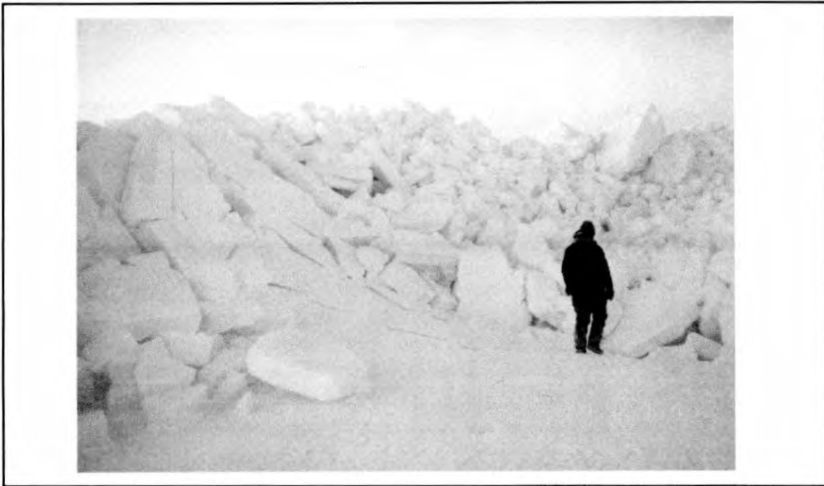
PLATE 6. BENDING FAILURE OF AN ICE SHEET AGAINST AN EXISTING RIDGE WHICH RESULTED IN RIDE-UP. THE FIRST-YEAR ICE SHEET WAS ABOUT 0.4 M THICK AND THE WIDTH OF THE BENT ZONE WAS 20 M. COURTESY OF CANMAR.
