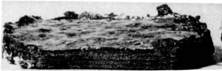
Figure 10. Closeup of Level D membrane sample taken from a blister.
