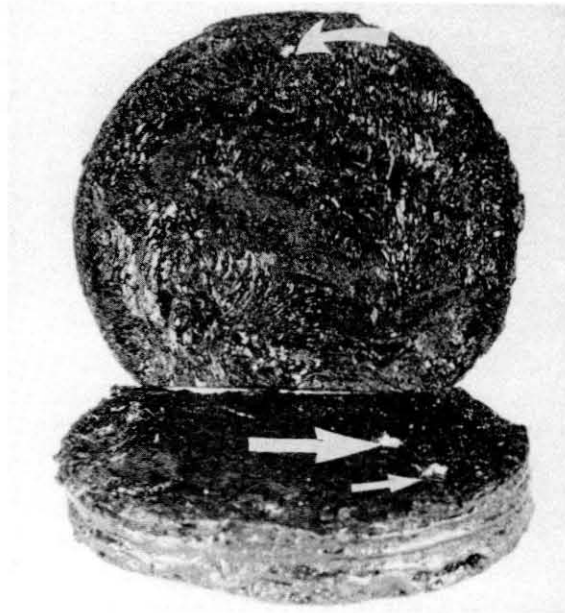
Figure 11. Particles of urethane insulation (arrows) entrapped within the plies of this membrane sample.
