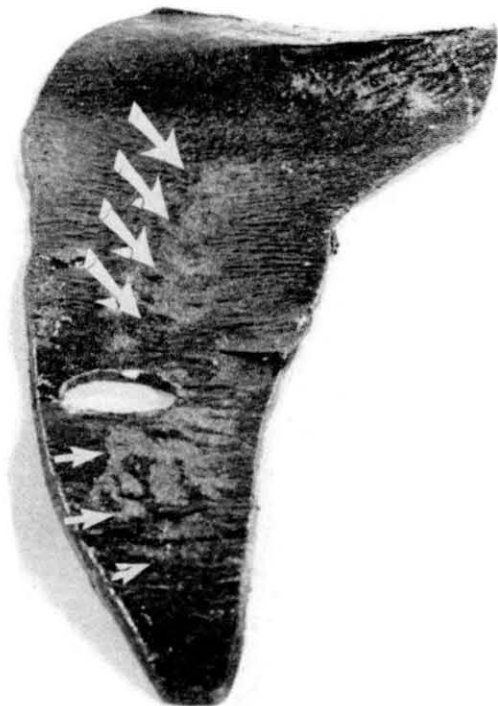
Figure 12. Arrows point to areas with insufficient bitumen coating. (A 2-in.-diameter sample was removed.)
