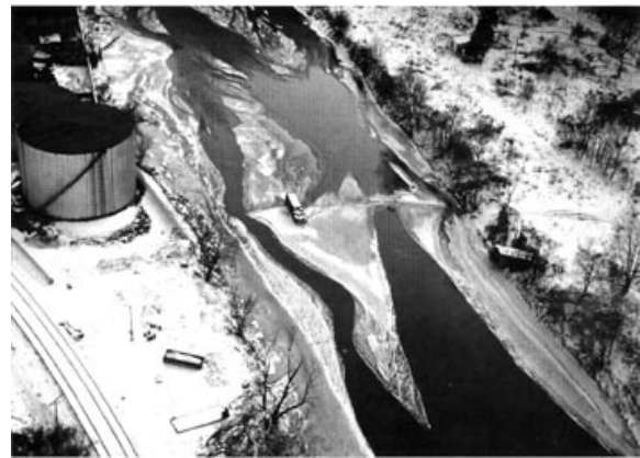
Figure 3. Funnel-shaped ice formation at Oil Creek, Pennsylvania.
