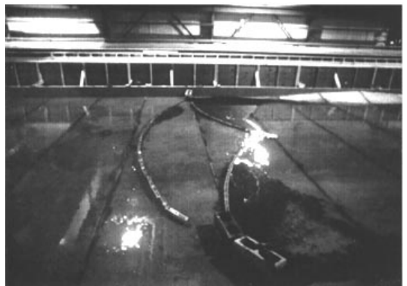
c. Sag and shear ice booms during testing.
