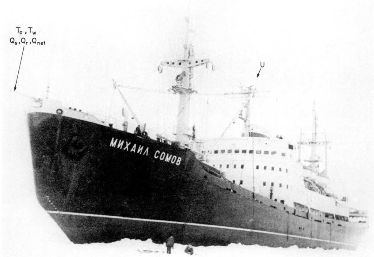
Fig. 2. Locations of sensors on the Somov .
