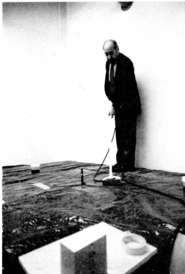
Figure 19. Model 3100 antenna, attached to a rod, is being swept across the path of the surveyor. Scan data for this operation appear in Figure B5.
