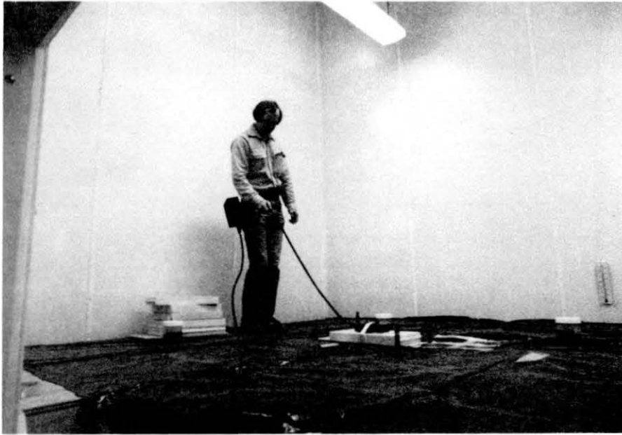
Figure 18. Model 3100 antenna being pulled across the test box at a fixed height above the surface. Scan data for these tests appear in Figures B1-B4.
