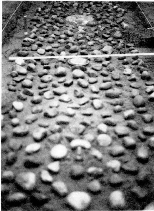
Figure 9. Location of stones in the box with RAAM mine in the center.
