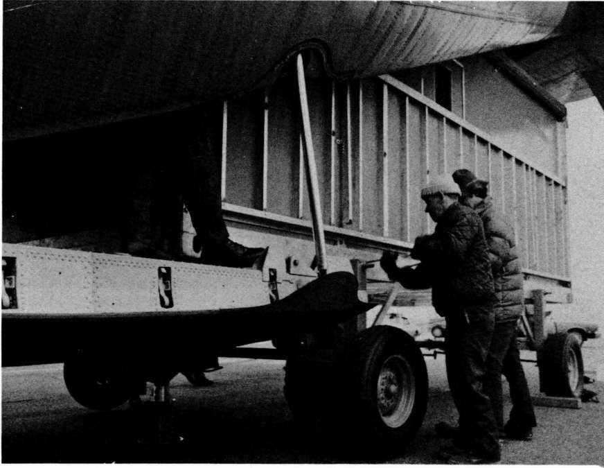
Figure 1.2.1. The shelter in shipping configuration being loaded into a USAF C-130. Legs mount wheels or skis to permit mobility to and from nearby sites. These legs are removed for transport.
