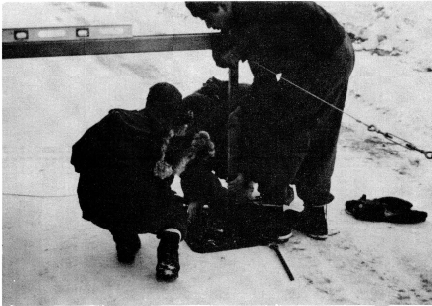
Figure 3.4.3. The expansion beam jacks should be about 1/2 in. above level or more to allow for settlement of the bearing surface.
