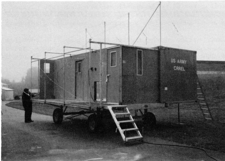
Figure 1.2.2. The expanded shelter. Roof, sidewall, and end walls roll back to the left as a rigid structural unit. The porch swings down to reveal the front door and engine compartment access (behind the step ladder). A frame supports the tent.
