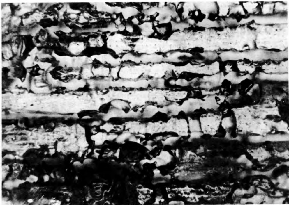
Figure 15. Photomicrograph of sea ice at a temperature only slightly below the freezing temperature (-3C, Thule, Greenland).
