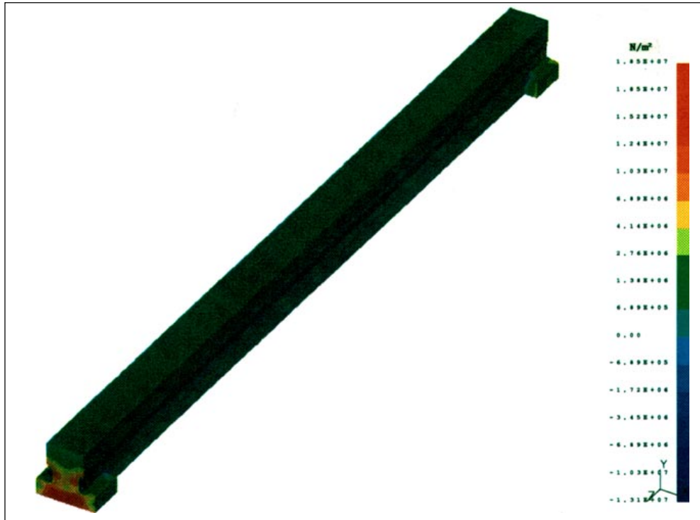
Figure 17. Maximum principal stress contours for Bechtel girder.
