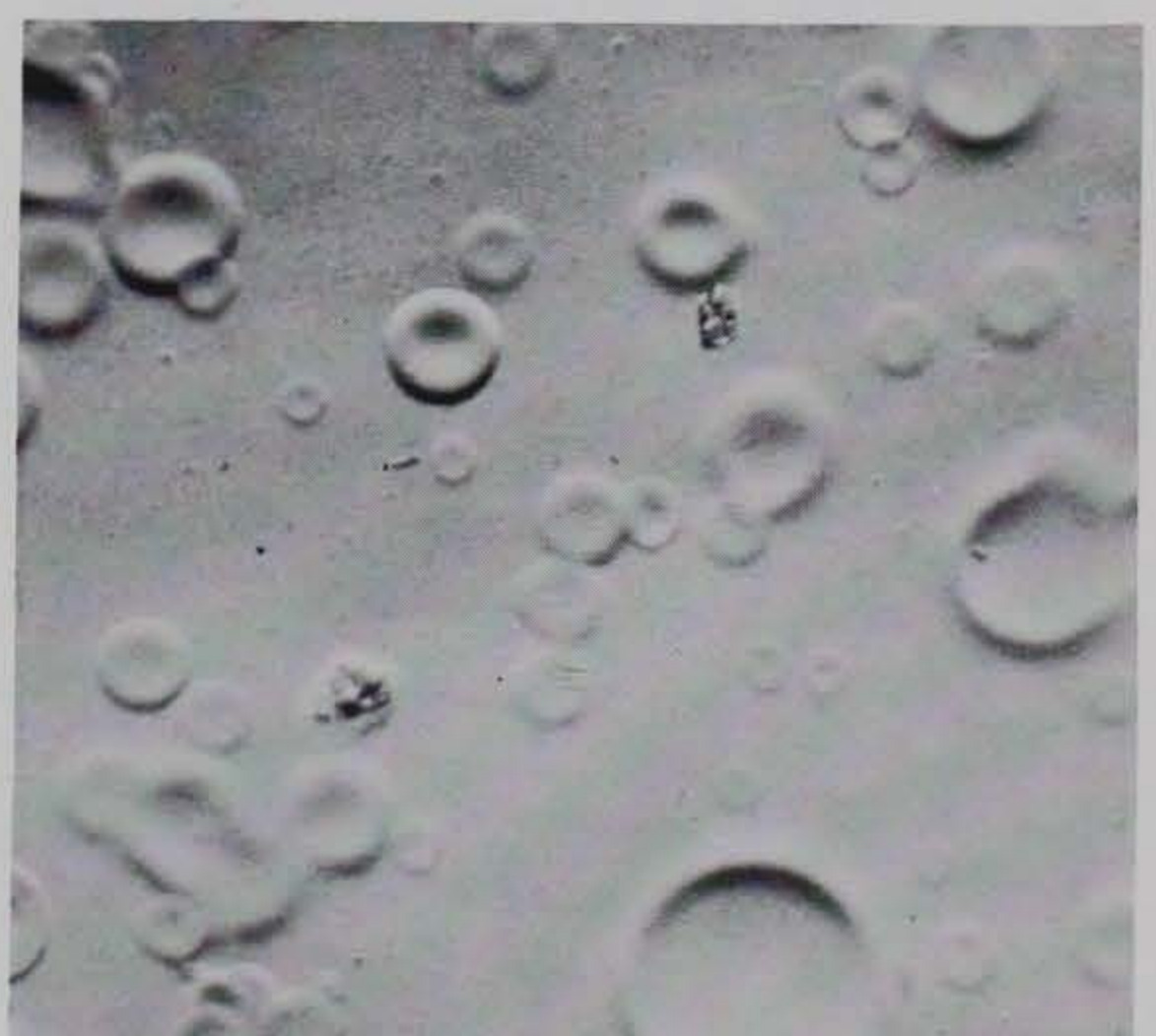
Figure 3. Fog drop prints on chloride-sensitive gelatin-coated glass slides.
