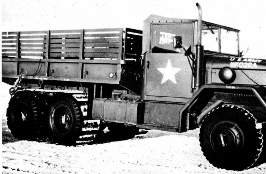
Figure 1. Tyr-Trac mounted on the M35-A2, 6x6 2½-ton truck.
