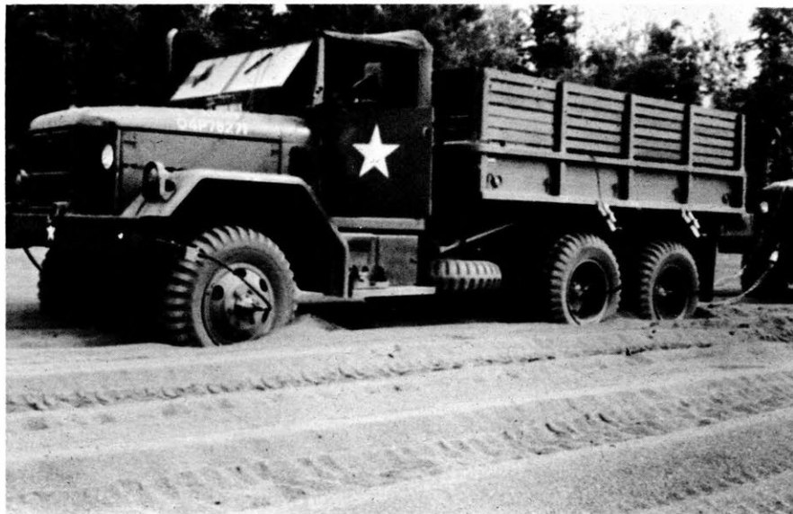
Figure 10. Wheel sinkage, 15-psi tires.
