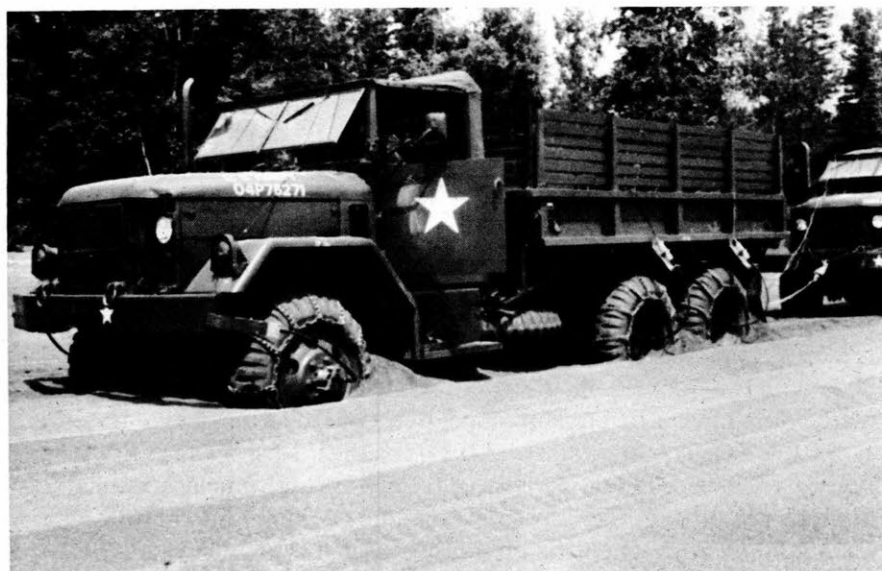
Figure 11. Wheel sinkage, tires with chains.
