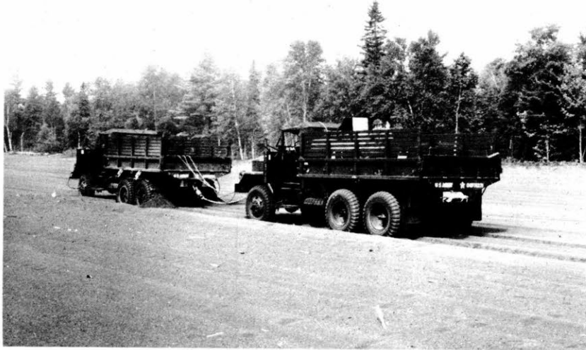
Figure 6. Stamp sand test course, load: instrument-carrying vehicle.
