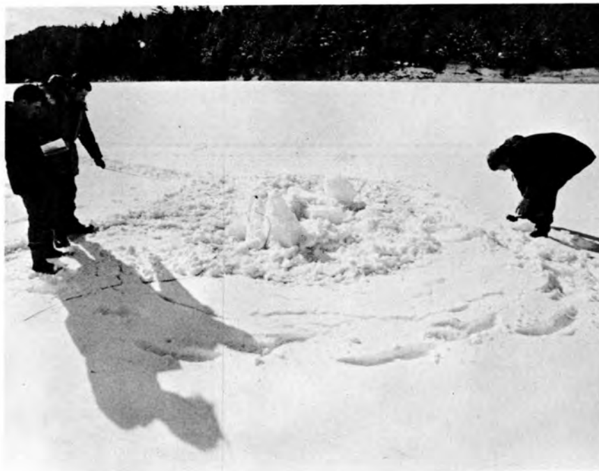
Figure 21. N.H. explosive tests. Discharge and breakage pattern for charge no. 2.
