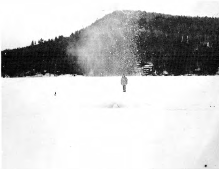
Figure 14 (Cont'd). Second N.H. test series. Discharge sequence and pattern of ice breakage for Cardox shell no. 1.
