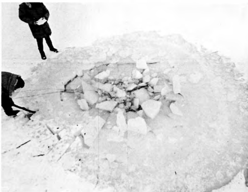
Figure 15. Second N.H. test series. Discharge sequence and pattern of ice breakage for Cardox shell no. 2.
