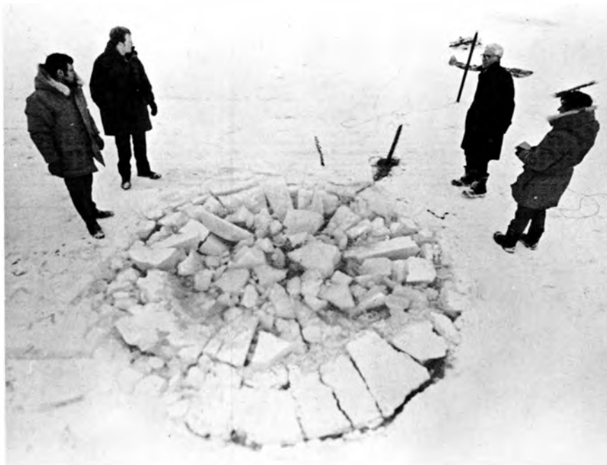
Figure 18 (Cont'd). Second N.H. test series. Discharge sequence and ice breakage pattern for Cardox shell no. 6.
