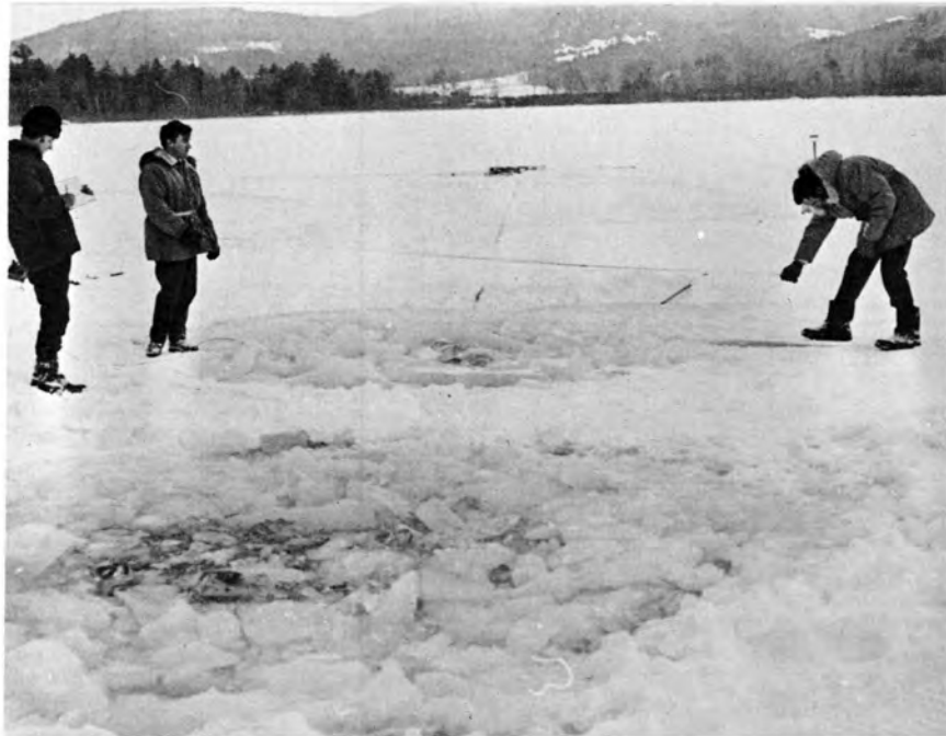
Figure 9. First N.H. test series. Craters, or breakage areas, for Cardox shells no. 1 (foreground) and no. 2 (center).
