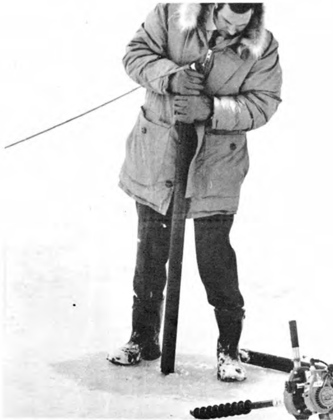
Figure 6. First N:H. test series. Cardox shell being placed for Shot #1.
