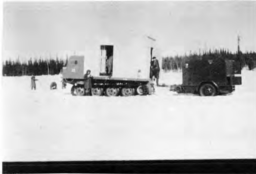
Figure 4. Alaska test site. The six-stage airblast compressor is mounted on a tracked vehicle, and a cabin has been built around it for shelter. The vehicle is towing an electrical generator.
