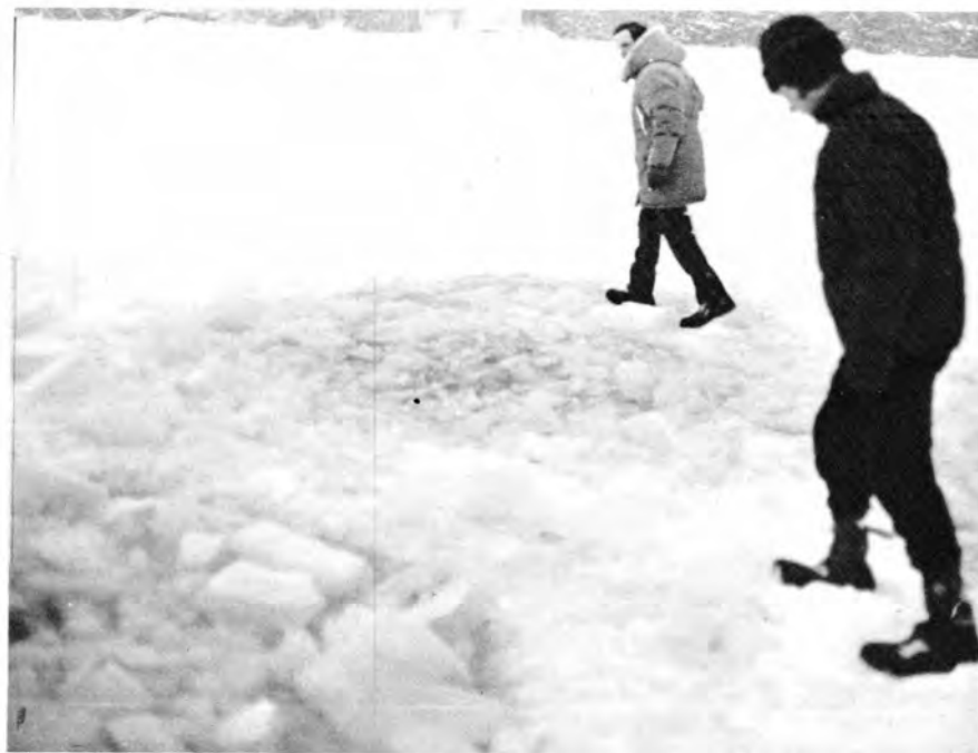
Figure 13. First N.H. test series. Discharge for Cardox shell no. 5. (a) Connecting firing line to Cardox shell no. 6. (b) Ice broken by shell no. 6.
