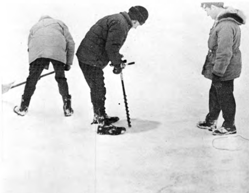
Figure 10. First N.H. test series. Installation of shell and discharge sequence for Cardox shot no. 3.
