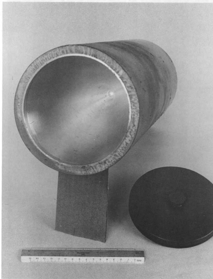
Figure 32. Cases and liners for experimental binary shaped charges. The smaller charge has a 60^\circ copper cone with a 5-in. mouth diameter. The larger charge has a 45^\circ/30^\circ biconic copper liner with a 5.75-in. mouth diameter.
