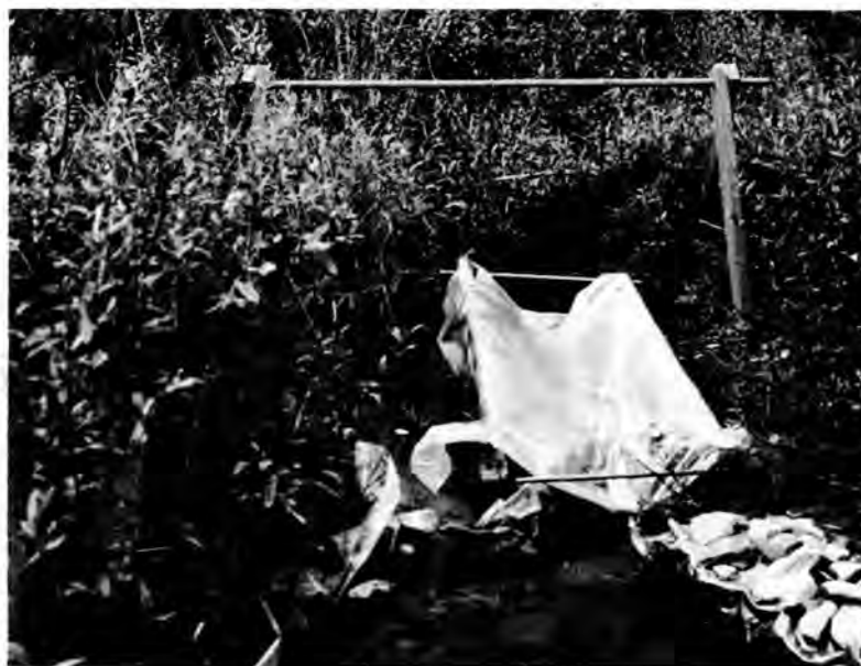
Figure 5. Flume used in volumetric discharge determinations.
