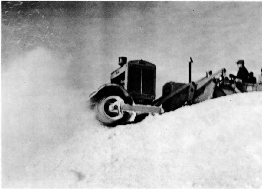
Figure 5. Ice chipper working on top of pressure ridge. Notice that ice chipper is in a raised position.
