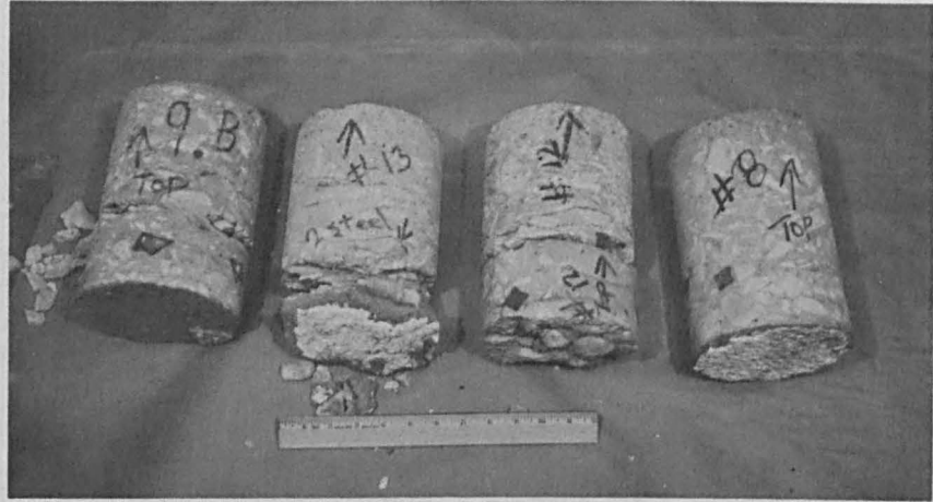
a. South span (cores 8, 9, 12, and 13)
