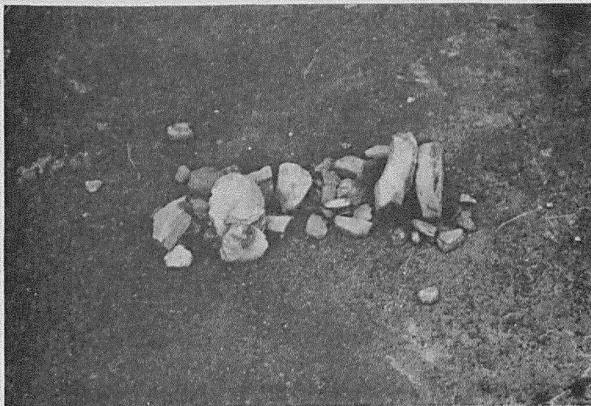
b. Backfill Recovered with 6-in.-Diameter Core Barrel
