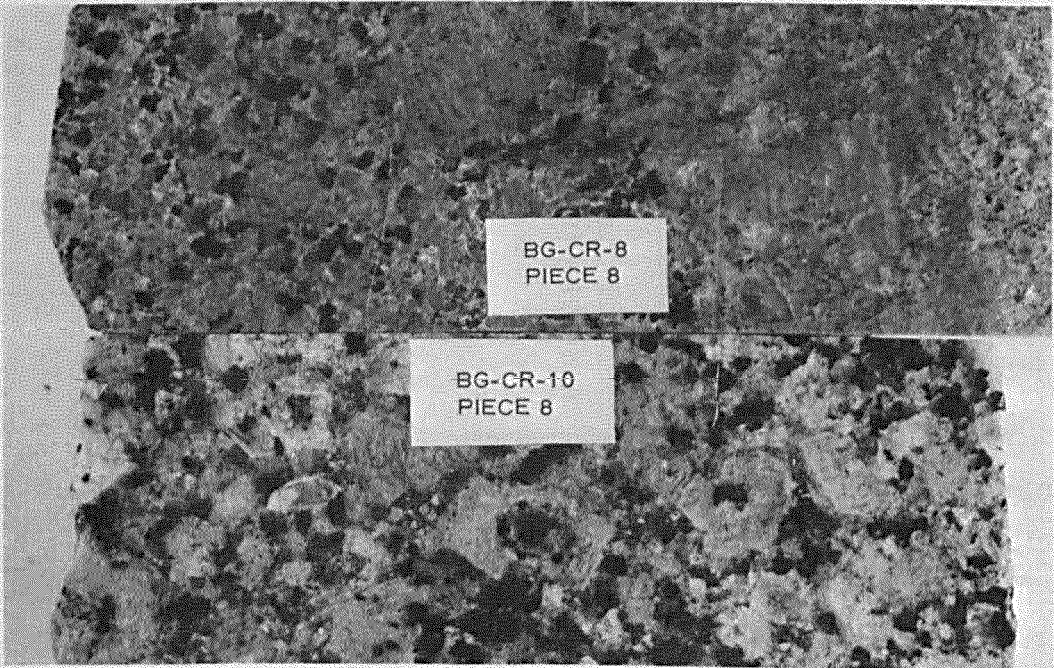
Figure 4.1 Core BG-CR-8, Piece 8, and Core BG-CR-10, Piece 8. Magnification, \times 1 . Portion on left side of Piece 8, Core 8, is typical reddish granitic rock; that on right side is reddish pegmatite. Piece 8, Core 10, is typical pinkish granitic rock. The large phenocryst below the label shows a mantle of pink microcline around a core of plagioclase feldspar, biotite, and quartz (antirapakivi texture).
