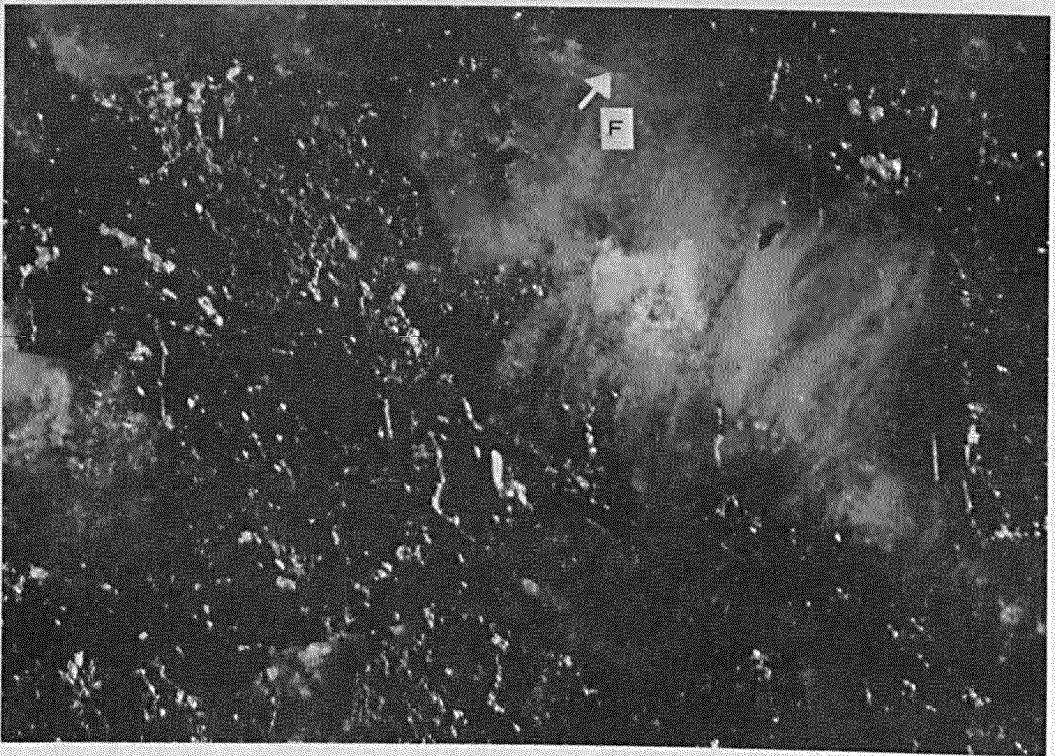
Figure 4.7 Typical portion of Core 19, Piece 14, at \times 20 magnification. There is only one perceptible crack; it is in plagioclase feldspar and is indicated by an arrow.
