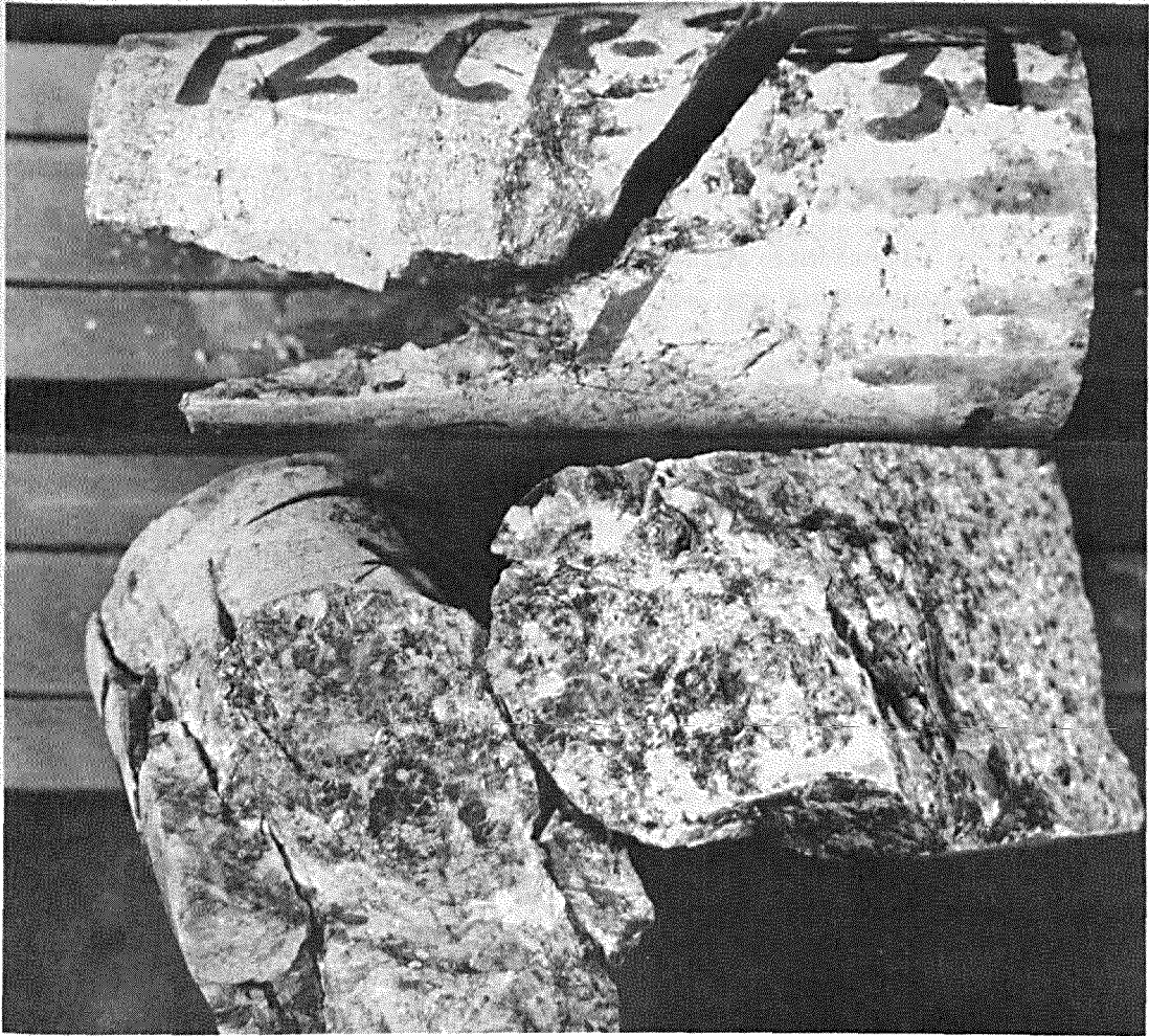
Figure 3.2 Core PZ-CR-23, Specimen 7. The top half of the photograph shows the planes along which the section failed during compressive tests. The lower half shows a mica layer inclined at about 40 degrees along which failure occurred.
