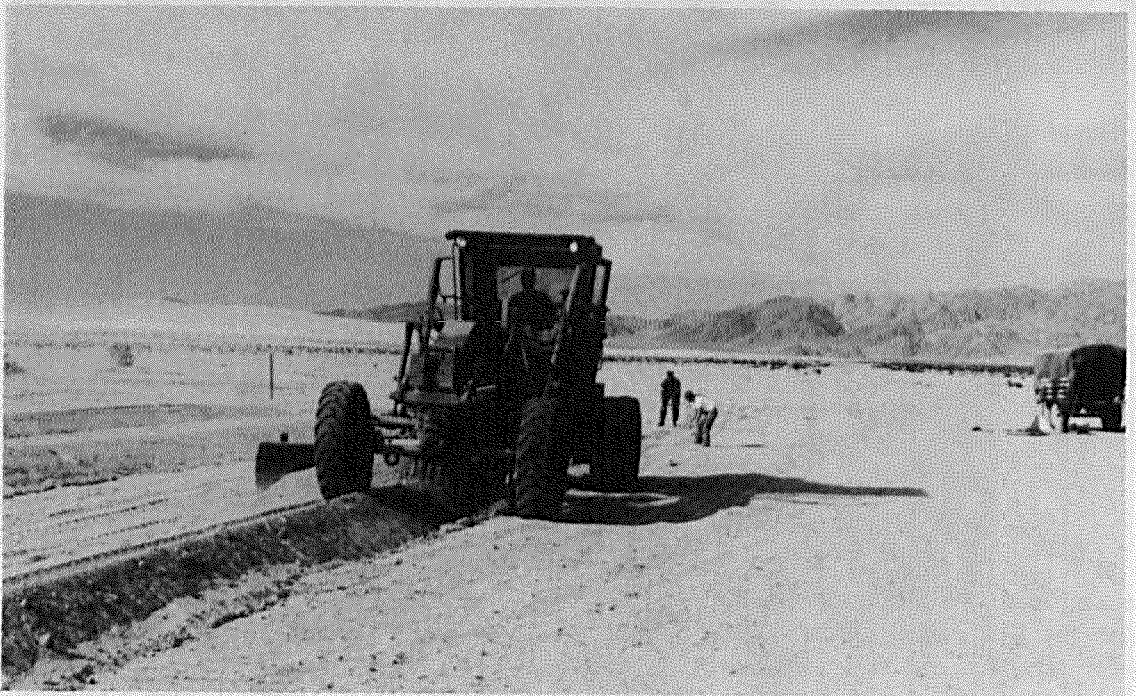
Figure 7. Grader burying mines.
