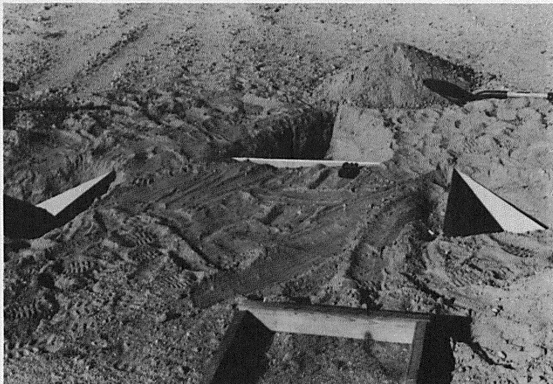
Figure 16. Buried corner reflectors with sieve.
