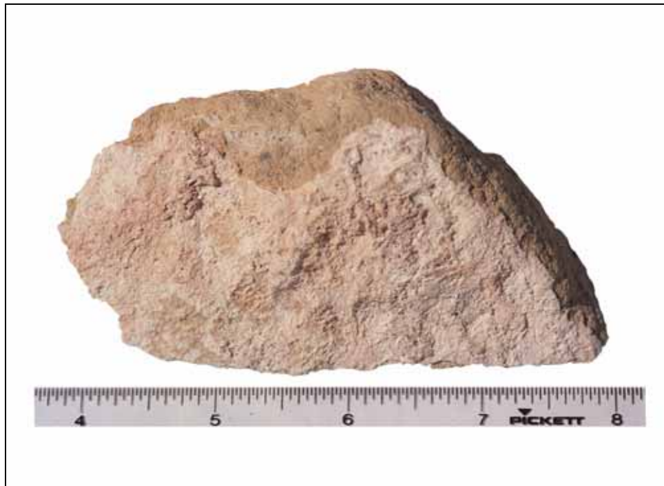
Figure 16. Carbonate deposit (white) and weathering rind (yellow-green) on basalt clast sample from Figure 14.
