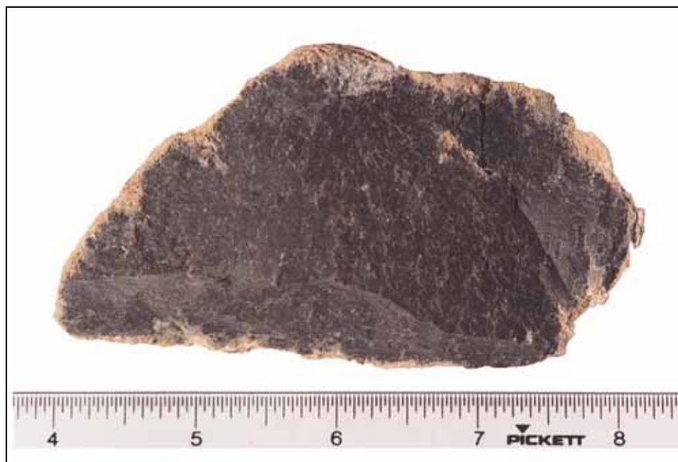
Figure 14. Basalt cobble (black) and external weathering rind (yellow-green).
