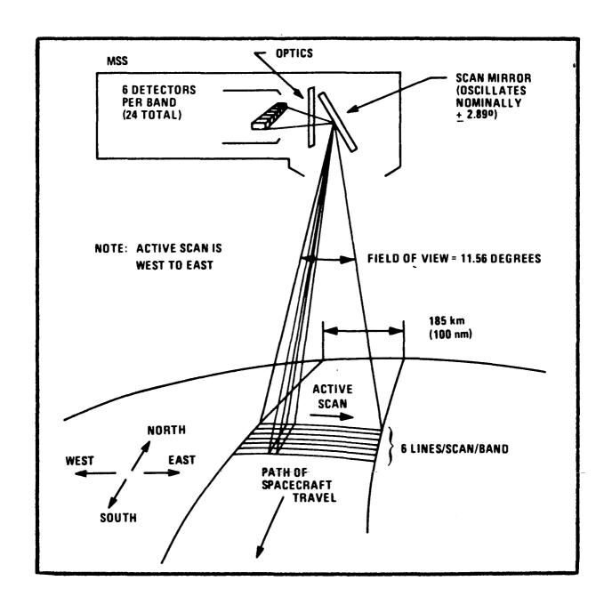
Figure 2. Schematic of Multispectral Scanner Subsystem
