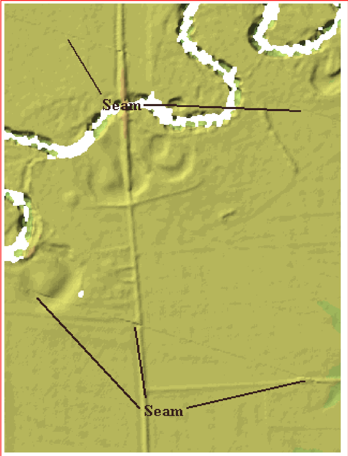
Figure 46. Third LIDAR Delivery Seaming Anomaly
