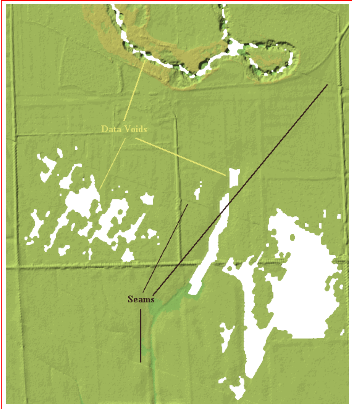
Figure 37. Data Voids in Second LIDAR Delivery and Seam Anomaly
