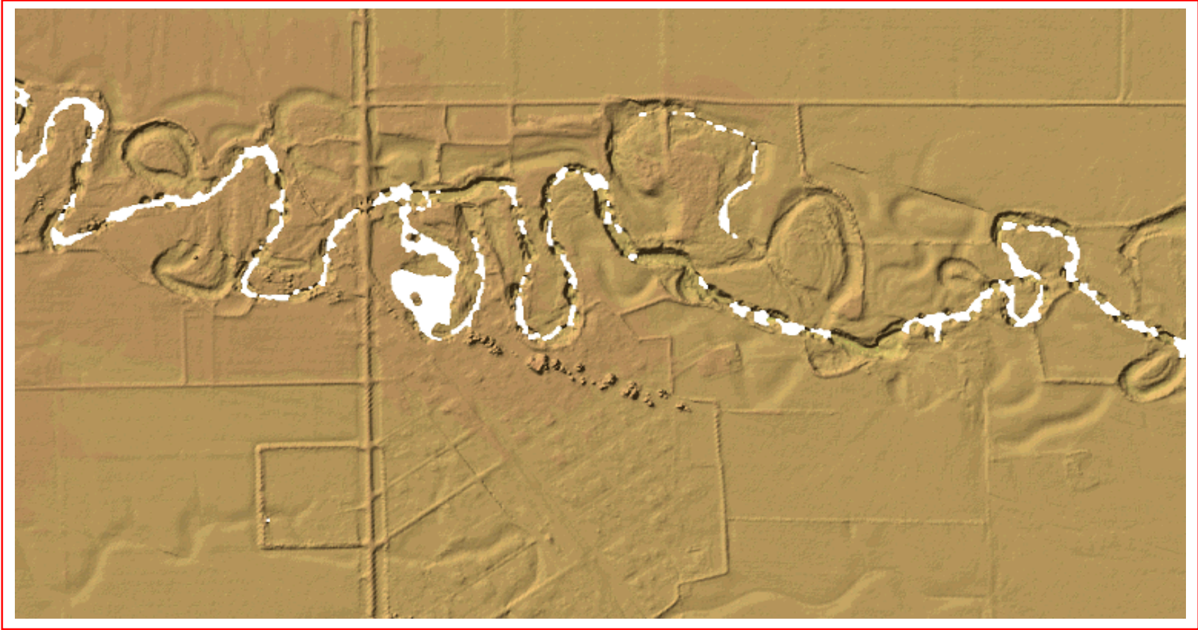
Figure 38. Data Voids in Second LIDAR Delivery
