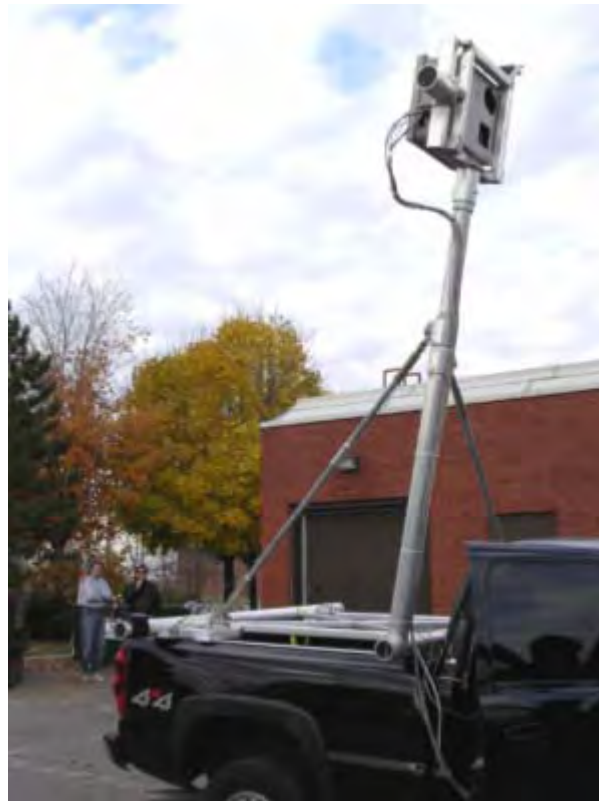
Figure A1. SideSwipe truck mounted LIDAR system.
