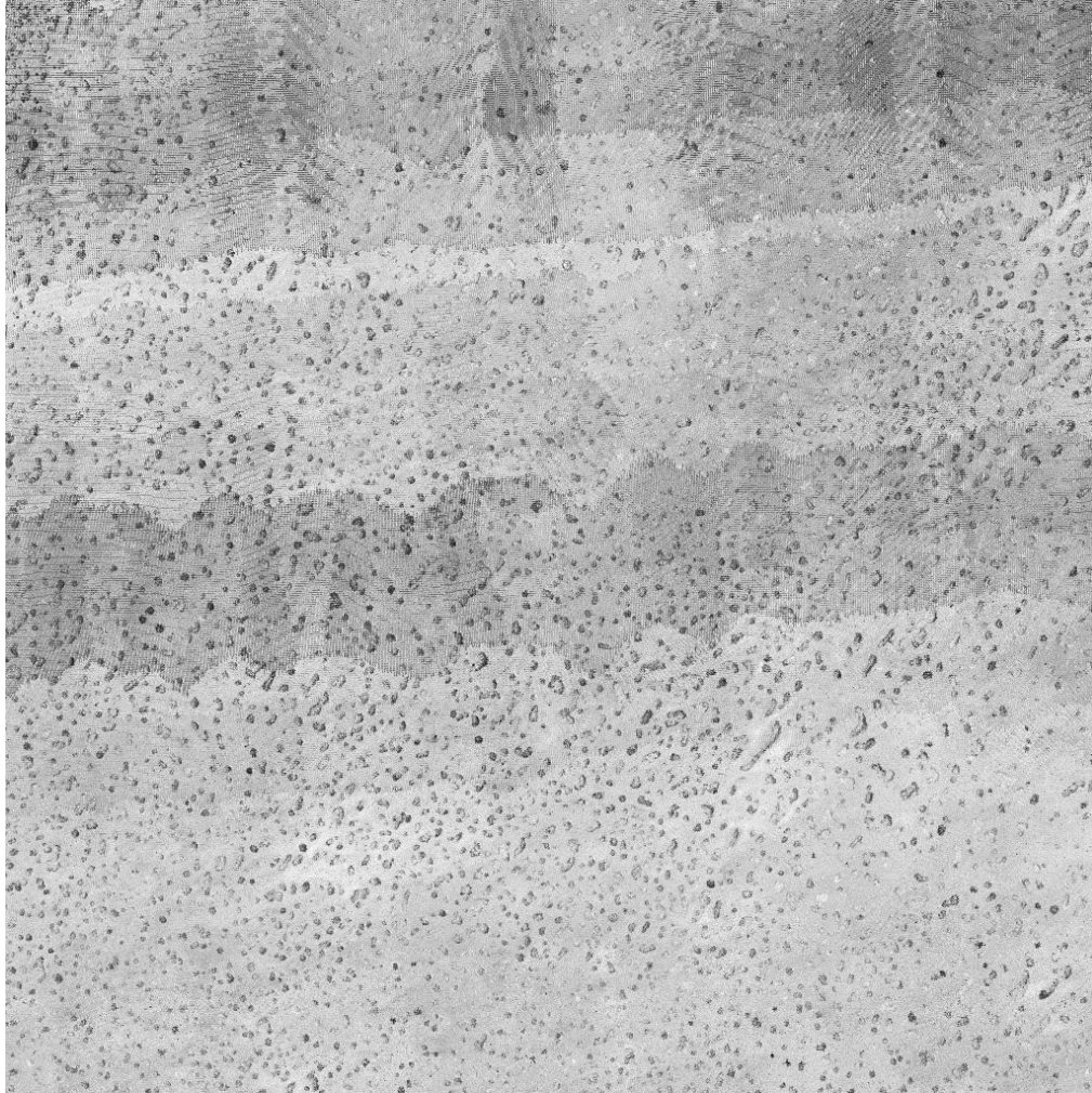
Figure 85. An example of poor calibration of intensity returns between different flight lines that affects data about vegetation reflectivity (1-m resolution data for tile 381_3577).
