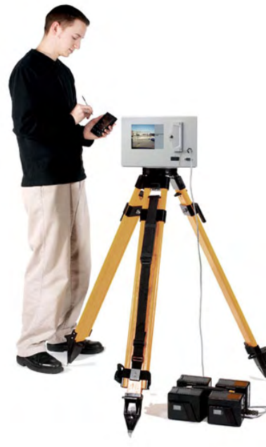
Figure A3. General view of portable ILRIS-3D.
