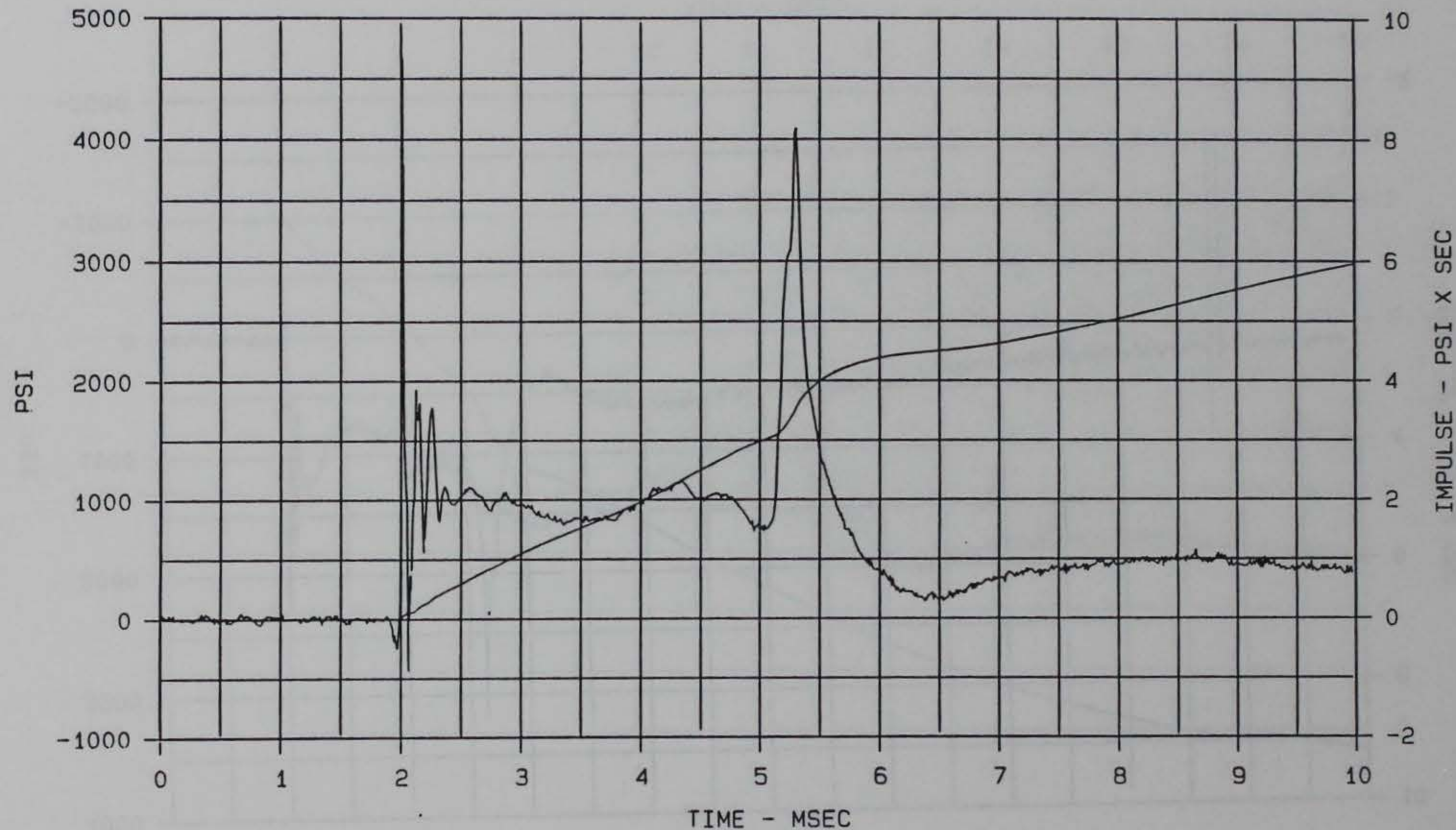
Figure 90. Soil stress wave form measured by gage SEV-3, 10 msec duration, MCBI Gage Validation Test 2
