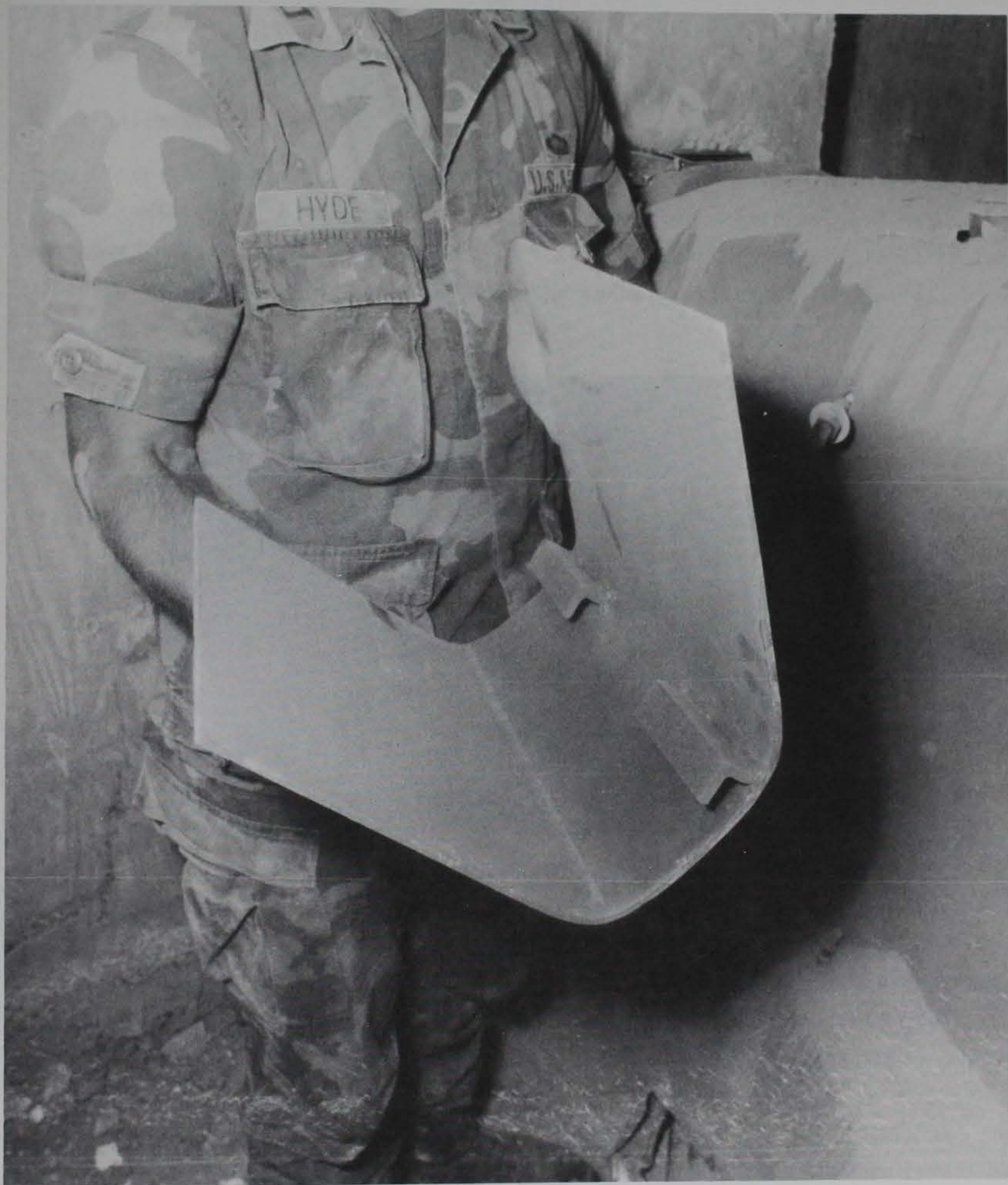
Figure 4.6. Damage to commercial door support plate.
