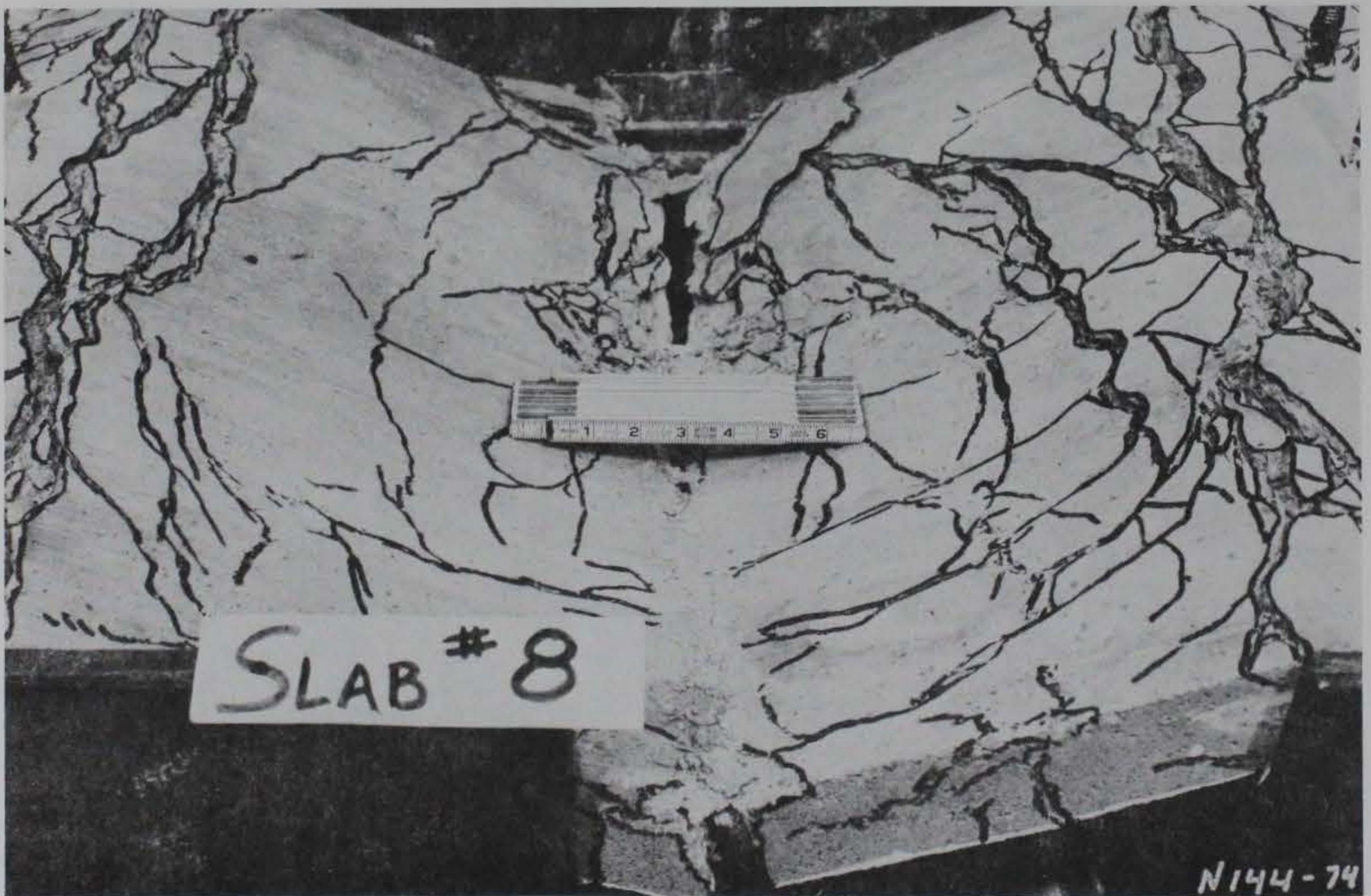
Figure 4.19. Closeup view of Slab 8, posttest.
